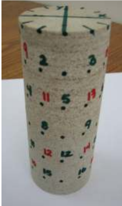
Figure 3.6: Sensor Locations on Berea Sandstone Sample
