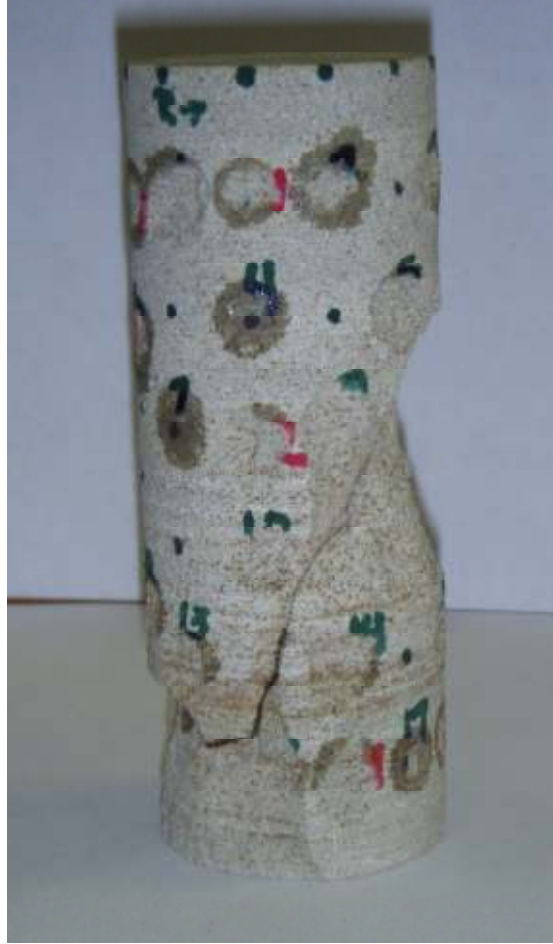
Picture of Failed Sample from Experiment #4
