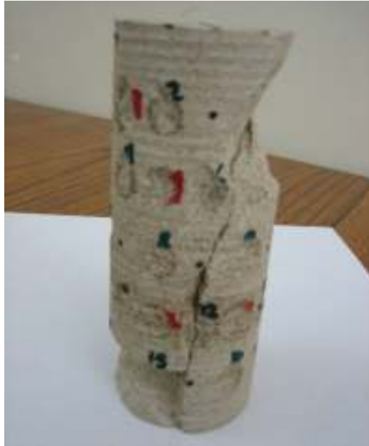
Figure 3.9: Failed Berea Sandstone Sample
