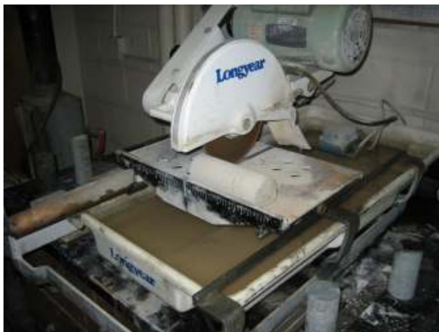
Figure 3.3: Tile Saw used for Sample Length Reduction
