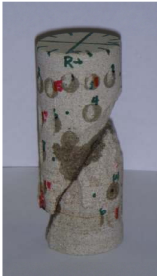
Figure 5.20: Failed Berea Sandstone Sample from Experiment #2
