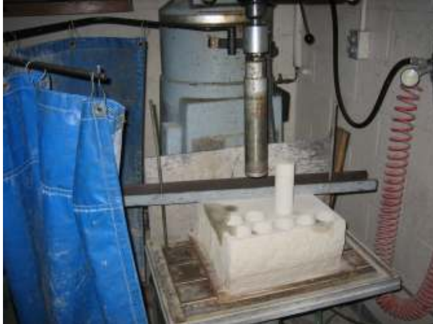
Figure 3.2: Modified Milling Machine for Coring Rock Samples
