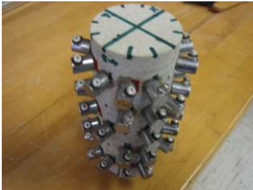
Figure 3.7: Sensors Attached to a Berea Sandstone Sample
