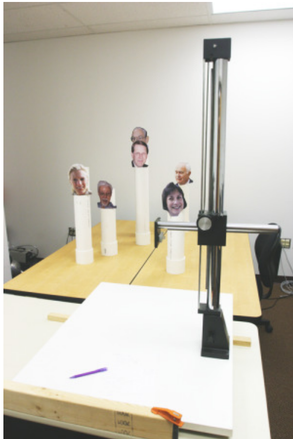
Figure 1.3: Our setup for gathering data includes the copy stand in the foreground and PVC pipes with photos of faces taped on top.
