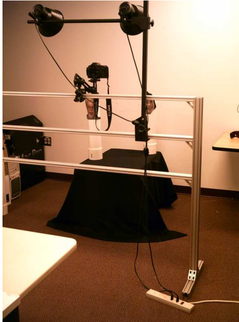
Figure 1.2: The aluminum stand I built to take the pictures for the camera array
