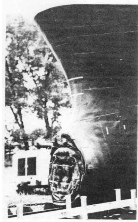
Figure 4.2 – Scale Model of a Bulbous Bow After Collision [43]
