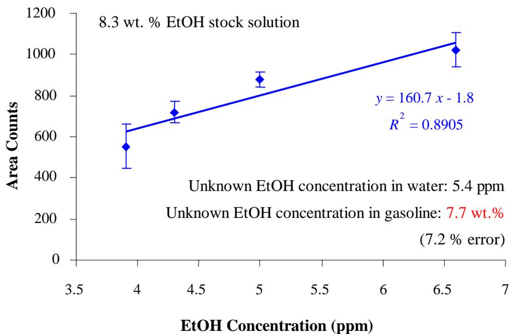
Fig. 4.13: Calibration curve using result set #1
