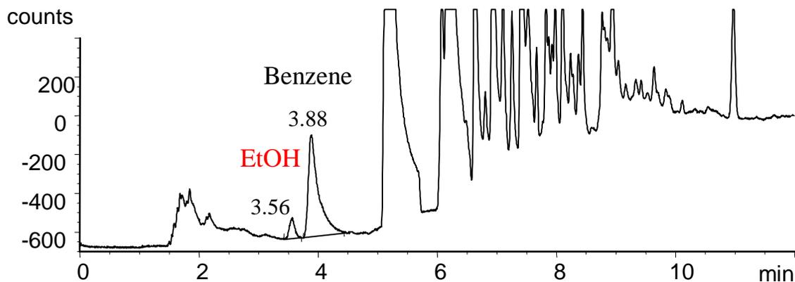
**Fig. 4.7: SPME-GC of 4.3 ppm EtOH in the water extracted gasoline fraction**
