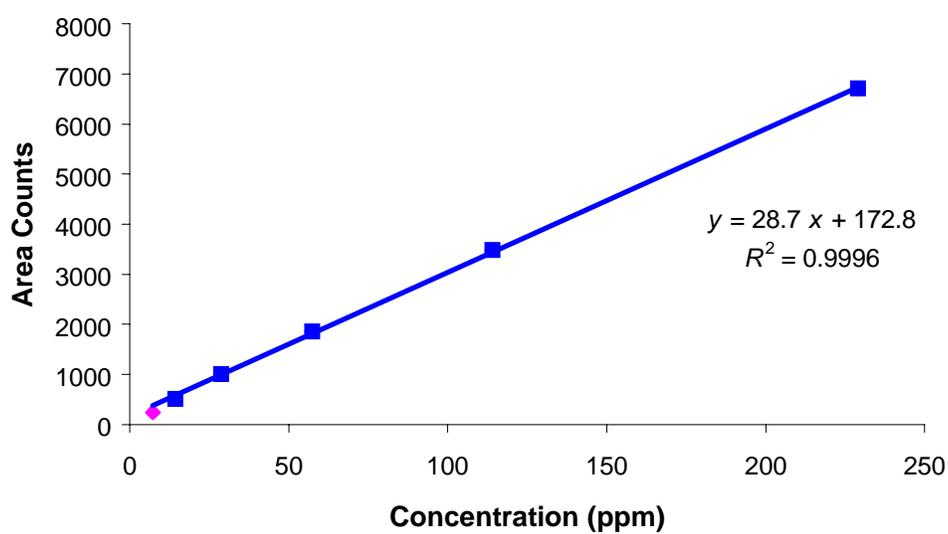
**Fig. 4.1: Linearity curve for methanol (F.I.D)**
