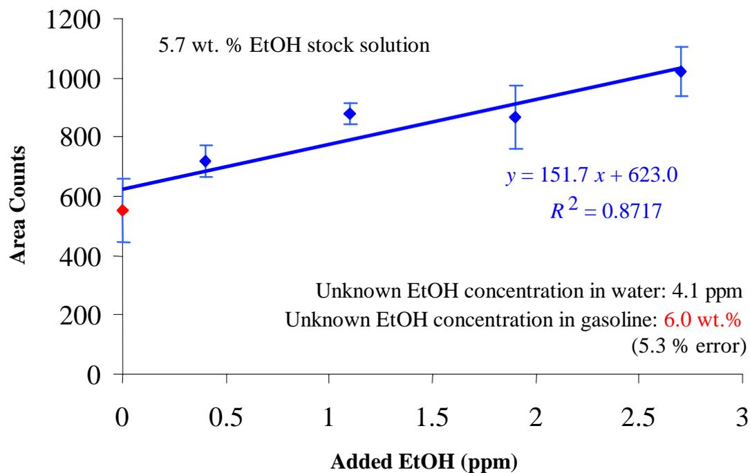
**Fig. 4.10: Standard addition curve using result set #1**
