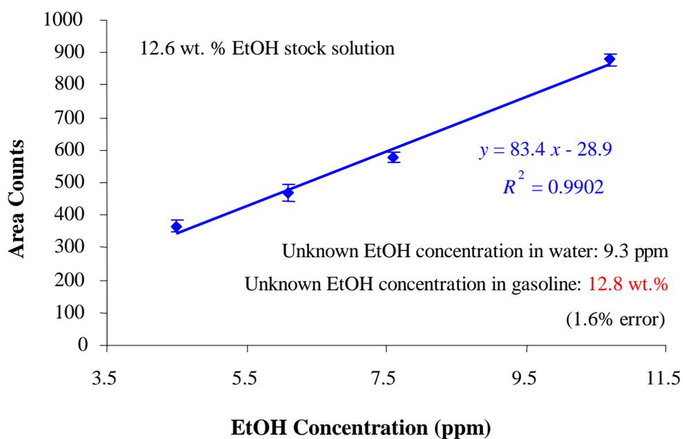
**Fig. 4.14: Calibration curve using result set #2**
