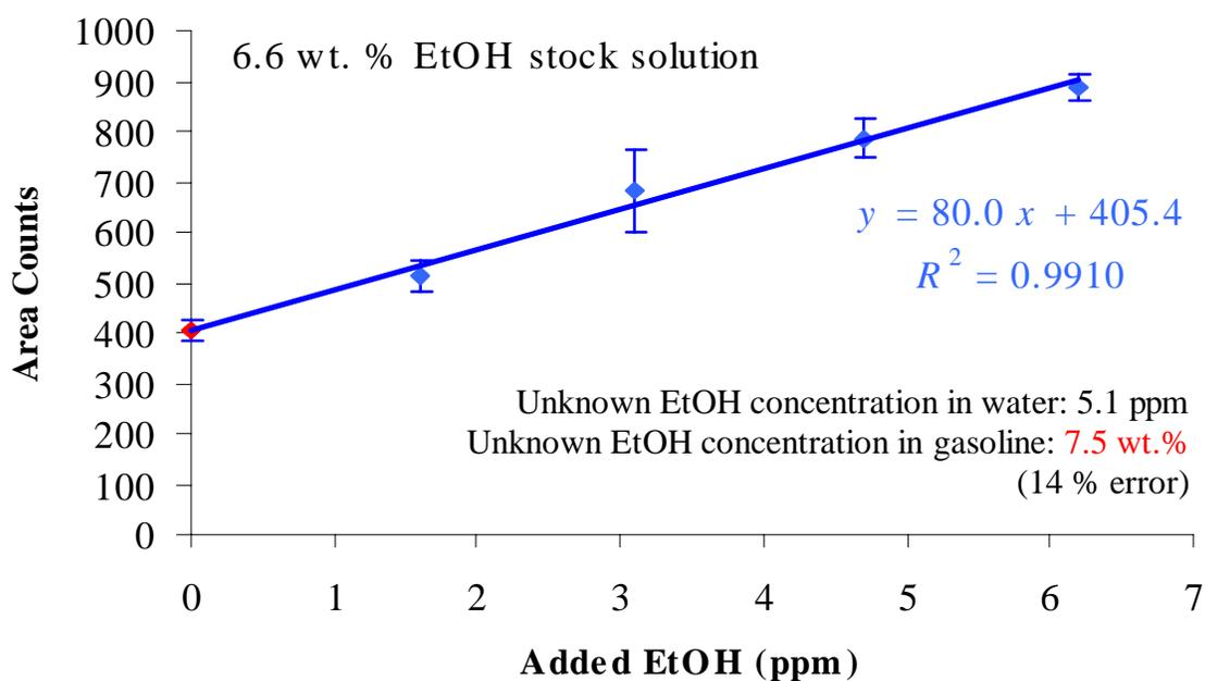
**Fig. 4.12: Standard addition curve using result set #3**
