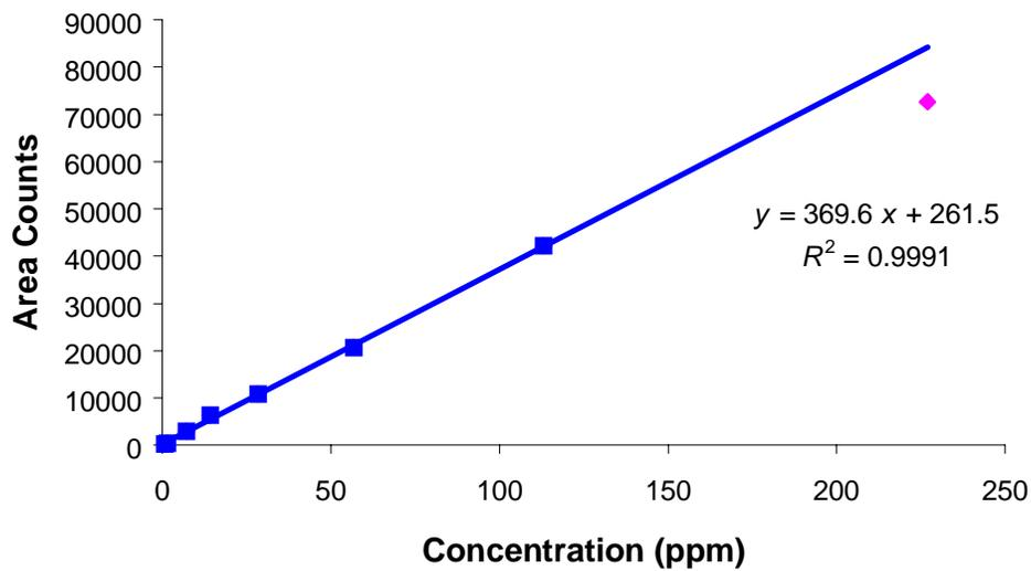
**Fig. 4.2: Linearity curve for ethanol (F.I.D)**
