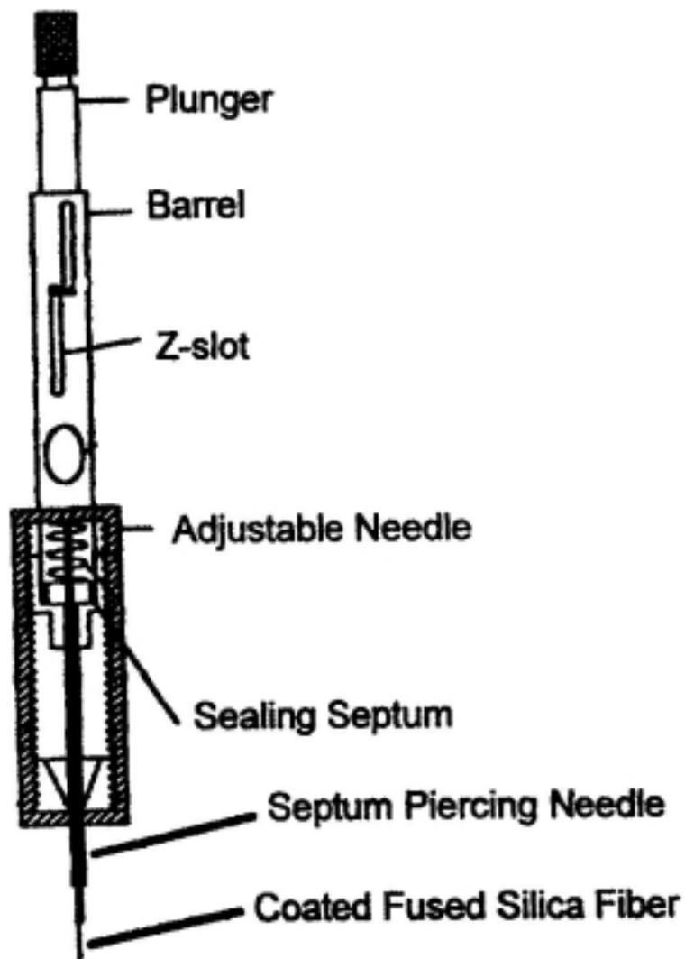
**Fig. 2.3: Scheme of SPME assembly**
