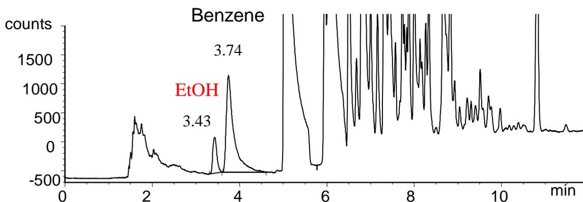
**Fig. 4.6: SPME-GC of 39 ppm EtOH in the water extracted gasoline fraction**
