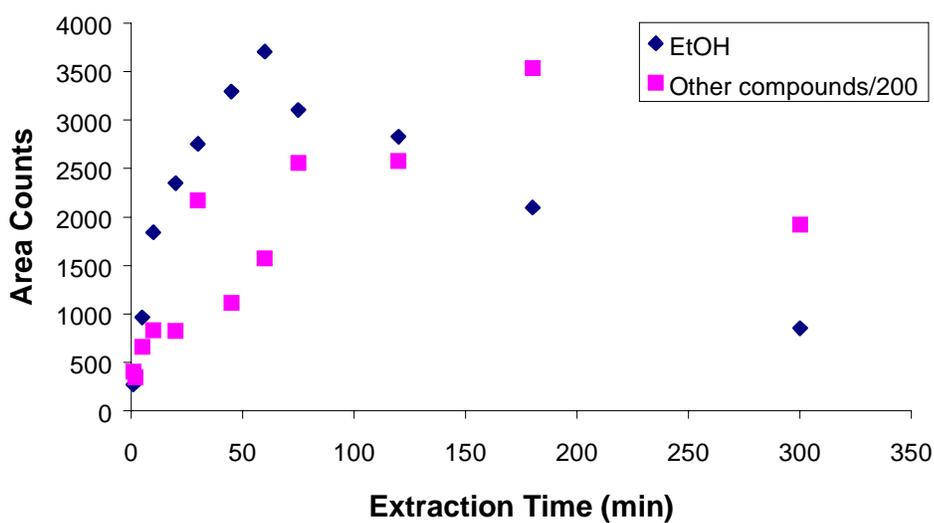
**Fig. 4.9: Headspace sampling extraction time curve**
