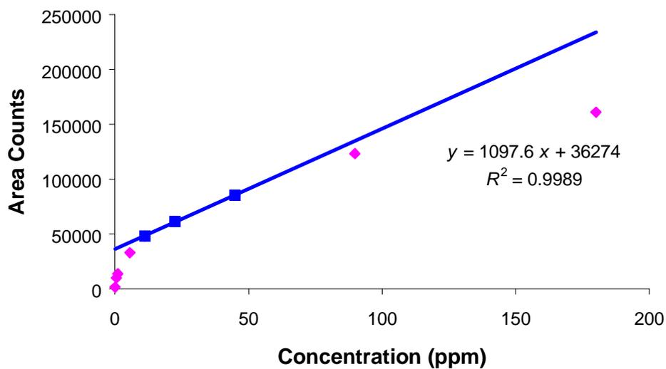
**Fig. 4.3: Linearity curve for methyl-tert-butyl-ether (F.I.D)**
