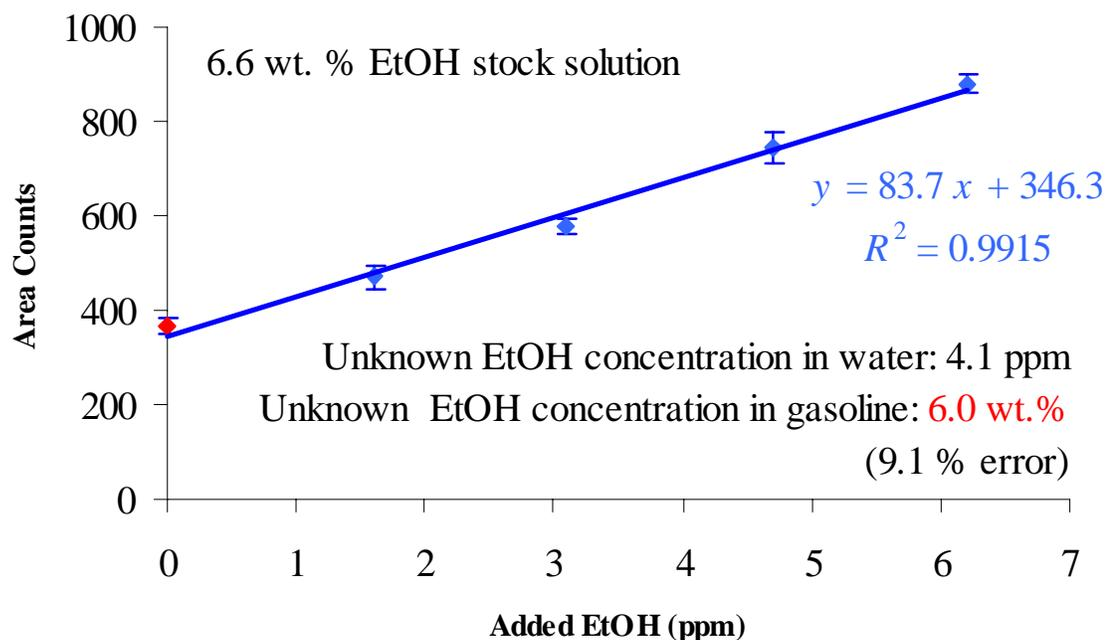
**Fig. 4.11: Standard addition curve using result set #2**
