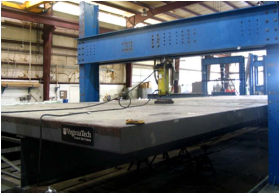
Figure 5.4: Test setup for finite element panel validation
