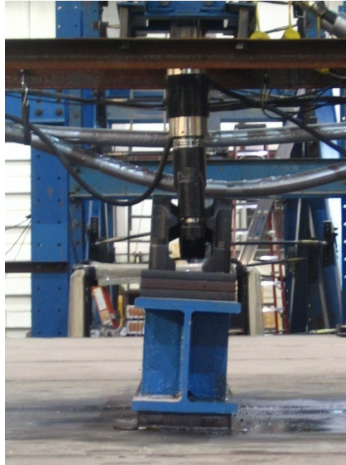
Figure 4.16: Spreader beam and bearing pad under maximum load after weld cracking
