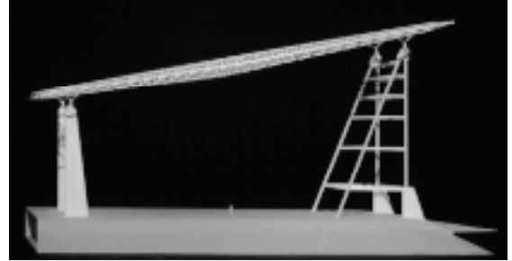
Structure Model. The roof structure spans the exhibition hall in 64.5m (215').
