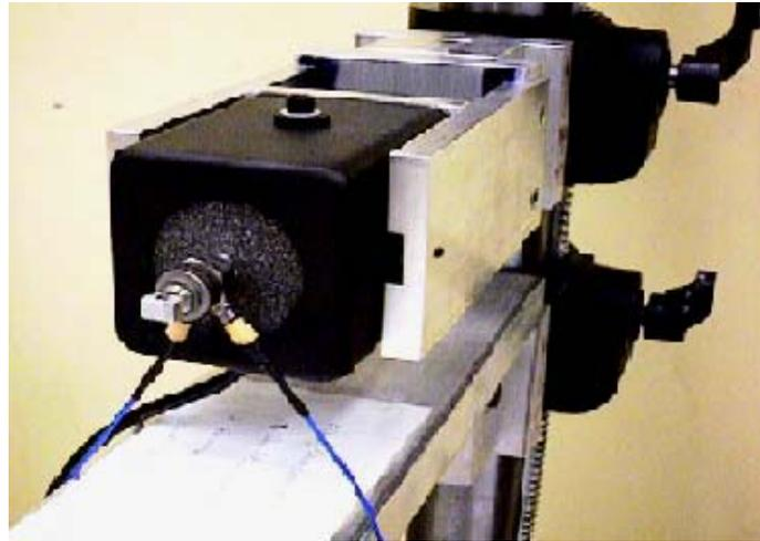
**Figure 3. MRTA device: shaker, probe, sensor, and platform.**
