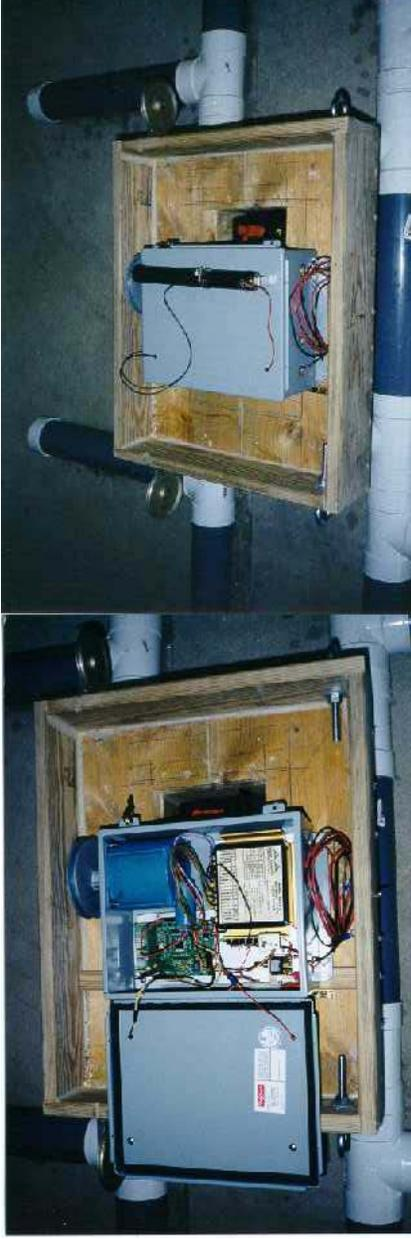
**Figure 5: Control box showing stepping motor and controller**
