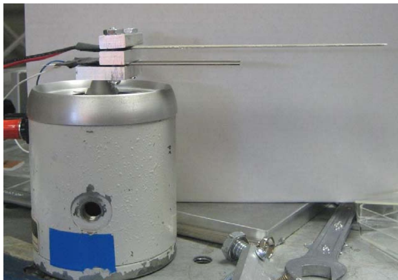
Figure 3.3.5. Photograph of test mount for AFC and PS monolithic bimorphs.
