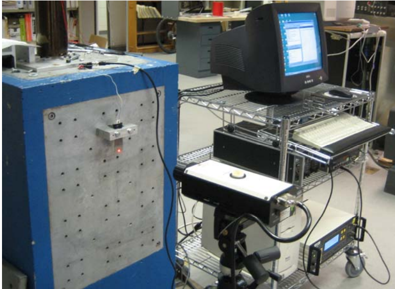
Figure 3.2.4. Photograph of test setup for Piezo Systems bimorph experiments.
