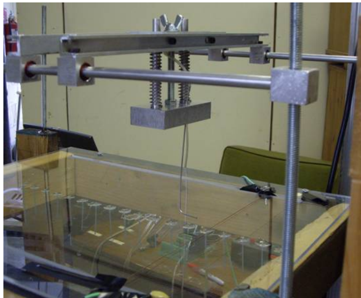
Figure 2.3.2 Picture of boundary layer positioning apparatus mounted above flat plate
