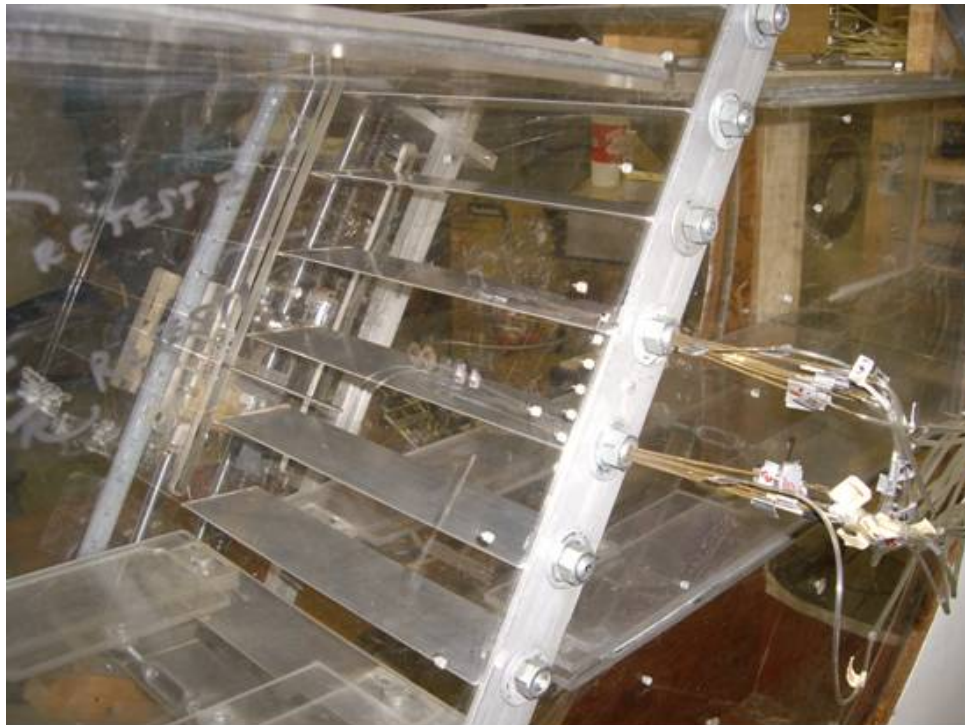
Figure 2.4.2 Linear blade row bolted to Plexiglas circles that make up the cascade test section; surface pressure measurement connections are shown
