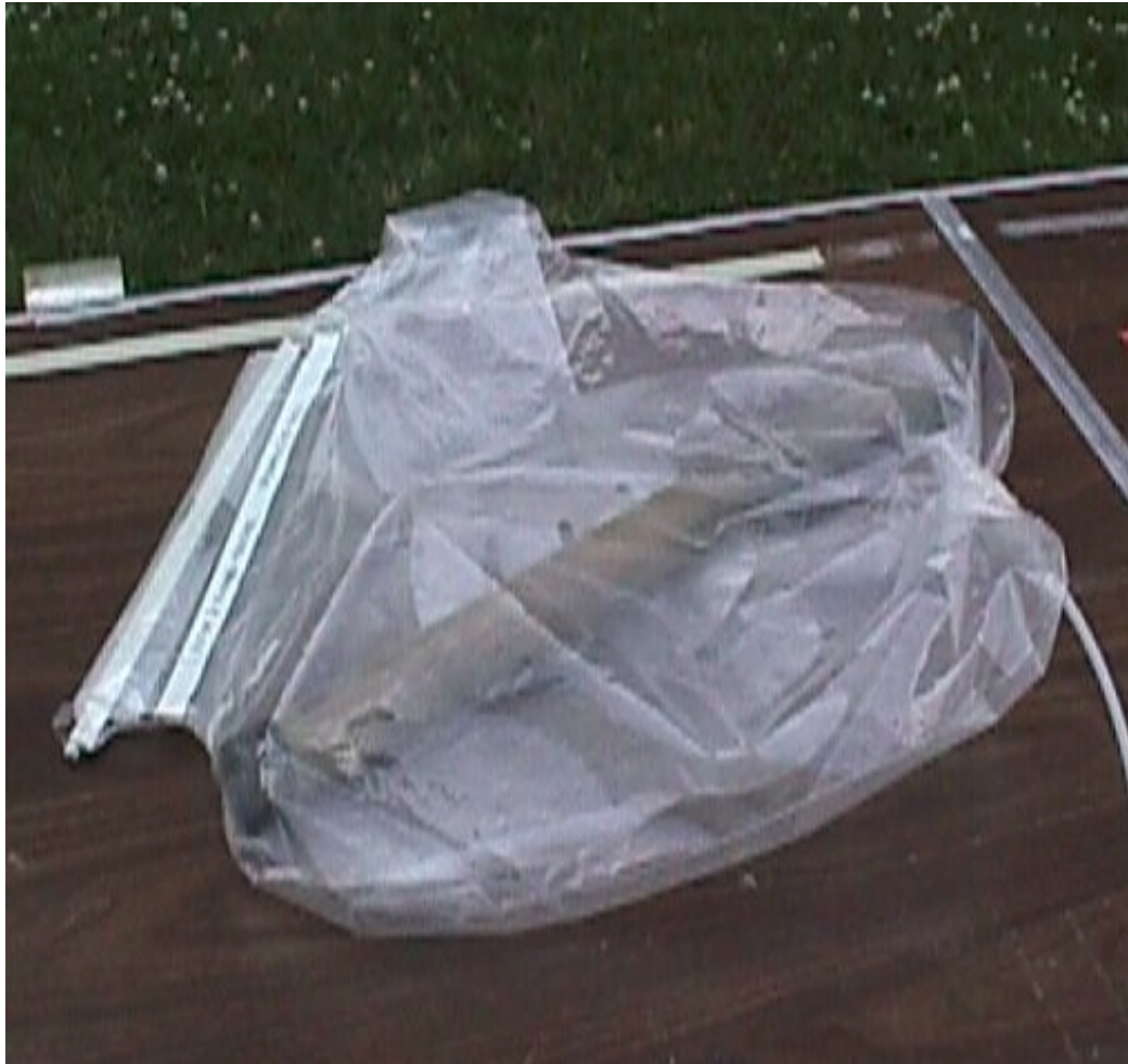
Photograph 3. Aquifer sediments placed in anaerobic glove bag and purged with nitrogen.
