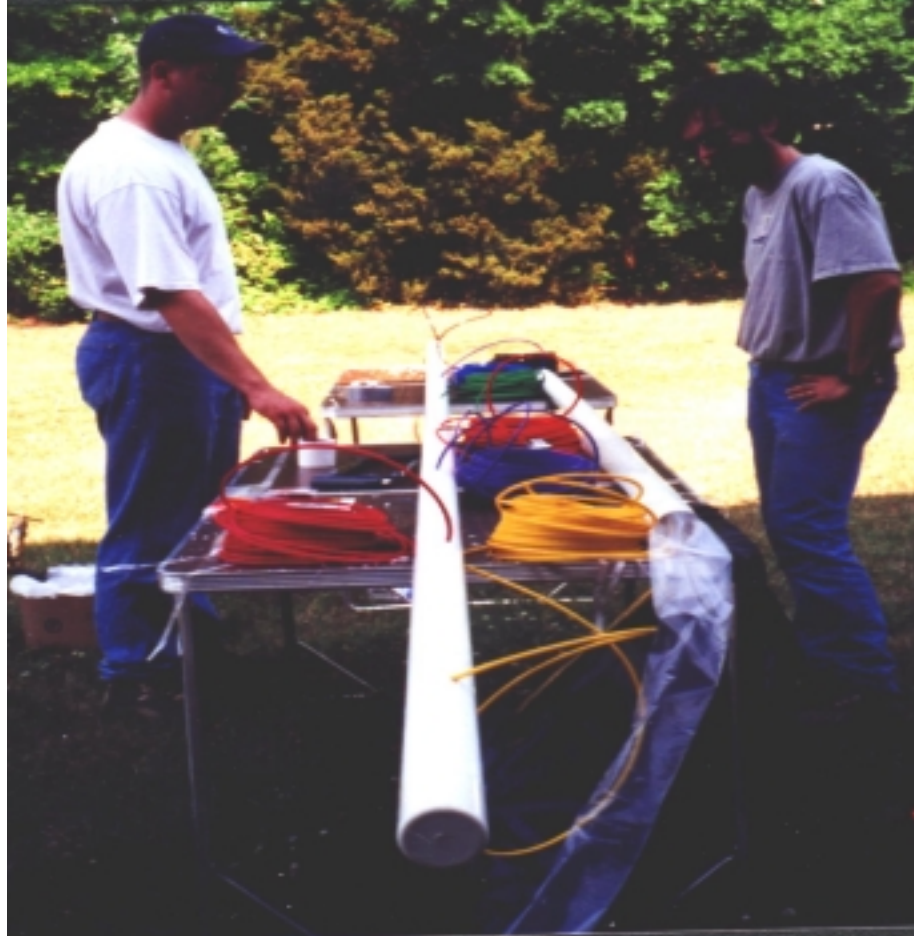
Photograph 4. Multi-level sampler well configuration. Colored tubing is used to distinguish sampling depths at the surface.
