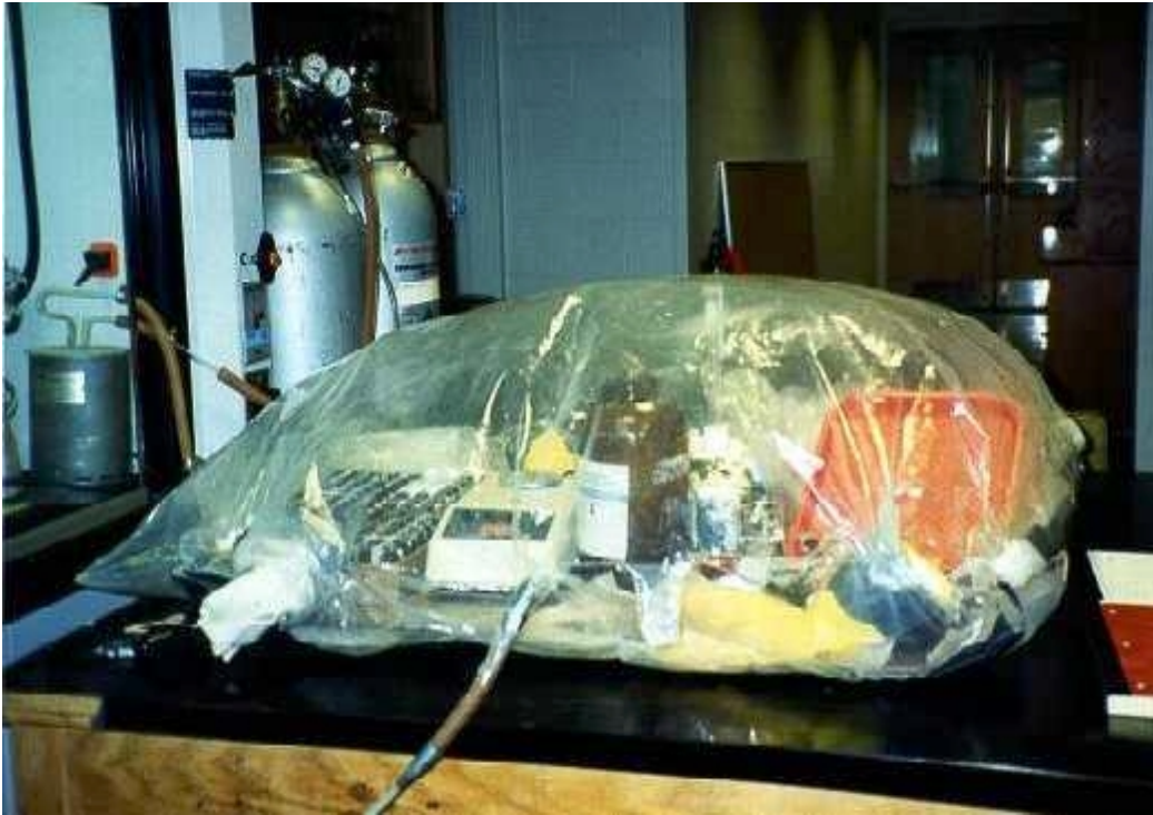
Photograph 6. Laboratory microcosms prepared in anaerobic glove bag.
