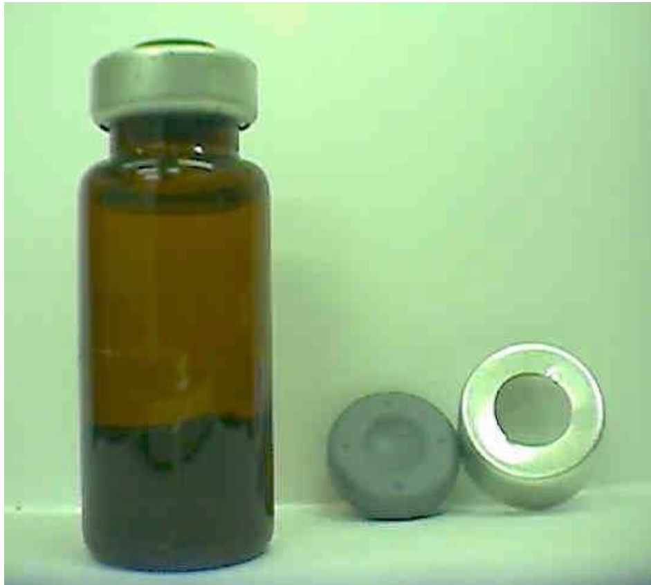
Photograph 7. Laboratory microcosm experiments conducted in 15-mL amber vials containing 7 grams (wet) aquifer sediment, 25 \mu M PCE and 10.5 mL aqueous solution. Teflon-lined rubber butyl septum and aluminum crimp cap used to seal microcosm.
