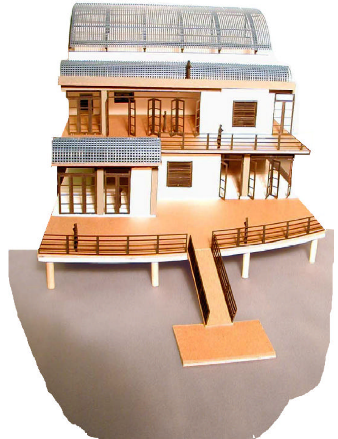
Sectional model (1/4" = 1') through pond, boat float, first and second floor decks, and atrium roof
