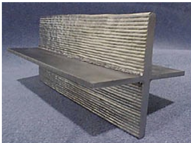
Figure 20: Machining preform (rib-on-web geometry) of a LAM Ti-6Al-4V part. From [69].
