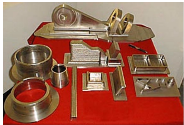
Figure 21: Machined LAM Ti-6Al-4V parts. From bottom left counter clockwise: cylindrical geometries, aircraft fitting, and angled walls. From [69].
