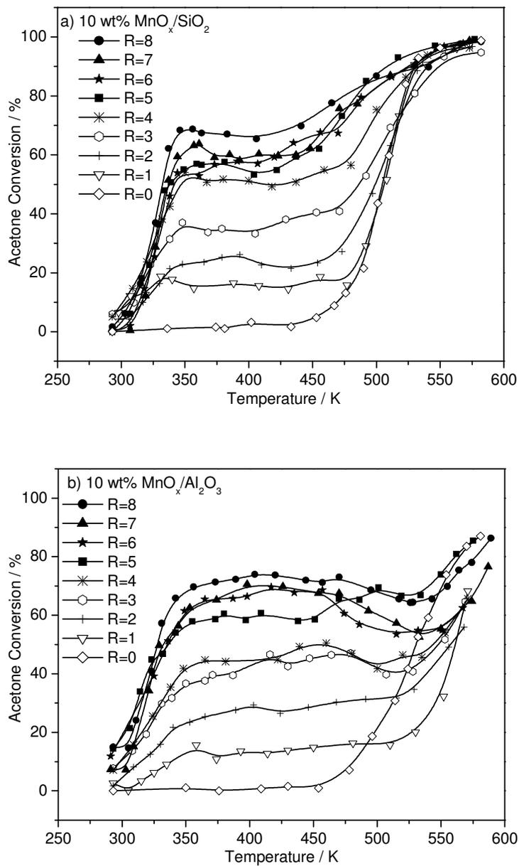
**Figure 2-8.** Acetone conversion versus temperature for 10 wt %  $\text{MnO}_x/\text{SiO}_2$  and 10 wt %  $\text{MnO}_x/\text{Al}_2\text{O}_3$  catalysts with various ozone concentrations: a) 10 wt %  $\text{MnO}_x/\text{SiO}_2$ ; b) 10 wt %  $\text{MnO}_x/\text{Al}_2\text{O}_3$ . R is the ozone/acetone molar ratio.  $F_{\text{tot}} = 3.1 \text{ L/min}$ ,  $S. V. = 15,000 \text{ h}^{-1}$ , acetone concentration = 1,000 ppm, ozone concentration = 1,000-8,000 ppm.
