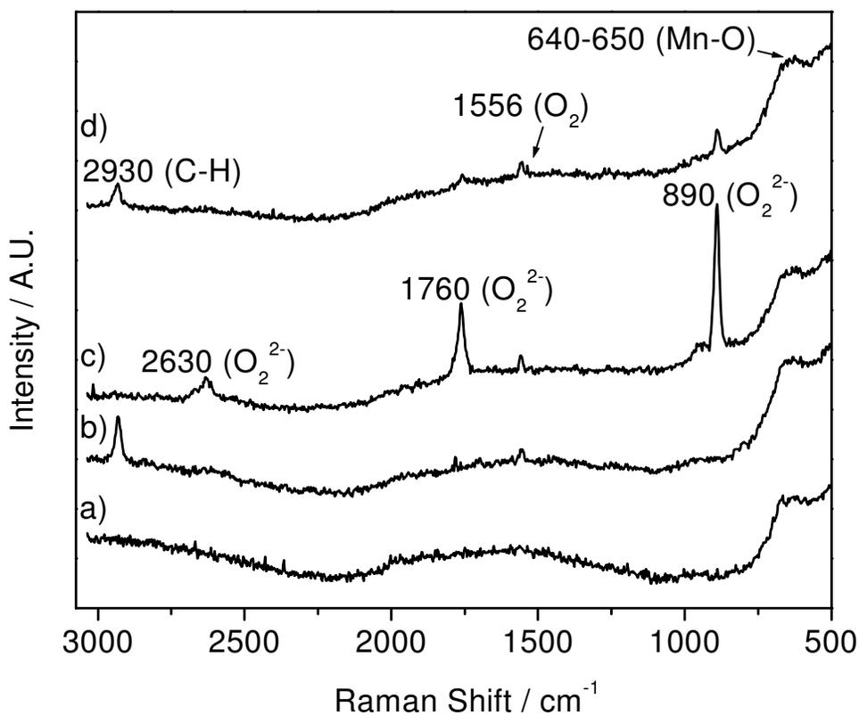
**Figure 2-10.** Raman spectra of the 10 wt %  $\text{MnO}_x/\text{SiO}_2\text{-H}$  exposed to different gas mixtures: a)  $\text{O}_2/\text{He}$ , b) acetone/ $\text{O}_2/\text{He}$ , c)  $\text{O}_3/\text{O}_2/\text{He}$ , and d) acetone/ $\text{O}_3/\text{O}_2/\text{He}$ .
