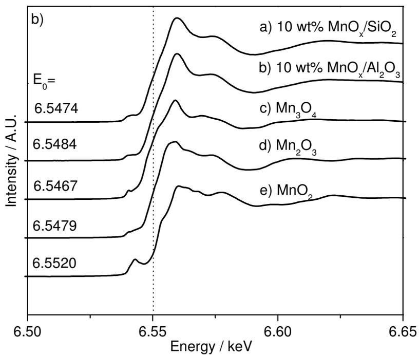
**Figure 2-4.** a) Fourier transforms of the Mn K-edge EXAFS spectra and b) Mn K-edge XANES spectra: a) 10 wt %  $\text{MnO}_x/\text{SiO}_2$ , b) 10 wt %  $\text{MnO}_x/\text{Al}_2\text{O}_3$ , c)  $\text{Mn}_3\text{O}_4$ , d)  $\text{Mn}_2\text{O}_3$ , and e)  $\text{MnO}_2$ .
