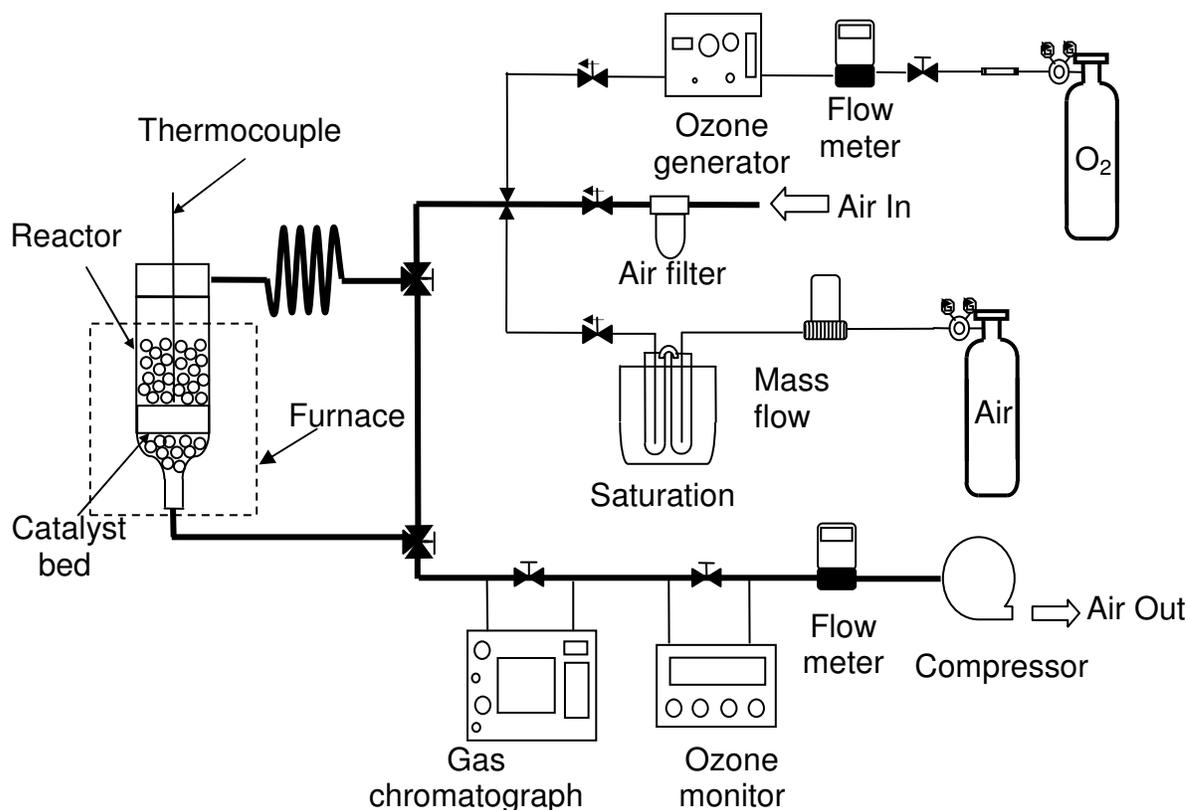
**Figure 2-1.** Schematic for acetone oxidation reaction system.
