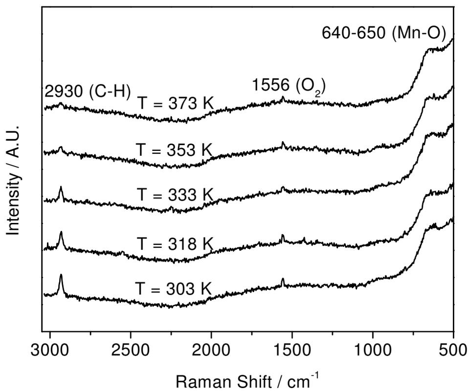
**Figure 2-11.** Effect of temperature on the 10 wt % MnO<sub>x</sub>/SiO<sub>2</sub>-H catalyst in acetone/O<sub>2</sub>/He.
