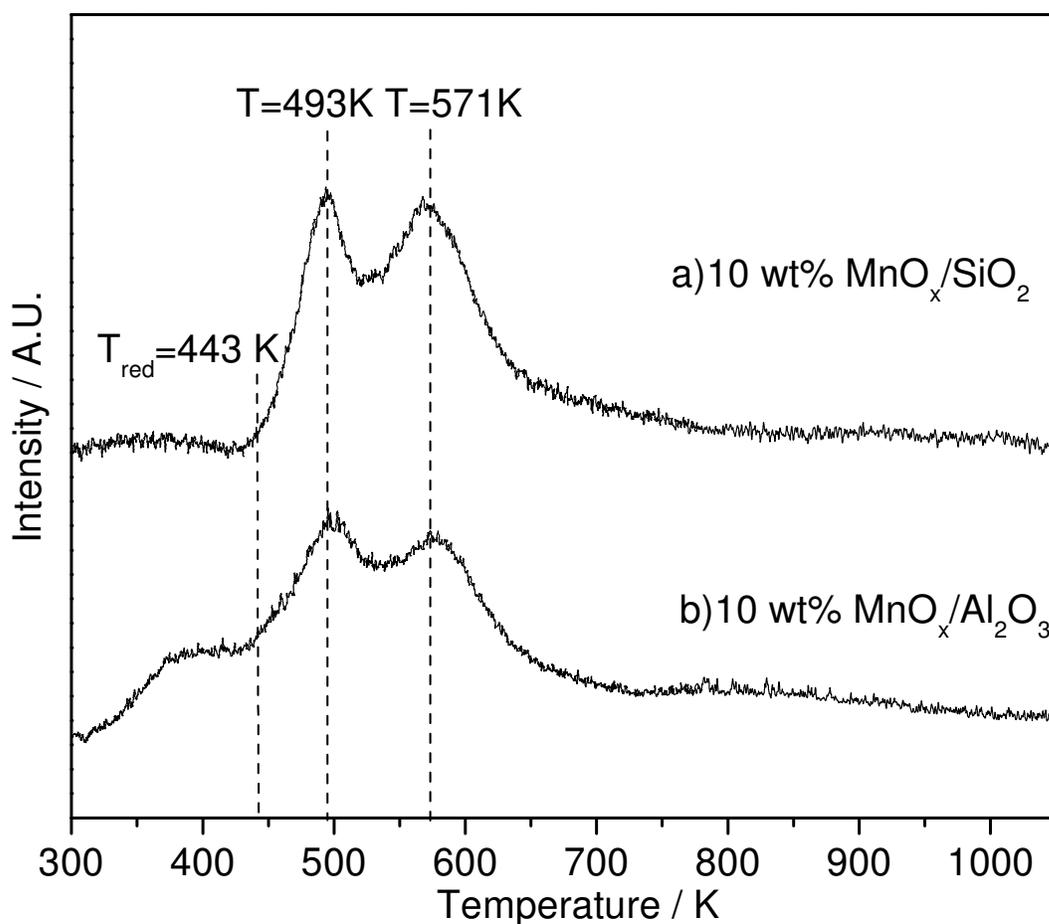
**Figure 2-5.** TPR traces ( $m/e = 18$ ) for a) 10 wt %  $\text{MnO}_x/\text{SiO}_2$  and b) 10 wt %  $\text{MnO}_x/\text{Al}_2\text{O}_3$ .
