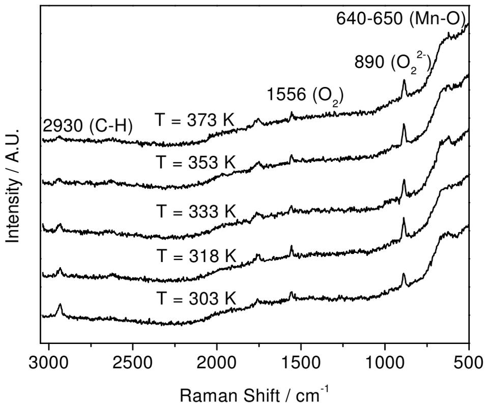
**Figure 2-12.** Effect of temperature on the 10 wt % MnO<sub>x</sub>/SiO<sub>2</sub>-H catalyst in acetone/O<sub>3</sub>/O<sub>2</sub>/He.
