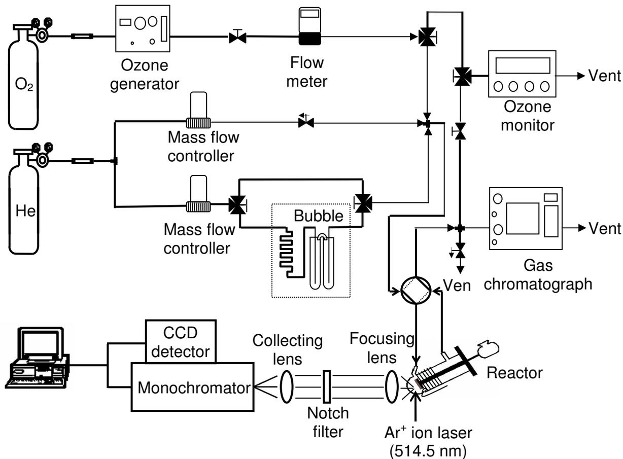
**Figure 2-2.** Schematic of *in situ* laser Raman spectroscopy system.
