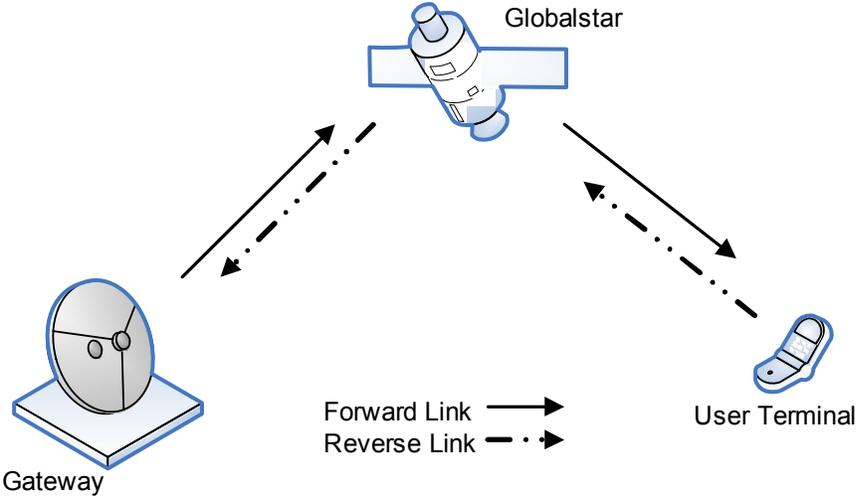
Figure 3.1. The Globalstar Satellite System Model
