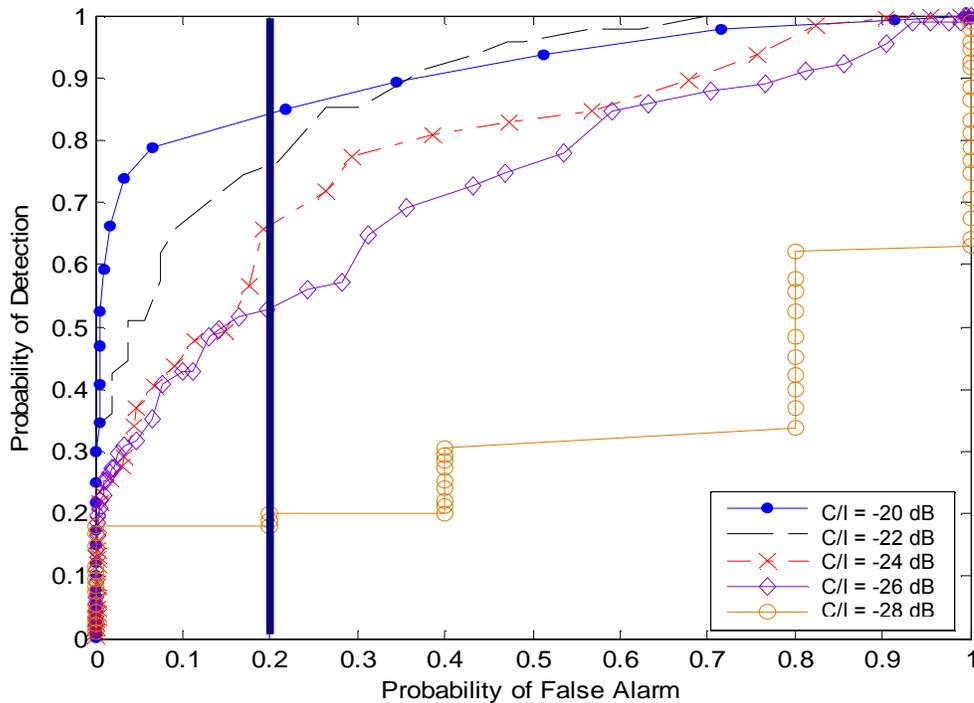
Figure 6.5. Results of Threshold Analysis for multi-user C/I values of -20, -22, -24, -26, and -28 dB. The solid vertical line represents the Probability of False Alarm used in the mean acquisition time analysis below.
