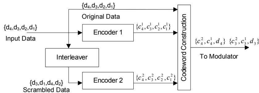
Figure 4.7. Turbo encoder block diagram. (From Figure 4 of [55], © The Aerospace Press. Reproduced with permission.)
