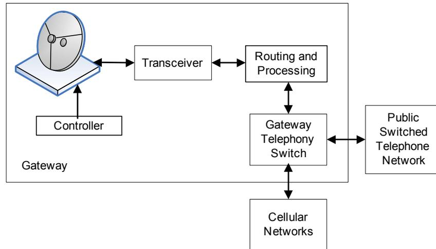
Figure 3.2. Globalstar gateway block diagram [11]
