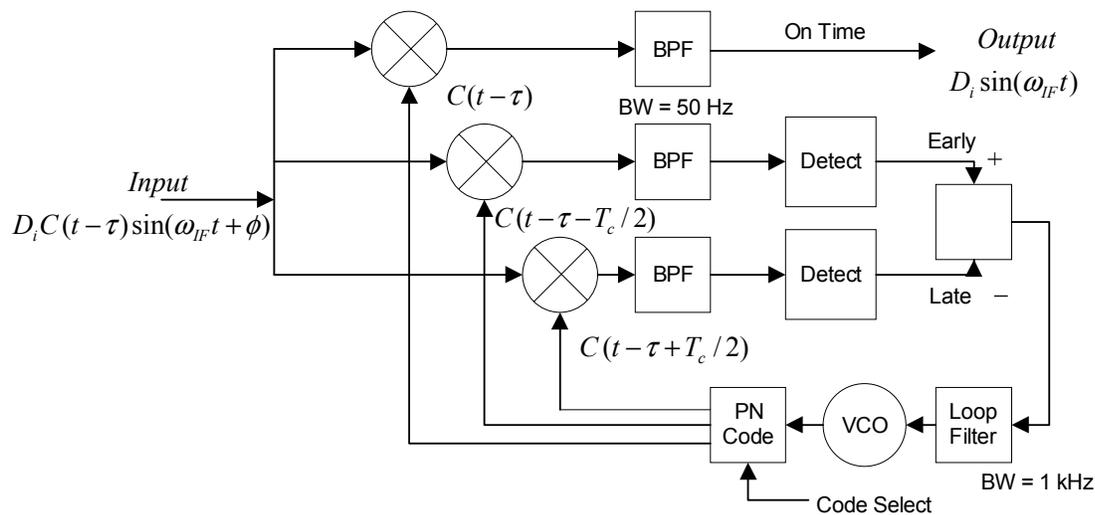
Figure 4.8. GPS Early-Late Gate Receiver Block Diagram
