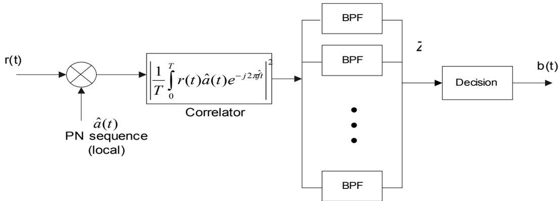
Figure 5.3. Block diagram of a Globalstar System receiver. The received signal is the transmitted signal plus noise from the channel:  $r(t) = s(t) + n(t)$ . The locally generated PN sequence,  $\hat{a}(t)$ , will not be correctly aligned with the transmitted PN sequence in either time or frequency. The decision device examines the output from the correlator ( $Z$ ) and determines the correct code alignment. (Reproduced from [6] with permission.)
