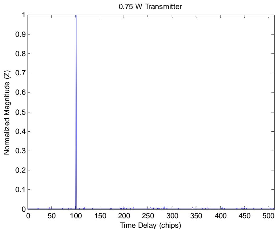
Figure 6.1. Output of correlator for a single user with known code with 100 chip time shift and no Doppler shift. The code length was 2046, the integration time was 512 chips, and the  $C/N$  was -3.7 dB. The correlation peak is at  $NT_c=101$  chips, as expected.
