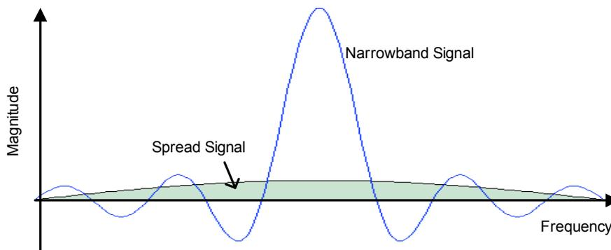
Figure 4.1 Direct Sequence – Spread Spectrum Waveform (spread signal). The Narrowband data represents the signal before spreading.
