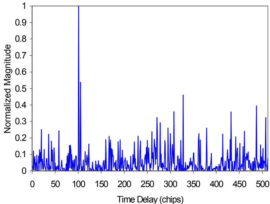
Figure 6.3. Output of correlator for a known code with 100 chip time shift and no Doppler shift. The code length was 2046, the integration time was 512 chips, and the C/I was -26 dB. The user transmit power was 50 mW for 165 simultaneous users in the satellite transponder. The correlation peak is at  $NT_c=101$  chips, as expected.
