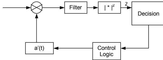
Figure 4.4 Spread Spectrum Receiver Block Diagram (Reproduced from [6] with permission.)
