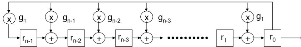
Figure 4.2. Modular Format of Feedback Shift Register for generating m-sequences. The initialization vector is represented by  $r_{n-1}, \dots, r_0$ , and the coefficients of the generator polynomial are denoted by  $g_n, \dots, g_1$ . (Reproduced from [6] with permission.)
