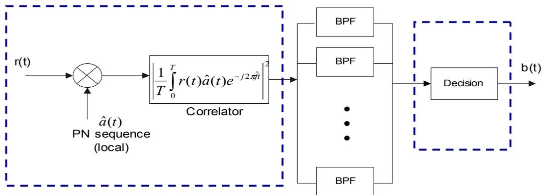
Figure 5.4. Block diagram of simulated Globalstar system receiver. The portions of the receiver inside the dashed lines were the only portions of the receiver simulated. Because of this, the decision statistic relies only on the output of the correlator, rather than the combined outputs of both the correlator and the filter bank. The decision device examines the output from the correlator ( $Z$ ) and determines the correct code alignment.
