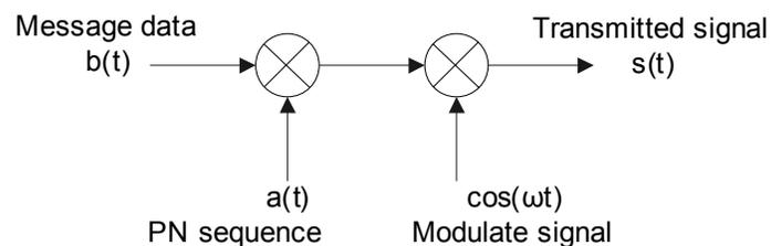
Figure 5.2. Block diagram of a generic RF section of a Globalstar transmitter. Both code and data modulation is BPSK, and the data is modulated with a carrier frequency of  $\omega$  rad/sec. (Reproduced from [6] with permission.)
