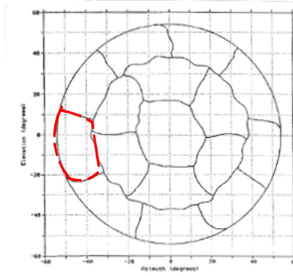
Figure 3.4. Beam pattern for a Globalstar System satellite beam (footprint) © [1998] IEEE. Reprinted, with permission, from [11]
