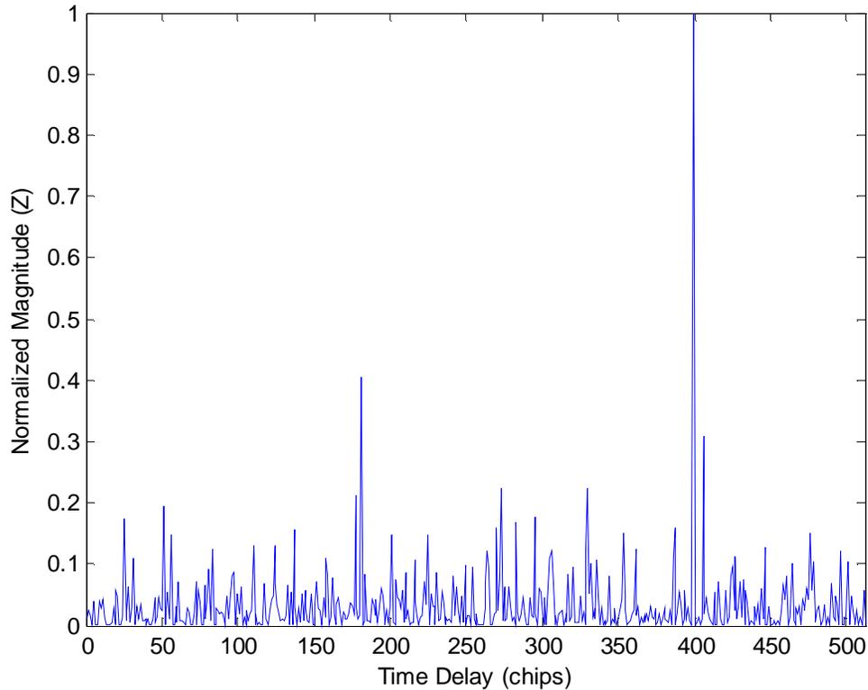
Figure 6.4. Output of correlator for a known code with 398 chip time shift and no Doppler shift. The code length was 2046, the integration time was 512 chips, and the C/I was -24 dB, which corresponds to a transmit power of 75 mW with 165 users in the satellite transponder. The correlation peak is at  $NT_c=399$  chips, as expected.
