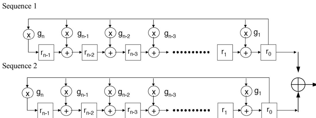
Figure 4.3. Gold Sequence Generator. The initialization vector is represented by  $r_{n-1}, \dots, r_0$ , and the coefficients of the generator polynomial are denoted by  $g_n, \dots, g_1$ . (Reproduced from [6] with permission.)
