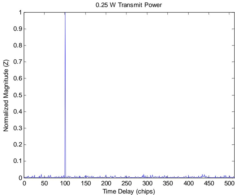
Figure 6.2. Output of correlator for a single user with a known code with a 100 chip time shift and no Doppler shift. The code length was 2046, the integration time was 512 chips, and the C/N was -8.5 dB, which corresponds to a 0.25 W transmit power. The correlation peak is at  $NT_c=101$  chips, as expected.
