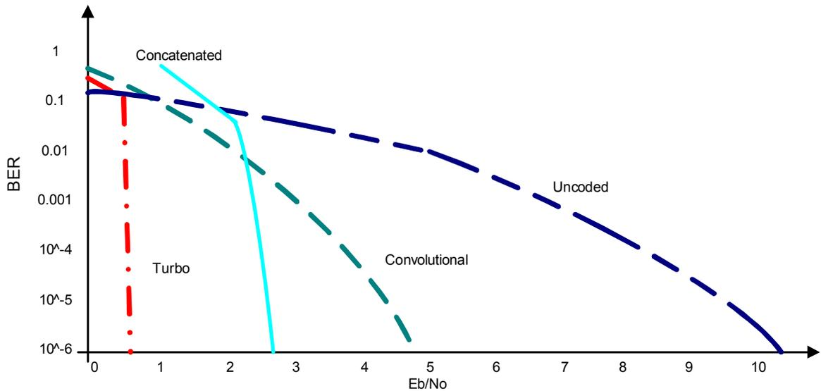
Figure 4.5  $E_b/N_0$  vs. BER for different forward error correction codes: Turbo coding, Convolutional coding, Concatenated coding, and no coding. (From Figure 2 of [55], © The Aerospace Press. Reproduced with permission.)
