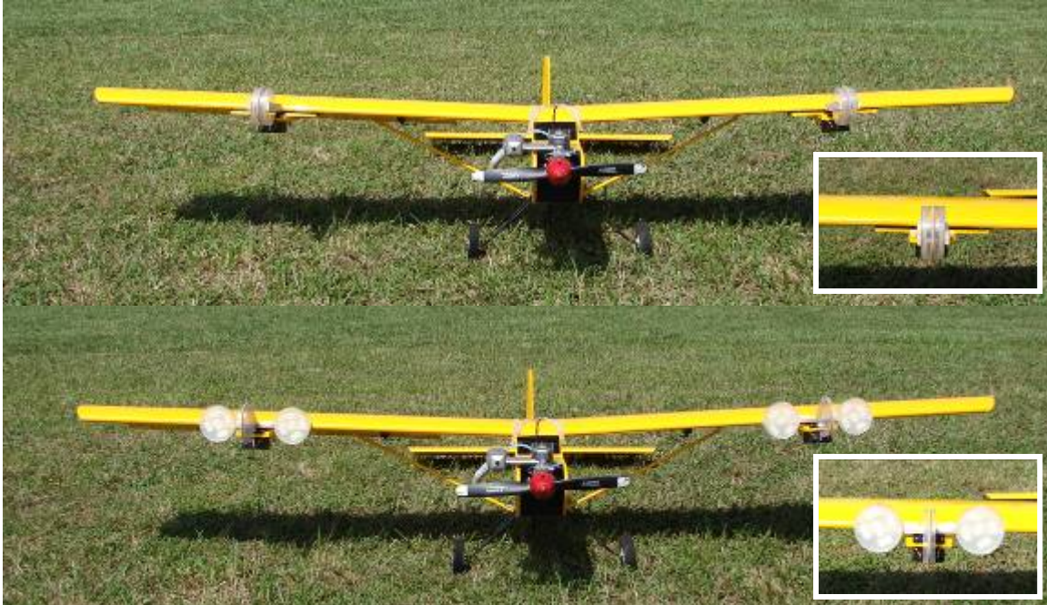
Figure 2.9. New and improved design of spore-samplers on the autonomous Senior Telemaster ARF. The spore-samplers open (bottom) and close (top) on the leading edge of the wing.
