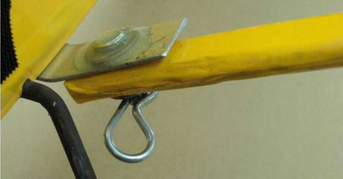
Figure 2.5. Wing strut attachment method on the Senior Telemaster ARF.
