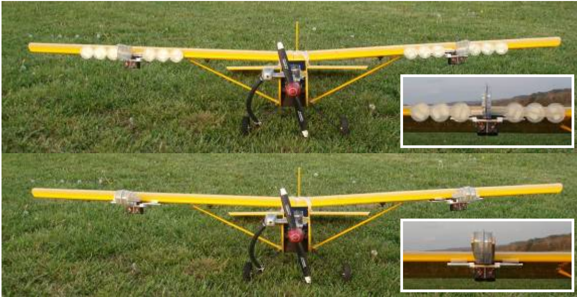
Figure 4.5. Redesigned sampling devices allow for greater flexibility of media used.
