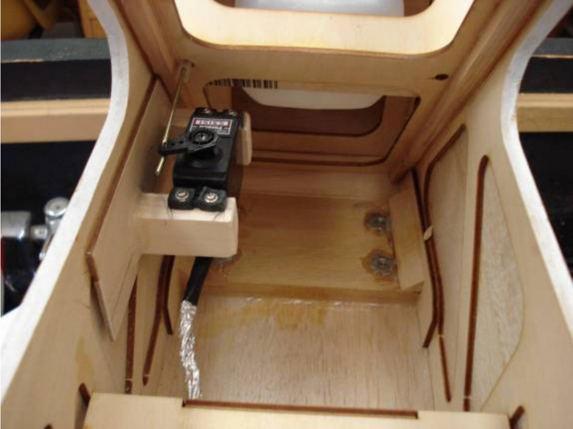
Figure 4.2. Relocated throttle servo to create space for autonomous unit and ensure consistent throttle response.
