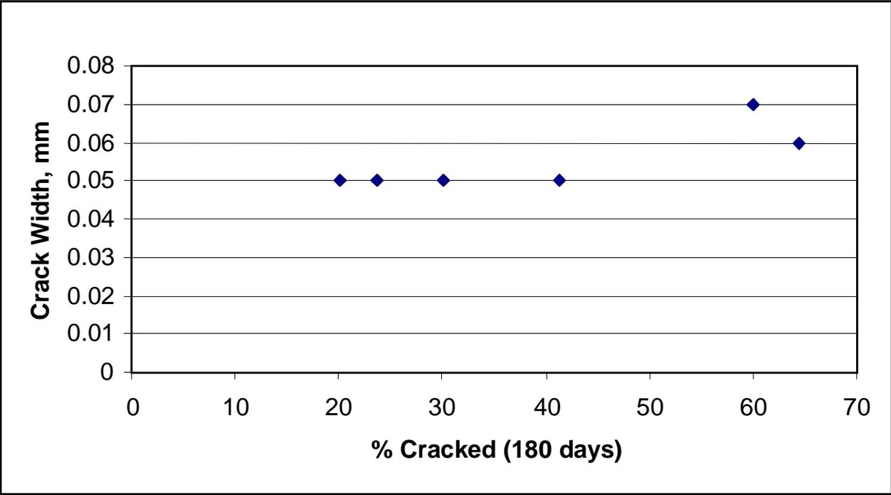
**Figure 6-8:** Surface Crack Width as a Function of Percent Surface Cracking, 813 mm (32 in.) Square, PC/GGBFS Concrete (Batch 1).
