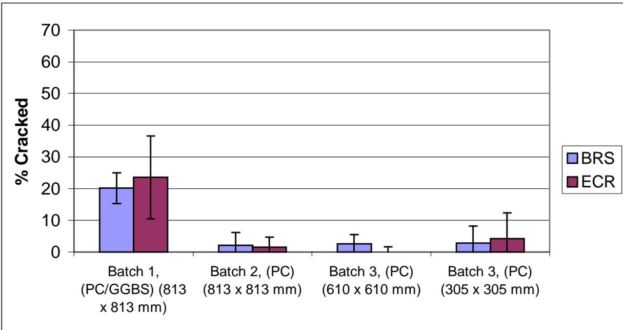
**Figure 6-7:** Percent Cracking in Specimens, 50.8 mm (2.0 in.) Concrete Cover Depth, 180 Days.
