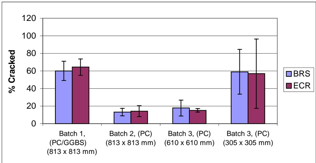
**Figure 6-5:** Percent Cracking in Specimens, 38 mm (1.5 in.) Concrete Cover Depth, 180 Days.
