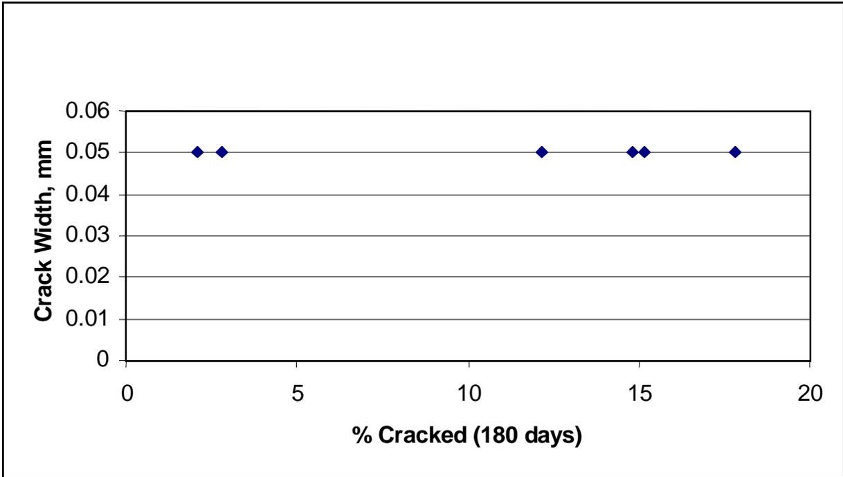
**Figure 6-10:** Surface Crack Width as a Function of Percent Surface Cracking, 610 mm (24 in.) Square, PC Concrete (Batch 3).
