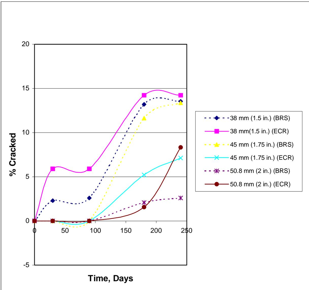
**Figure 6-2:** Percent Surface Cracking Propagation in 813 mm (32 in.) Square Specimens, PC (Batch 2).
