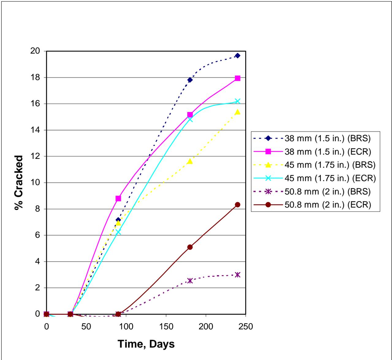
**Figure 6-3:** Percent Surface Cracking Propagation in 610 mm (24 in.) Square Specimens, PC (Batch 3).
