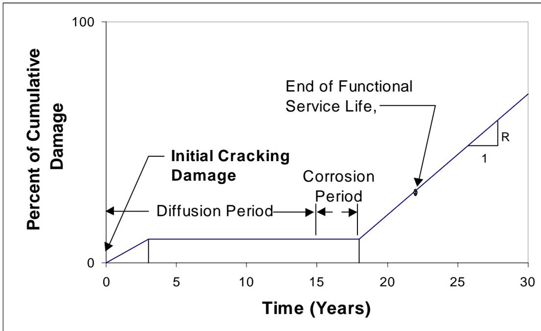
**Figure 1-1:** Concrete Service Life Model Relative to Corrosion Deterioration (Weyers, 1998)
