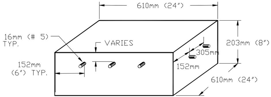
**Figure 5-2a: Isometric Diagram for 610 mm (24 in.) Specimen Size**
