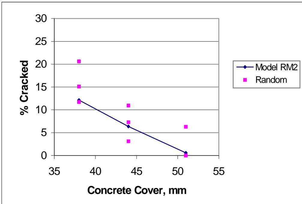
**Figure 7-1c:** Comparison of Actual Versus Computed Degree of Specimen Cracking (Model RM2). Batch 2 (PC), 813 mm (32 in.) Square Specimen Size, 200 mm (8 in.) Bar Spacing.
