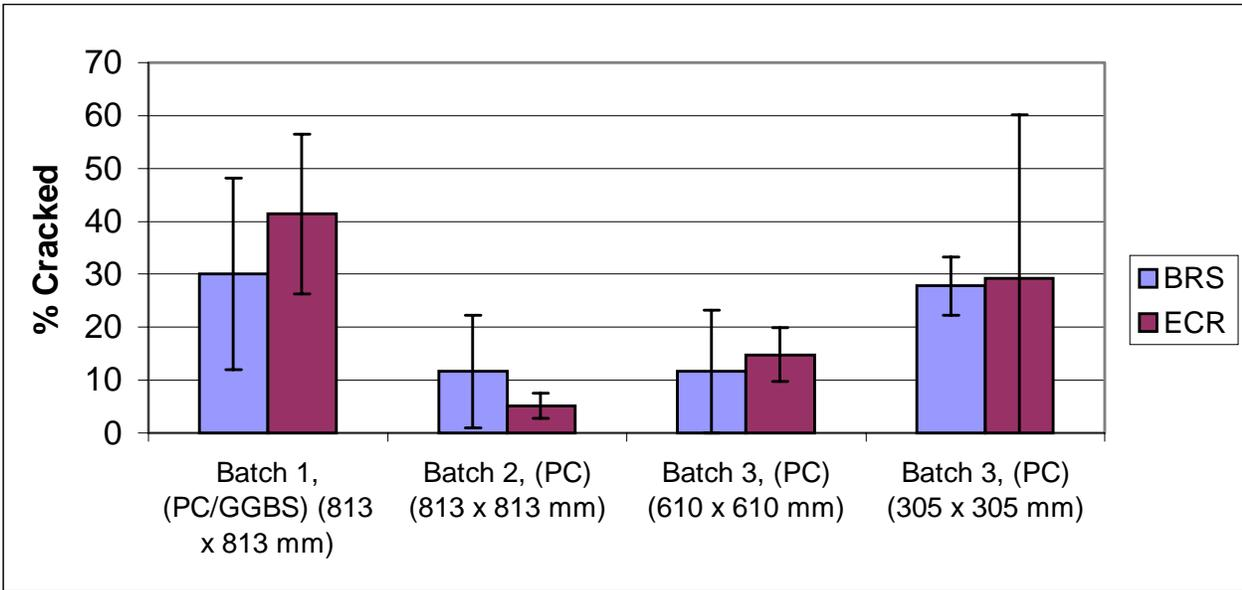
**Figure 6-6:** Percent Cracking in Specimens, 44.5 mm (1.75 in.) Concrete Cover Depth, 180 Days.
