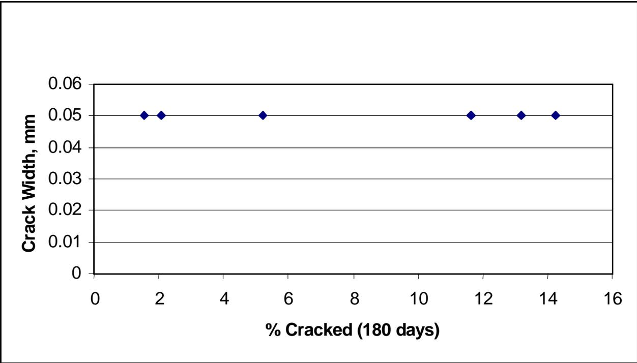
**Figure 6-9:** Surface Crack Width as a Function of Percent Surface Cracking, 813 mm (32 in.) Square, PC Concrete (Batch 2).
