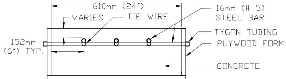
**Figure 5-2b: Form and Specimen Diagram for 610 mm (24 in.) Specimen Size**
