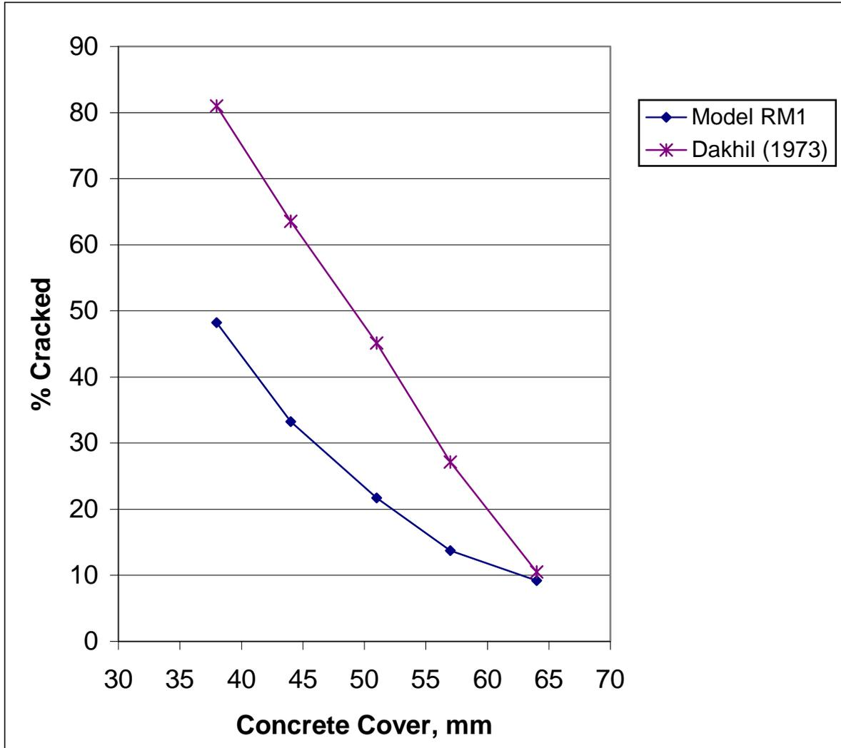
**Figure 7-2:** Comparison of Actual and Computed Results with the Regression Model Reported by Dakhil. Batch 3 (PC), 305 mm (12 in.) Square Specimen Size.
