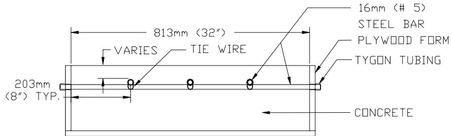
**Figure 5-1b:** Form and Specimen Diagram for 813 mm (32 in.) Specimen Size
