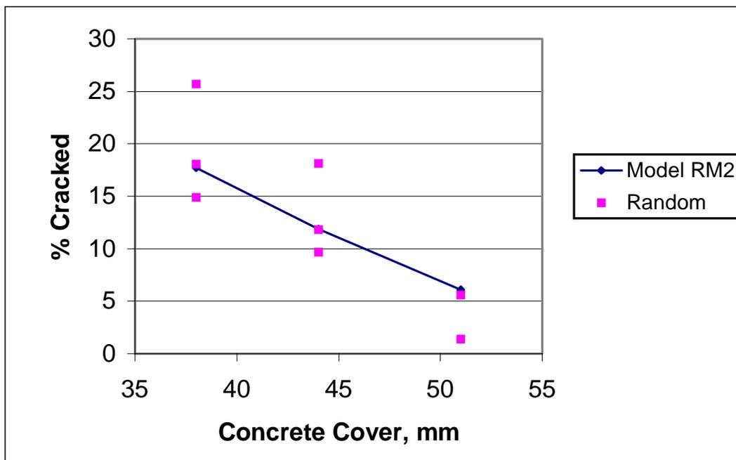
**Figure 7-1b:** Comparison of Actual Versus Computed Degree of Specimen Cracking (Model RM2). Batch 3 (PC), 610 mm (24 in.) Square Specimen Size, 150 mm (6 in.) Bar Spacing.
