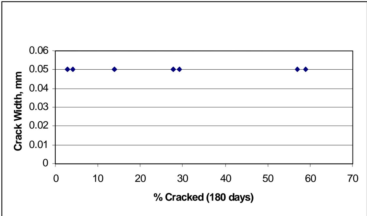
**Figure 6-11:** Surface Crack Width as a Function of Percent Surface Cracking, 305 mm (12 in.) Square, PC Concrete (Batch 3).
