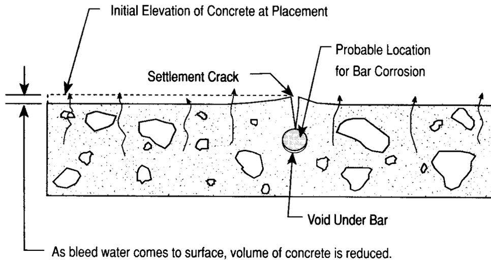
**Figure 1-2:** Subsidence Cracking of Concrete over Steel Reinforcement. (Emmons, 1993)
