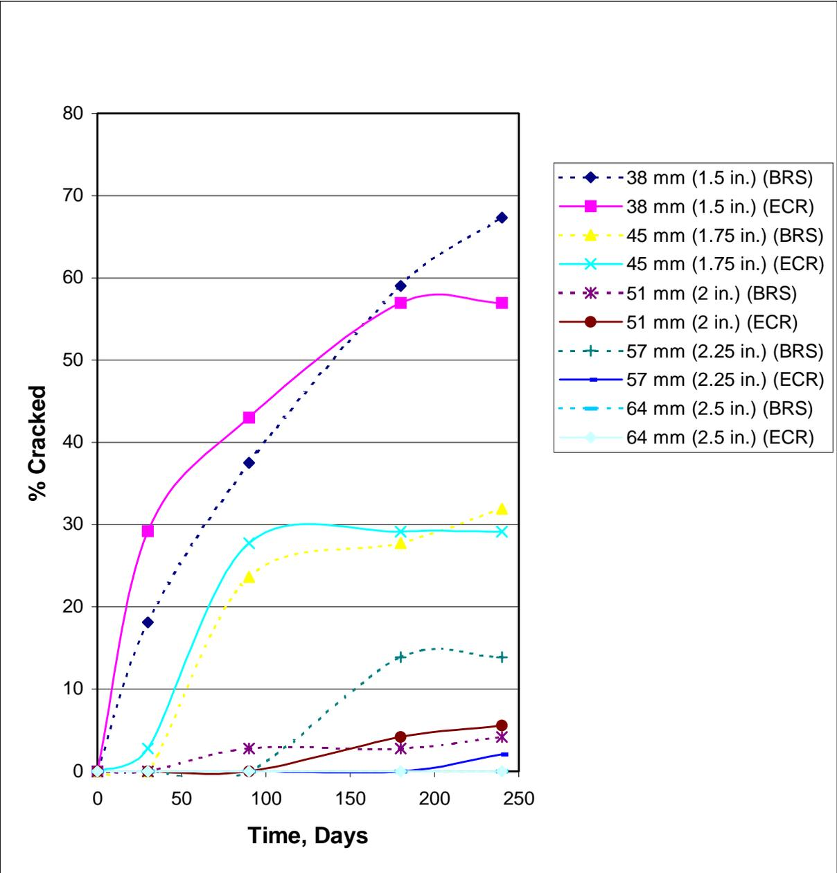
**Figure 6-4:** Percent Surface Cracking Propagation in 305 mm (12 in.) Square Specimens, PC (Batch 3).
