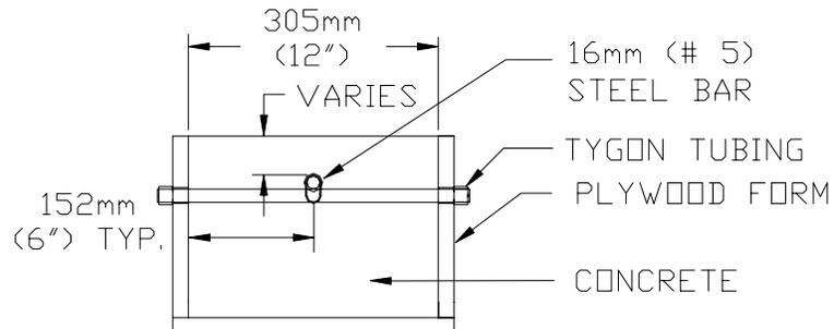
**Figure 5-3b: Form and Specimen Diagram for 305 mm (12 in.) Specimen Size**
