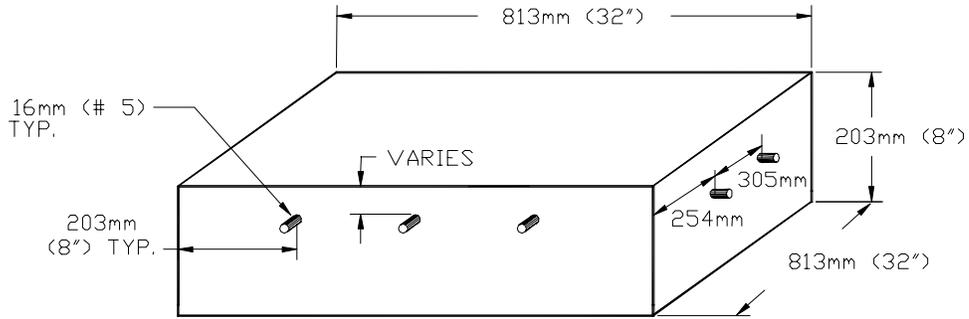
**Figure 5-1a:** Isometric Diagram for 813 mm (32 in.) Specimen Size
