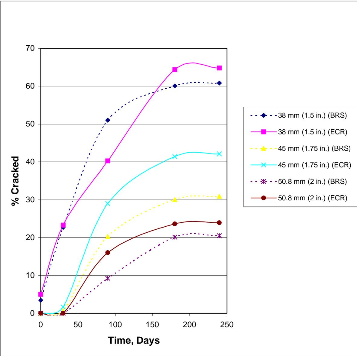
**Figure 6-1:** Percent Surface Cracking Propagation in 813 mm (32 in.) Square Specimens, GGBFS/PC (Batch 1).
