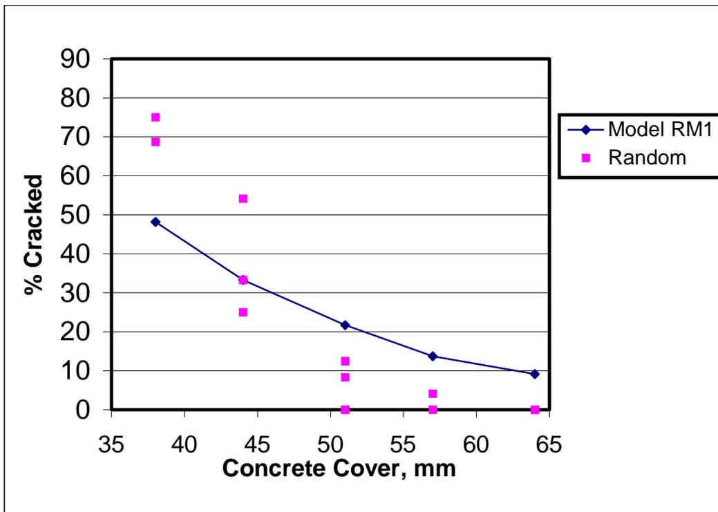
**Figure 7-1a:** Comparison of Actual Versus Computed Degree of Specimen Cracking (Model RM1). Batch 3 (PC), 305 mm (12 in.) Square Specimen Size
