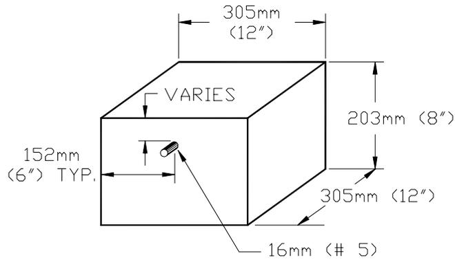
**Figure 5-3a: Isometric Diagram for 305 mm (12 in.) Specimen Size**
