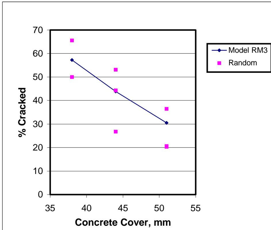
**Figure 7-1d:** Comparison of Actual Versus Computed Degree of Specimen Cracking (Model RM3). Batch 1 (PC/GGBFS), 813 mm (32 in.) Square Specimen Size, 200 mm (8 in.) Bar Spacing.
