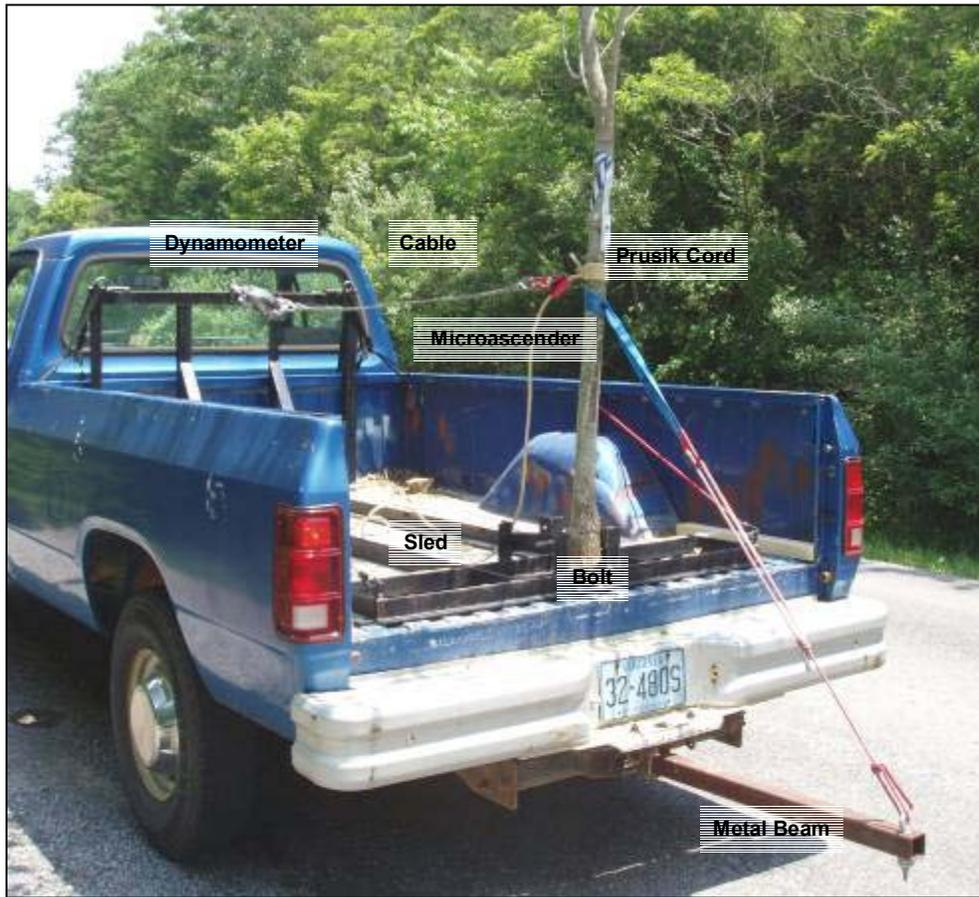
**Figure 3.5** – A custom-made, steel-framed sled equipped with a digital dynamometer (ED Junior 5K, Dillon/Quality Plus Inc., Kansas City, MO) mounted in the bed of a full-size, pick-up truck was used to measure the wind load imposed on 6.4 cm diameter white ash (*Fraxinus americana* L. ‘Autumn Purple’) trees driven at progressively increasing speeds.
