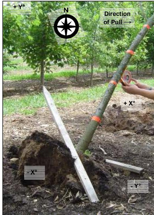
**Figure 3.2** – Trunk orientation (in X and Y planes) of 6.4 cm diameter balled-and-burlapped white ash (*Fraxinus americana* L. ‘Autumn Purple’) was measured using an angle gauge (Johnson 700 Magnetic Angle Locator, Johnson Level & Tool Mfg. Co., Mequon, WI) placed directly against the trunk 76 cm above ground line.
