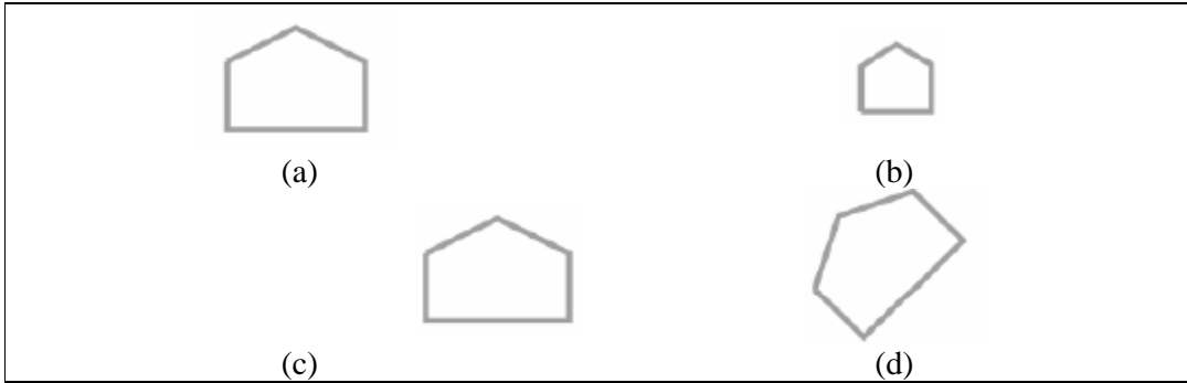
Figure 4.6: An example of geometrical transformations. (a) The original shape. (b) The same shape after a scaling effect. (c) The same shape after a translation effect. (d) The same shape under rotation.
