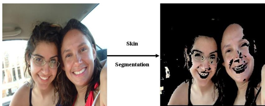
Figure 6.4: Example of skin segmentation using hardware software co-design features in Matlab, Simulink, and System Generator for DSP.
