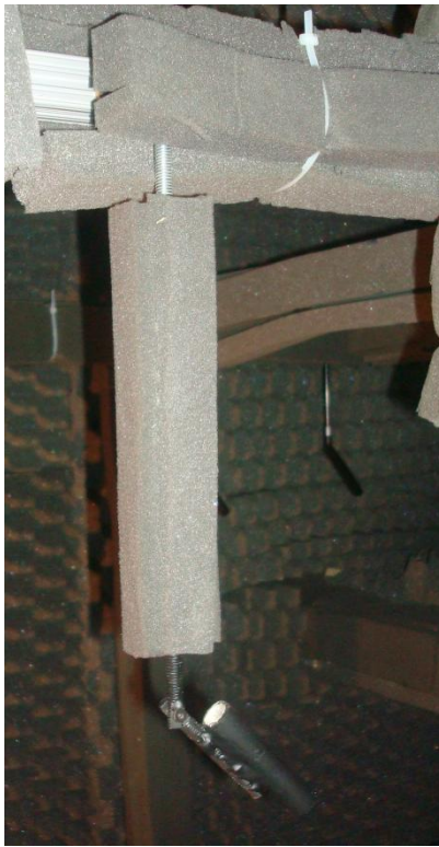
Figure 2-9 - Acoustically treated microphone mount
