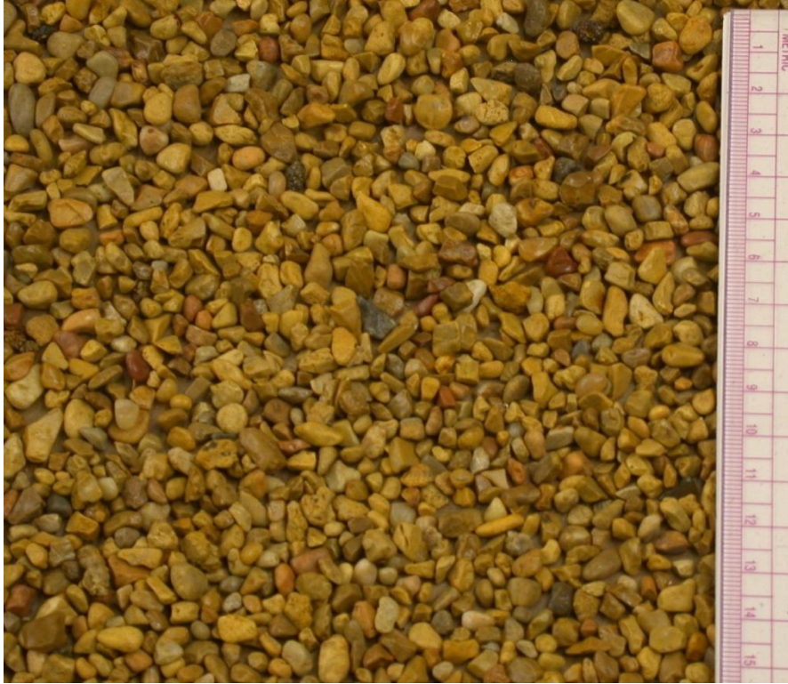
Figure 2-29 – Full fetch layout, 6mm gravel, scale in centimeters
