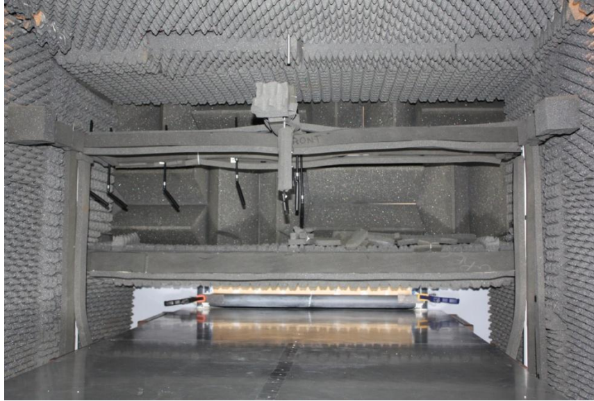
Figure 2-8 - Microphone traverse system, showing acoustic treatment and microphone stands
