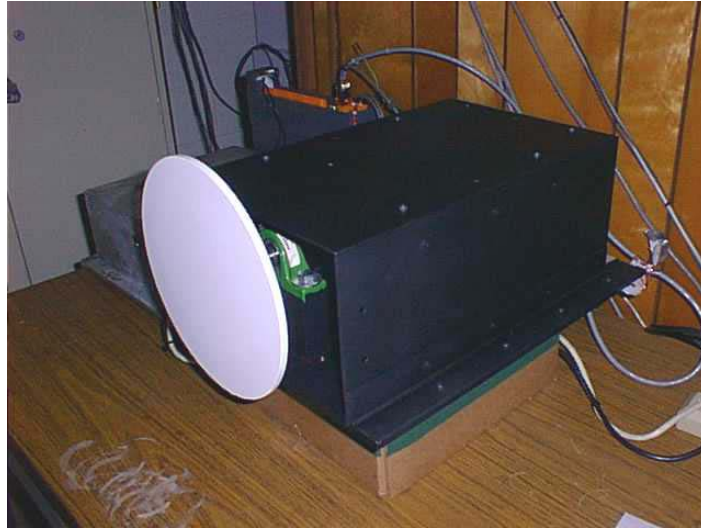
Figure 2.12: VT DGV calibration wheel
