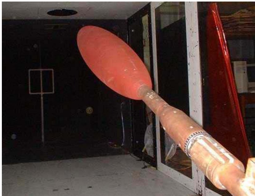
Figure 2.16: 6:1 prolate spheroid mounted in wind tunnel test section.
