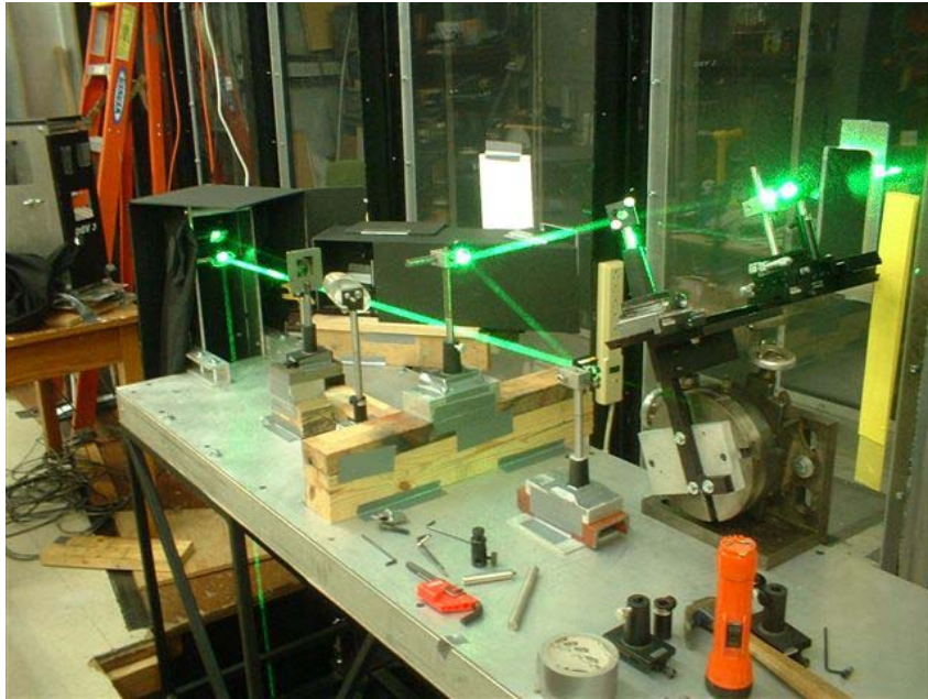
Figure 3.10: Setup for the laser optics used to form the laser sheet.
