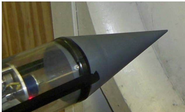
Figure 3-12: Propeller test rig sealing
