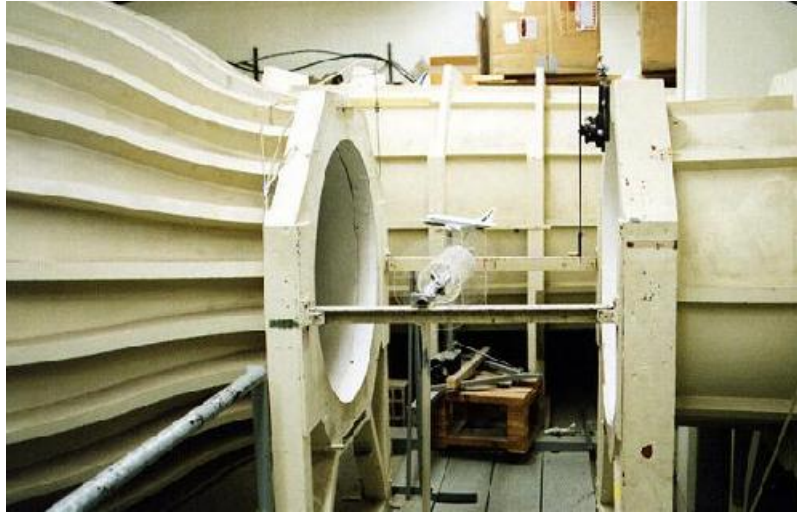
Figure 3-1: View of test section and return of the Instructional Tunnel [9]
