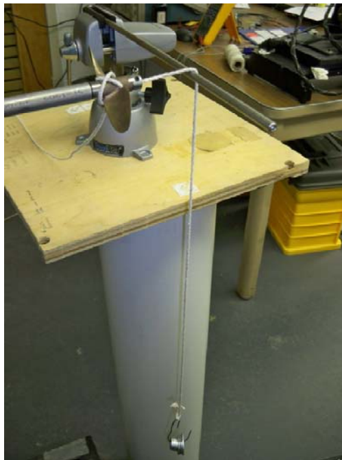
Figure 3-16: Propeller test rig load cell calibration process
