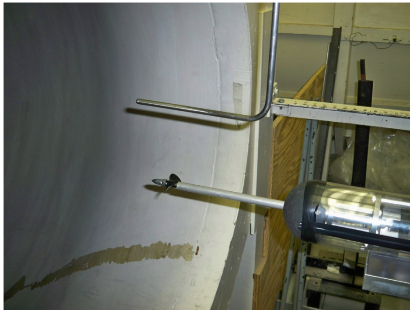
Figure 3-3: Pitot-static probe relative to propeller rig
