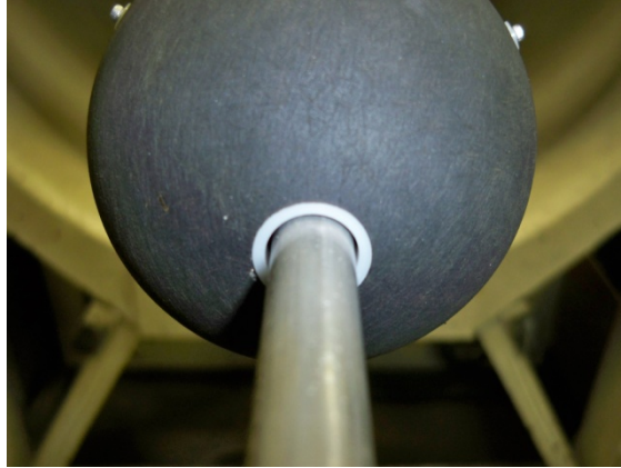
Figure 3-11: Propeller test rig shaft to nose tolerance
