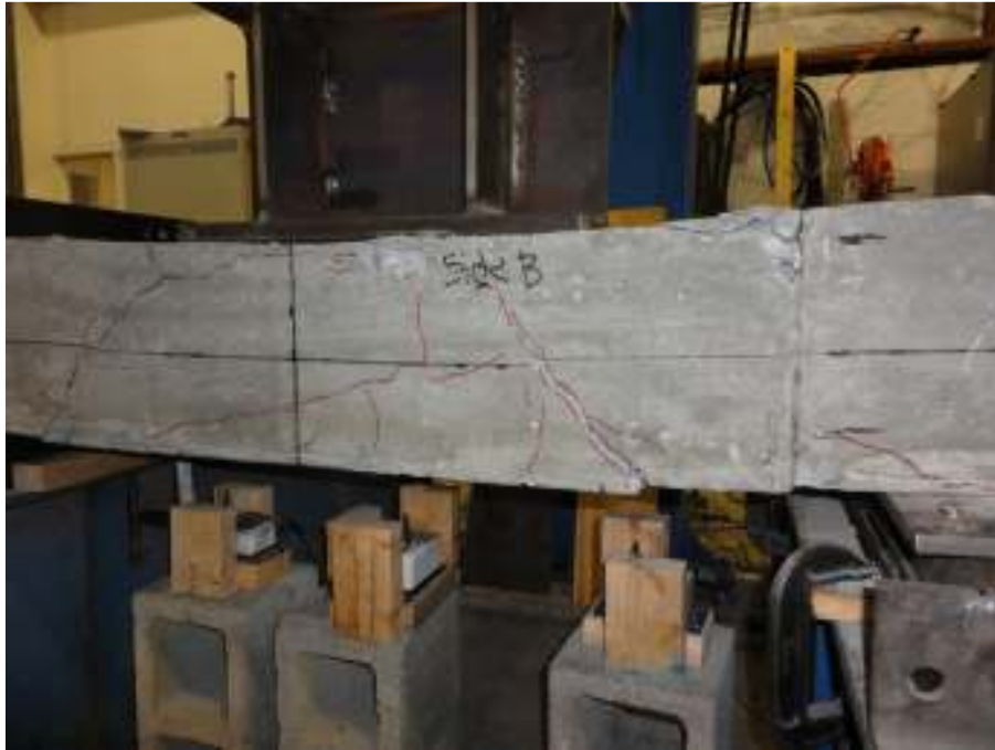
Figure D-11. Side B View of Failed Specimen B with Focus on Joint 2
