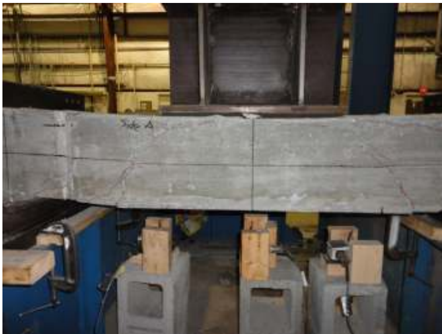
Figure D-10. Side A View of Failed Specimen B with Focus on Joint 2 and Main Cracks
