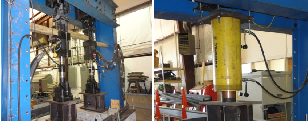
Figure 3-14. Actuators Used for Testing (MTS on Left, Enerpac on Right)
