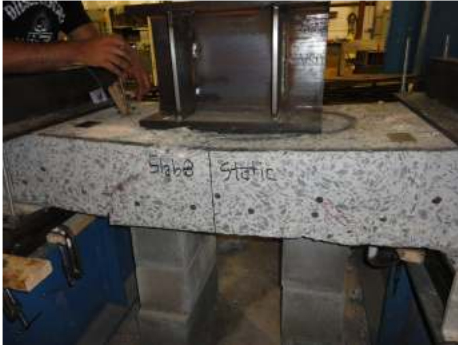
Figure D-5. Side A View of Failed Specimen 8
