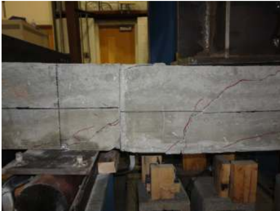
Figure D-12. Side B View of Failed Specimen B with Focus on Joint 1
