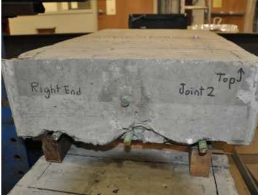
Figure D-17. End Face of Joint 2 with Failed Top Rebar (Bottom Bars Were Cut)
