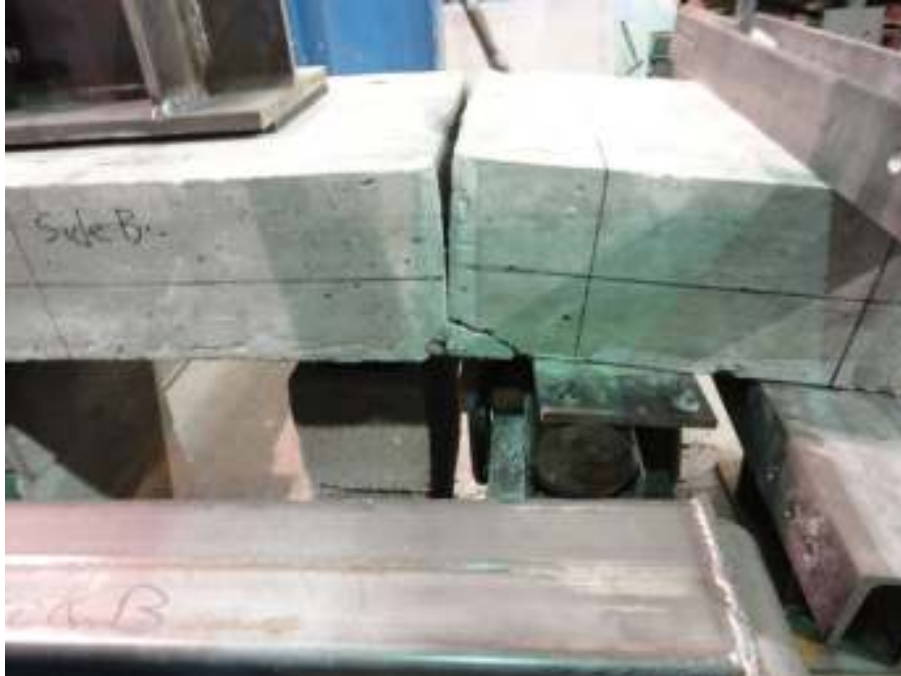
Figure D-15. Joint 2 with Jacking Struts and Connections Removed
