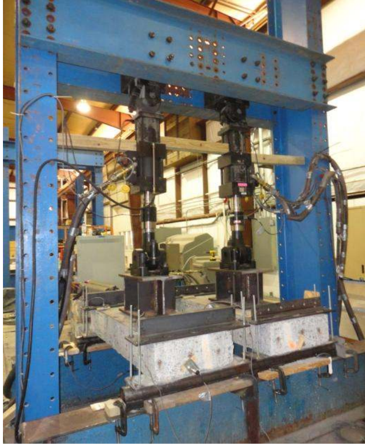
Figure 3-9. Complete Setup for Fatigue Loading
