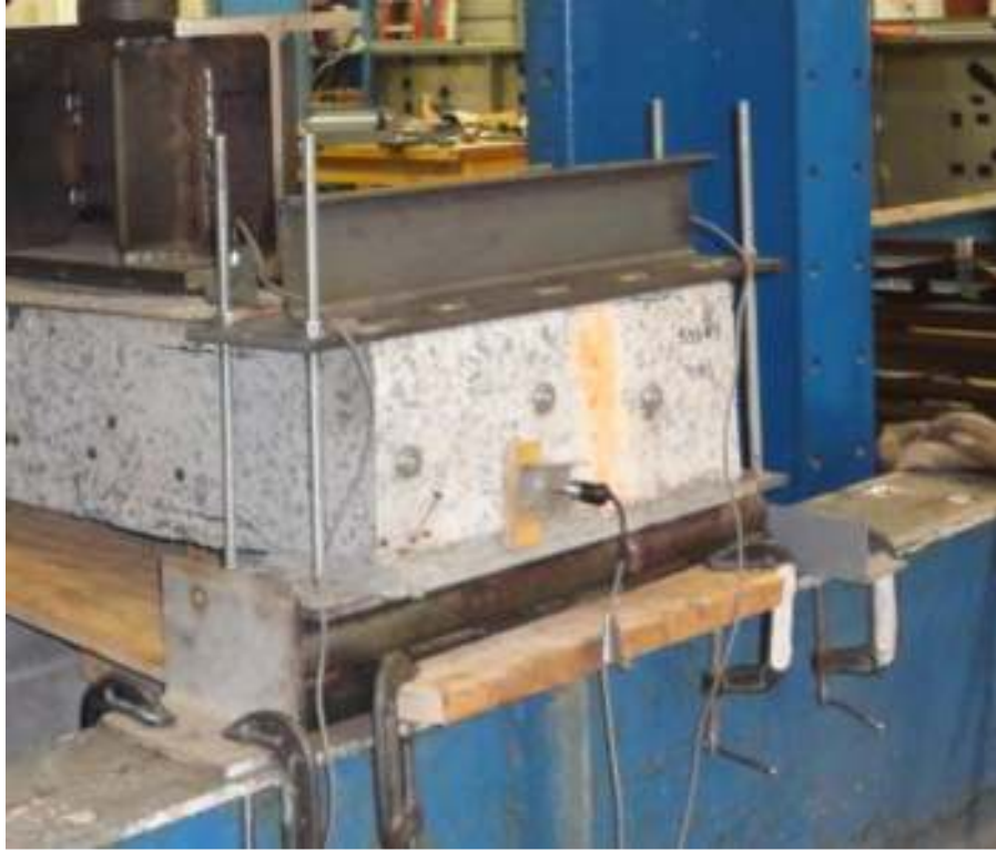
Figure 3-12. Steel Plate Assembly at Support Locations with Grout Layer
