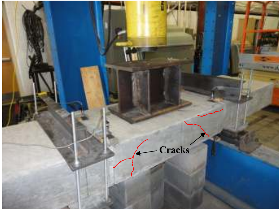
Figure 5-6. Failed Specimen C with Main Cracks Indicated
