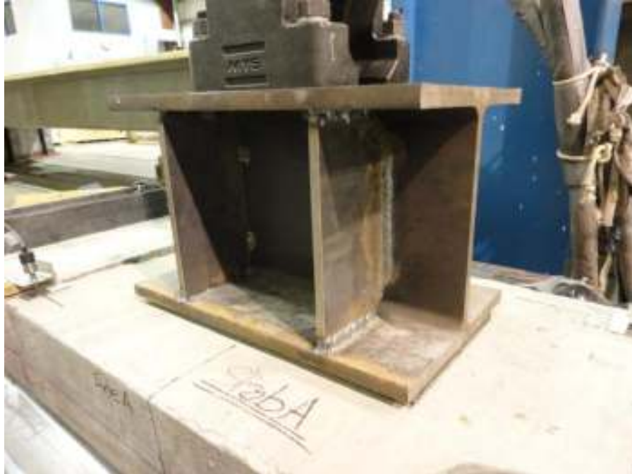
Figure 3-13. Stiffened W12x87 Section Used as Loading Extension
