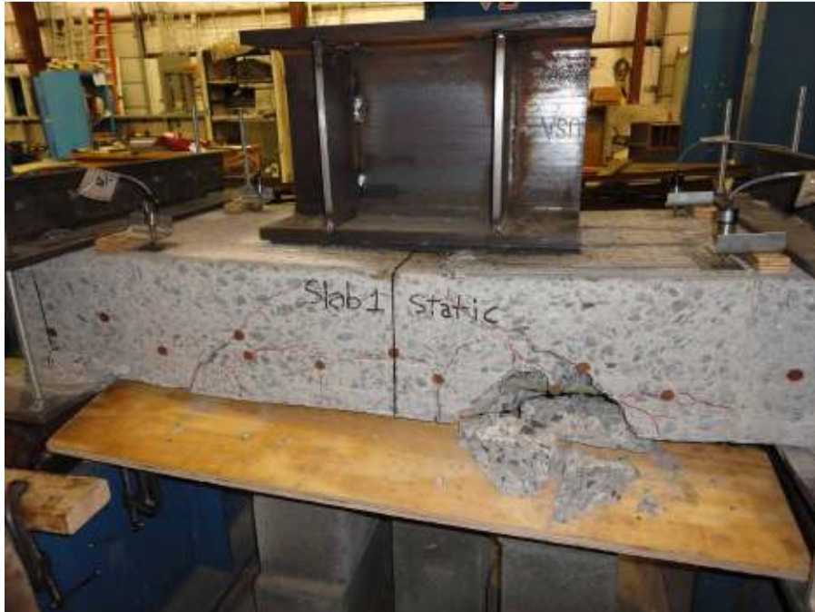
Figure 5-4. Failed I-81 Specimen with Test-Induced Cracks (Marked in Red)
