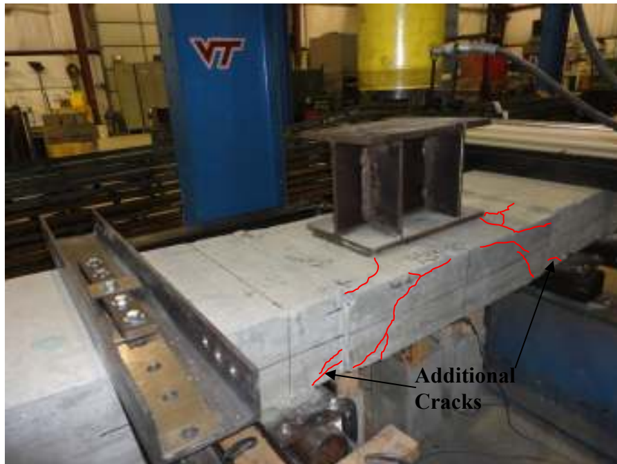
Figure 5-13. Failed Specimen B with Test-induced Cracks Marked
