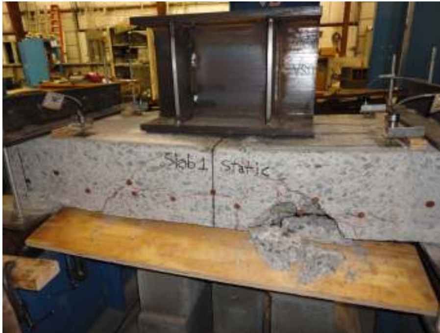
Figure D-1. Side A View of Failed Specimen 1
