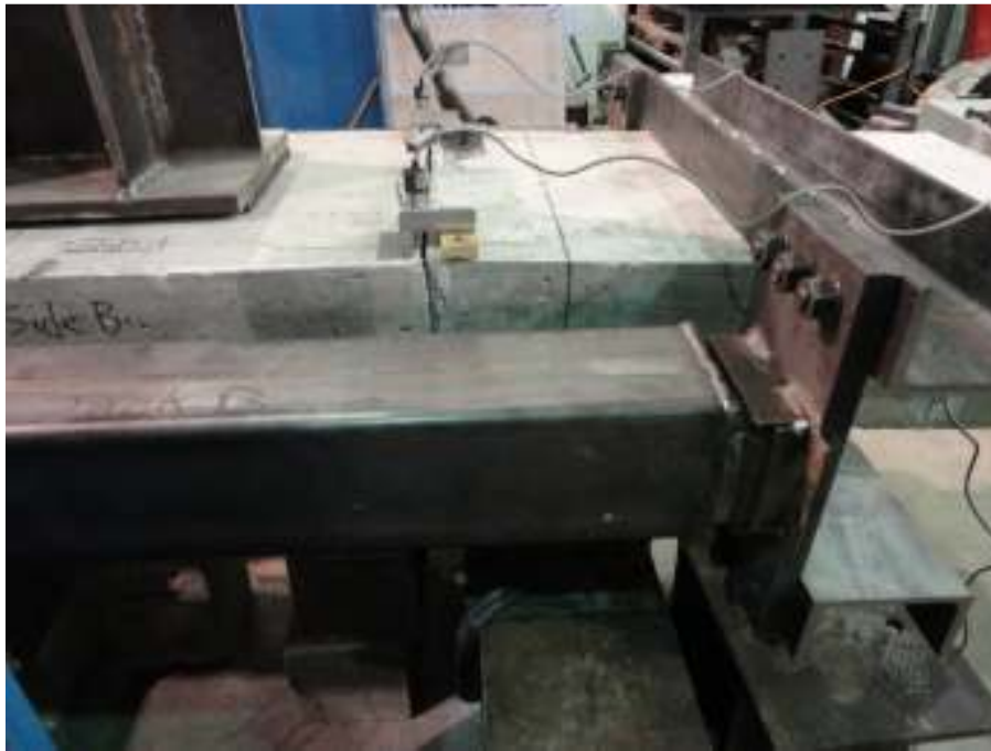
Figure D-13. Joint 2 after Top Rebar Failed in Fatigue (Jacking Setup in Place)
