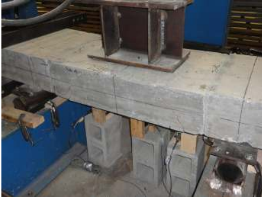
Figure D-9. Side A View of Failed Specimen B
