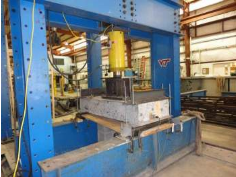
Figure 3-10. Complete Setup for Strength Tests
