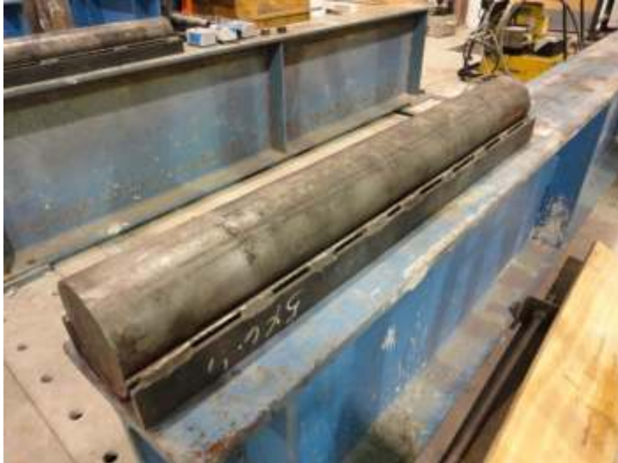
Figure 3-11. Roller-Type Support Used for all Tests
