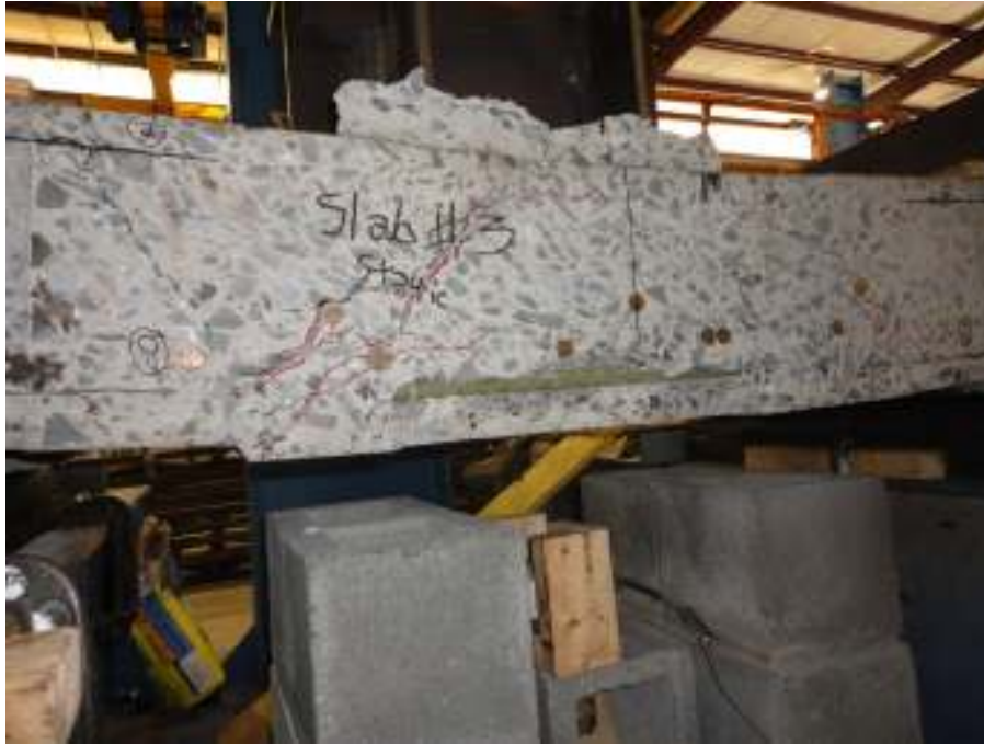
Figure D-3. Side A View of Failed Specimen 3
