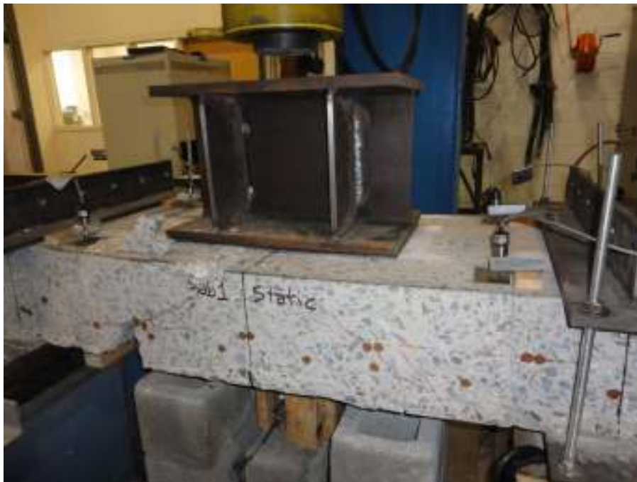
Figure D-2. Side B View of Failed Specimen 1
