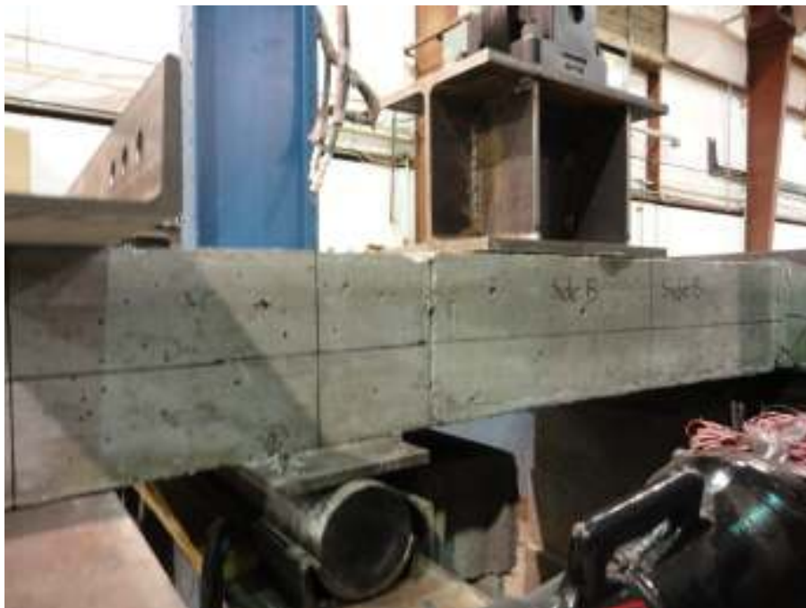
Figure D-16. Joint 1 with Jacking Struts and Connections Removed (No Failed Fatigue Rebars)
