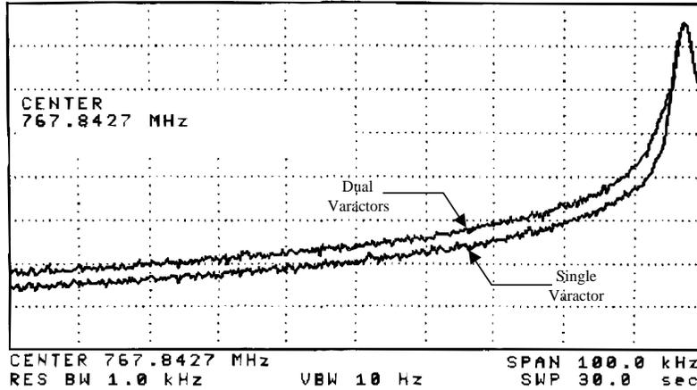
**Figure 5.20. Sideband oscillator noise spectrum using balanced tuning varactors vs. single varactor.**
