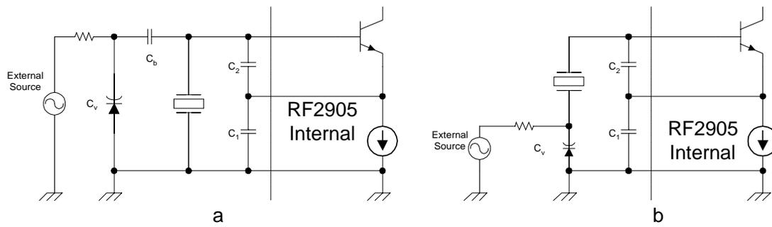
**Figure 5.18. (a) Parallel and (b) series mode oscillator pull setups.**
