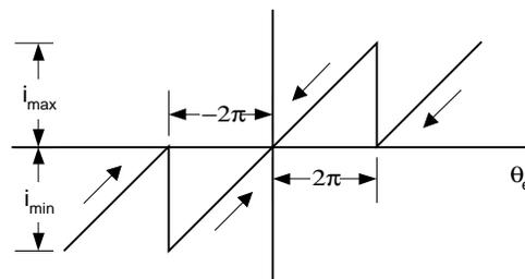
**Figure A.3. Phase-Frequency detector characteristic vs. phase error.**
