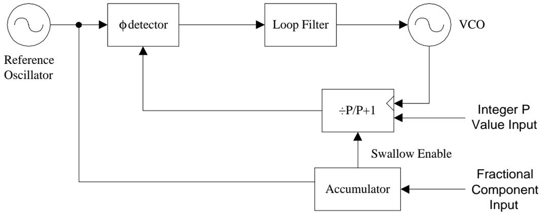
**Figure 7.2. Standard fractional-N frequency synthesizer without phase compensation.**
