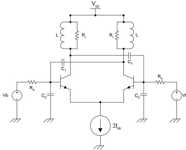
**Figure 5.11. Non-saturating balanced pair oscillator circuit.**
