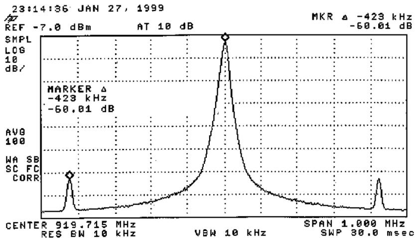
Figure 7.8. Output spectrum of implementation circuit with PLL bandwidth of 9 kHz.
