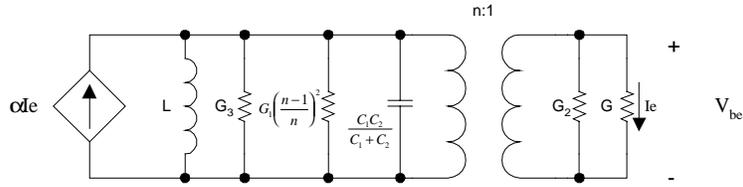
**Figure 5.6a. Equivalent circuit using ideal transformer.**
