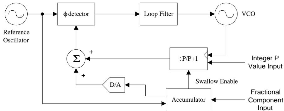
**Figure 7.13. Fractional-N with spurious signal compensation.**
