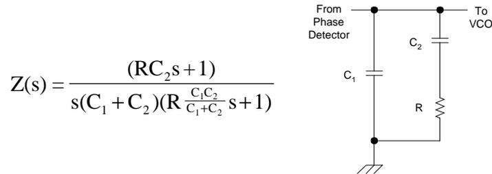
**Figure A.4. Third order loop filter and impedance transfer function.**
