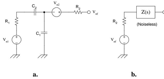
**Figure 6.4. Noise sources within the loop filter.**
