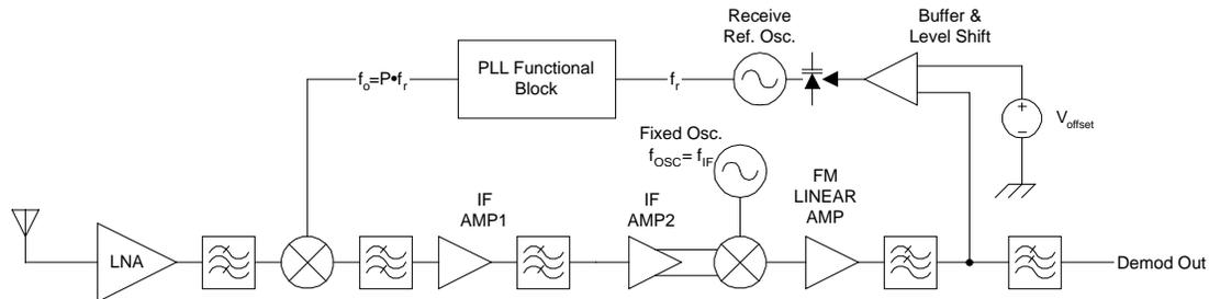
**Figure 3.11. Illustration of a potential RF2905 PLD setup.**
