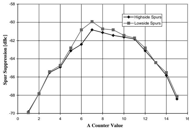
**Figure 7.9. Graph of base frequency spur amplitude relative to the carrier vs. A counter value.**
