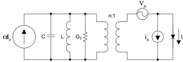
**Figure 5.21. Illustration of oscillator with transistor noise sources present.**
