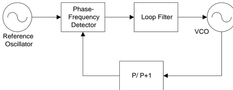
Figure A.1. PLL block diagram.
