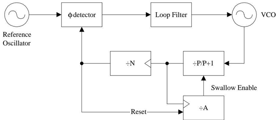
**Figure 7.1. Block diagram of PLL swallow counter frequency synthesizer.**
