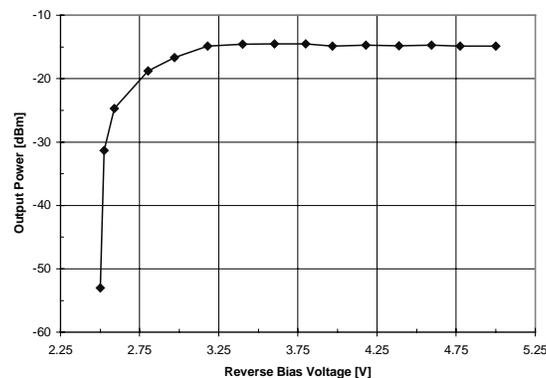
**Figure 5.16. Plot of RF2905 output power vs. varactor reverse bias voltage.**
