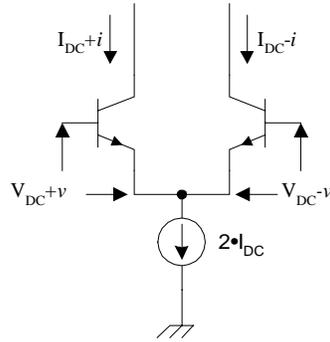
**Figure 5.7. Differential pair schematic.**
