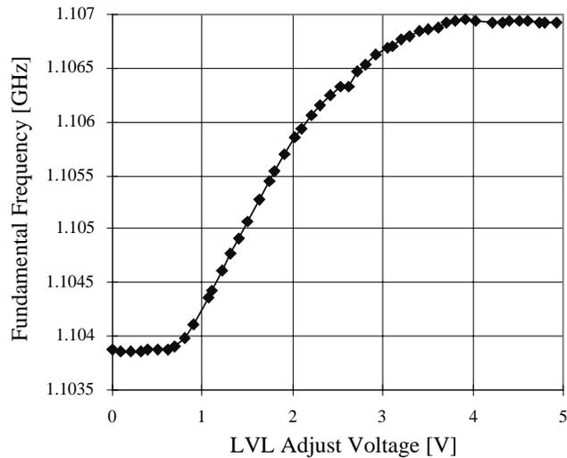
**Figure 4.3. Open loop VCO frequency vs. LVL ADJ voltage.**
