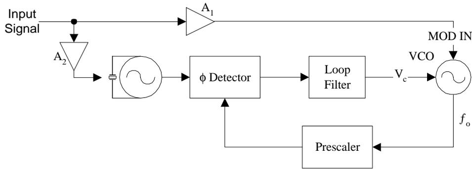
**Figure 4.8. Analog dual modulation technique.**
