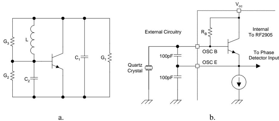
**Figure 5.1. General three node Colpitts oscillator circuit(a) and RF2905 reference oscillator(b).**
