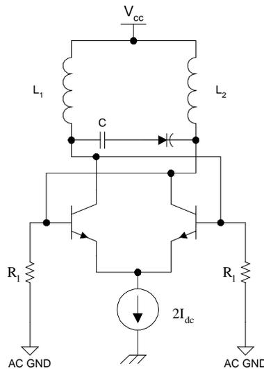
**Figure 5.14. Typical implementation of the saturating balanced pair oscillator.**
