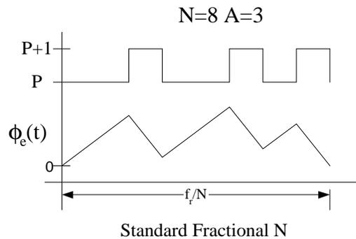
**Figure 7.12. Illustration of phase error and prescaler value for standard fractional-N technique.**
