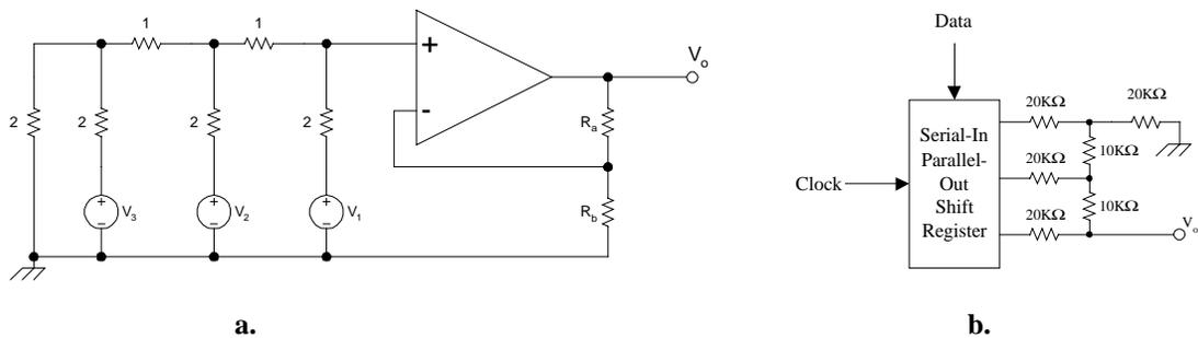
**Figure 4.10 D/A converter circuit typologies for multilevel FSK implementations.**
