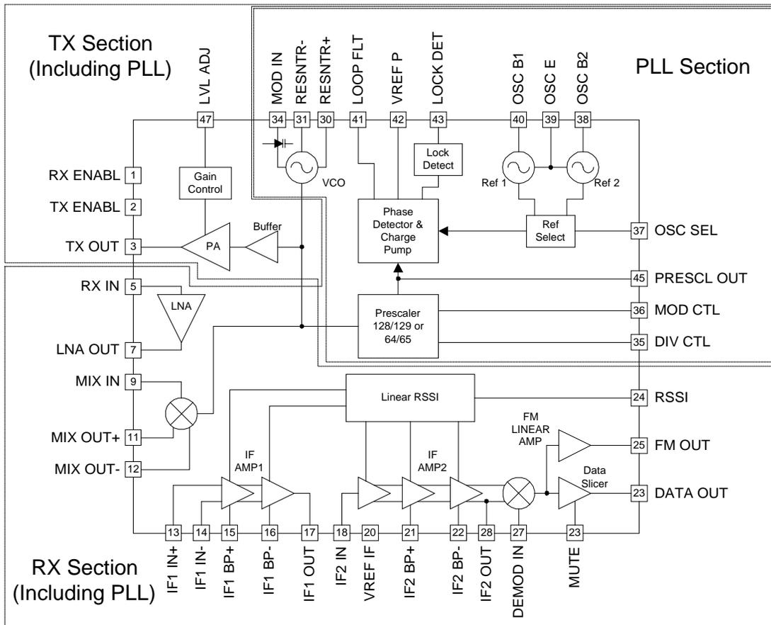
Figure 2.1. RF2905 functional block diagram from RF2905 data sheet.
