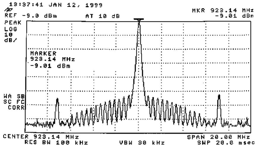
Figure 7.10. Illustration of two types of spurs resulting from fractional-N synthesis<sup>2</sup>.
