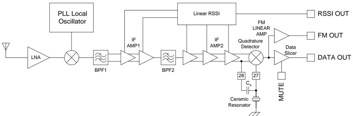
Figure 3.1. Manufacturer's suggested implementation of RF2905 receiver.
