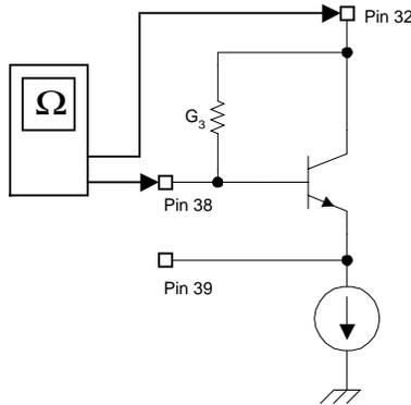
**Figure 5.2. Measurement of the bias resistor of the RF2905.**
