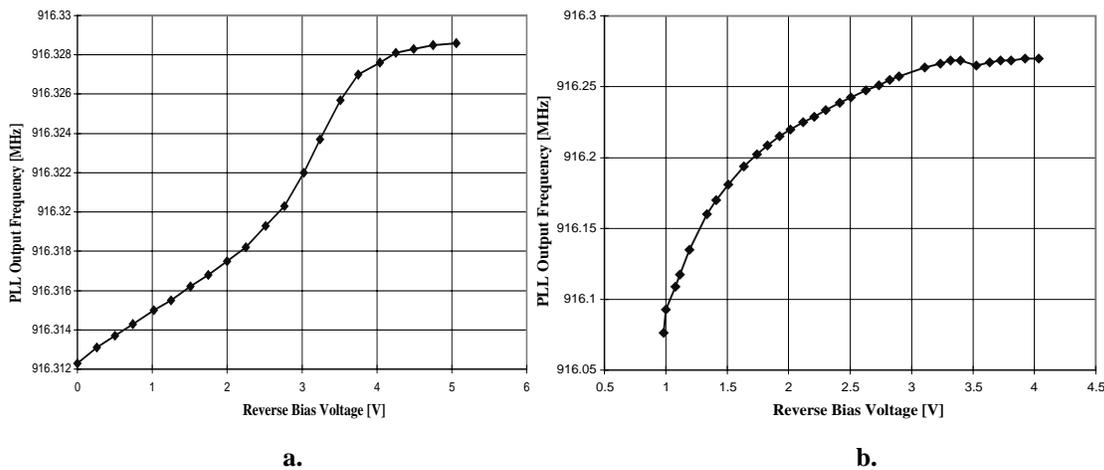
**Figure 5.19. Measured performance of (a) parallel and (b) series reference oscillator pull.**
