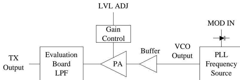
Figure 4.1. Block diagram of transmitter.
