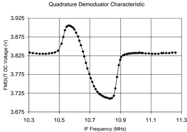
**Figure 3.10. Voltage vs. Frequency characteristic of quadrature detector.**
