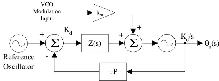
**Figure 4.6. PLL with direct modulation of the VCO.**
