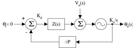
**Figure 6.5. Addition of loop filter noise.**
