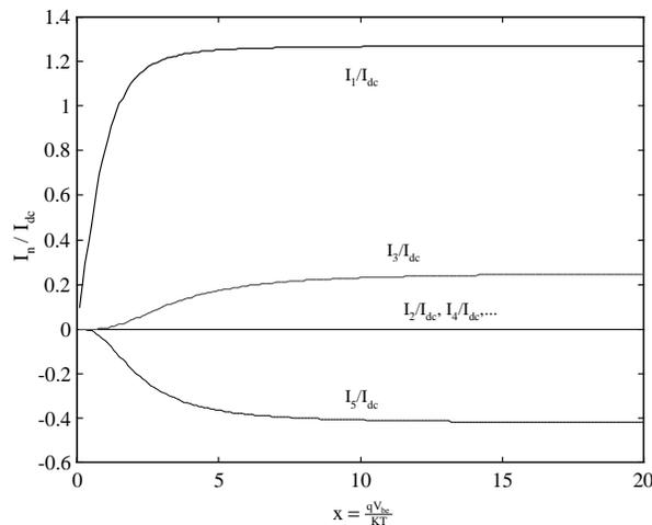
**Figure 5.9. First five orders of collector current components vs. drive level[17].**
