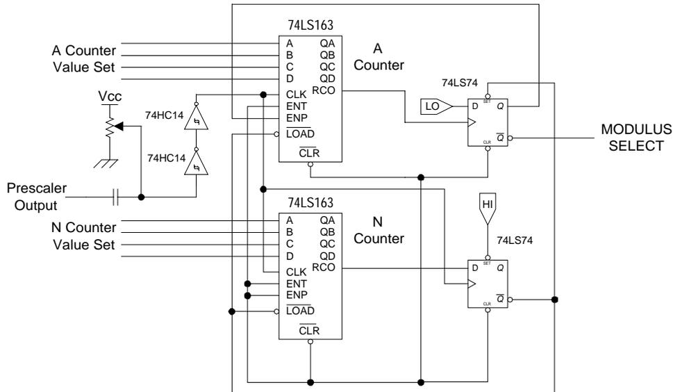
**Figure 7.5. Schematic of TTL realization of Fractional-N counters.**
