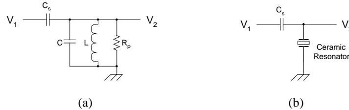
**Figure 3.5. Typical phase shift network implementations.**
