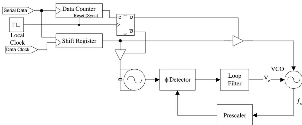
**Figure 4.9. Digital wideband modulation conceptualization.**
