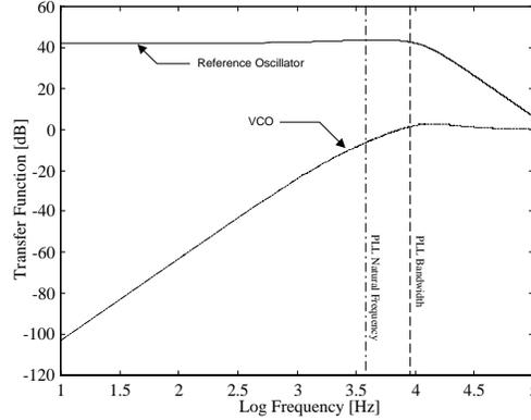
**Figure 6.7. Transfer functions for VCO and reference oscillator phase noise.**
