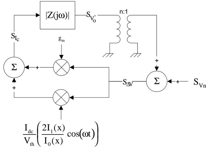
**Figure 5.23. Block diagram of noise in nonlinear oscillator circuit.**
