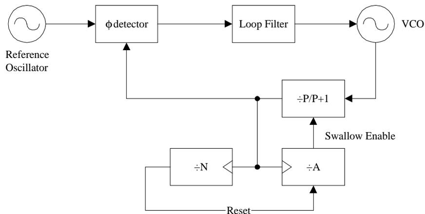
**Figure 7.4. Block diagram of the simple fractional-N synthesis method.**
