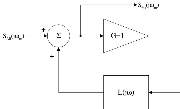
**Figure 5.22. Illustration of Leeson's oscillator model.**
