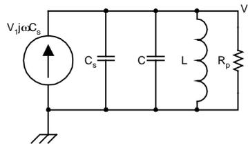
**Figure 3.6. Norton equivalent representation of Fig. 3.5a.**
