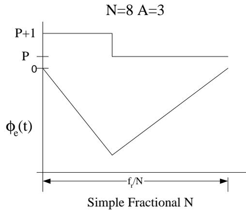
**Figure 7.11. Illustration of phase error and prescaler value for simple fractional-N technique.**
