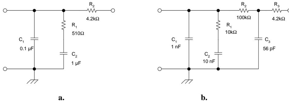
**Figure 7.6. Illustration of loop filters for (a) 460 Hz PLL bandwidth and (b) 9 kHz PLL bandwidth.**
