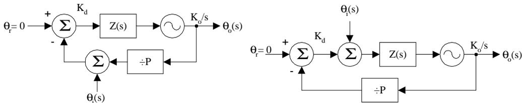
**Figure 6.6. Prescaler and phase detector noise sources.**
