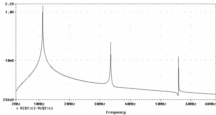
**Figure 5.13a. Differential voltage between collectors of non-saturating balanced pair oscillator.**
