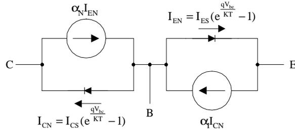
**Figure 5.4. Ebers-Moll model of an NPN transistor.**
