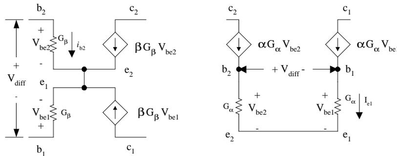
**Figure 5.10. Equivalent representations of the differential pair.**
