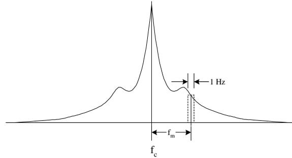
**Figure 6.1. Illustration of carrier with phase noise.**
