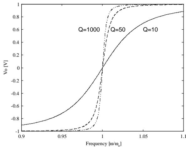
**Figure 3.7. Quadrature detector output voltage vs. frequency characteristic for different parallel phase shift network  $Q$  values.**
