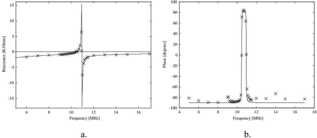
**Figure 3.9. Reactance (a) and phase shift (b) characteristics of the ceramic discriminator.**
