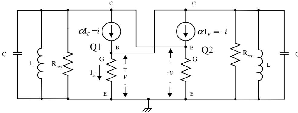
**Figure 5.15. AC equivalent circuit of saturating balanced pair oscillator.**
