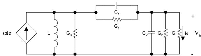
**Figure 5.5. Equivalent circuit of the Colpitts oscillator.**
