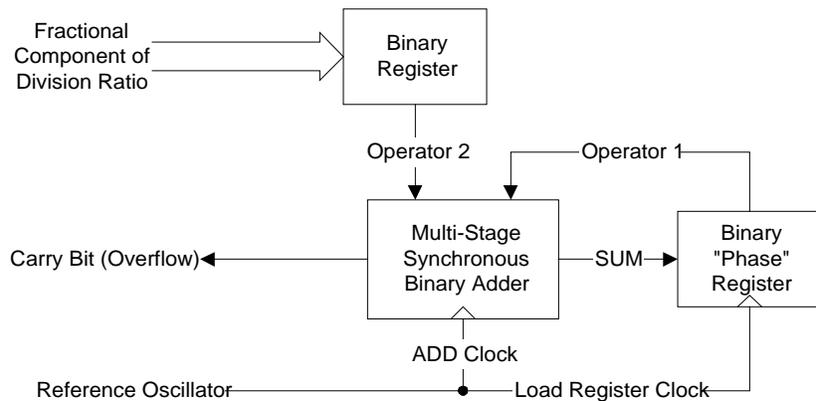
**Figure 7.3. Conceptual drawing of accumulator block.**
