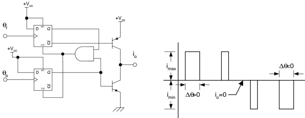
**Figure A.2. (a) Phase-Frequency detector block diagram and (b) output waveform.**
