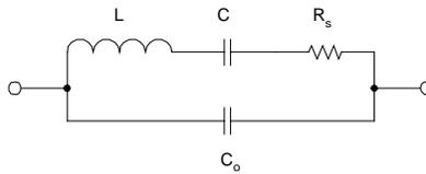
**Figure 5.17. Equivalent Circuit of quartz crystal near fundamental resonance.**
