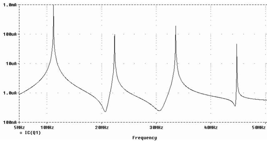
**Figure 5.13b. Collector current of one transistor of non-saturating balanced pair oscillator.**
