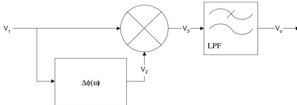
**Figure 3.4. Diagram of quadrature detector composed of mixer, low pass filter, and phasing circuit.**
