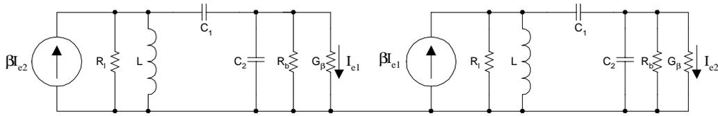
**Figure 5.12 Beta model equivalent circuit of balanced oscillator.**
