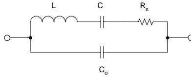
**Figure 3.8. Model of quartz crystal near fundamental resonance.**
