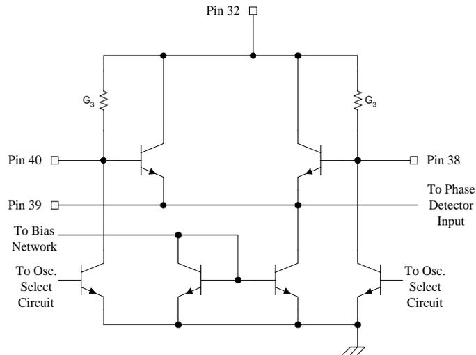
**Figure 5.3. Most likely reference oscillator bias interconnections.**
