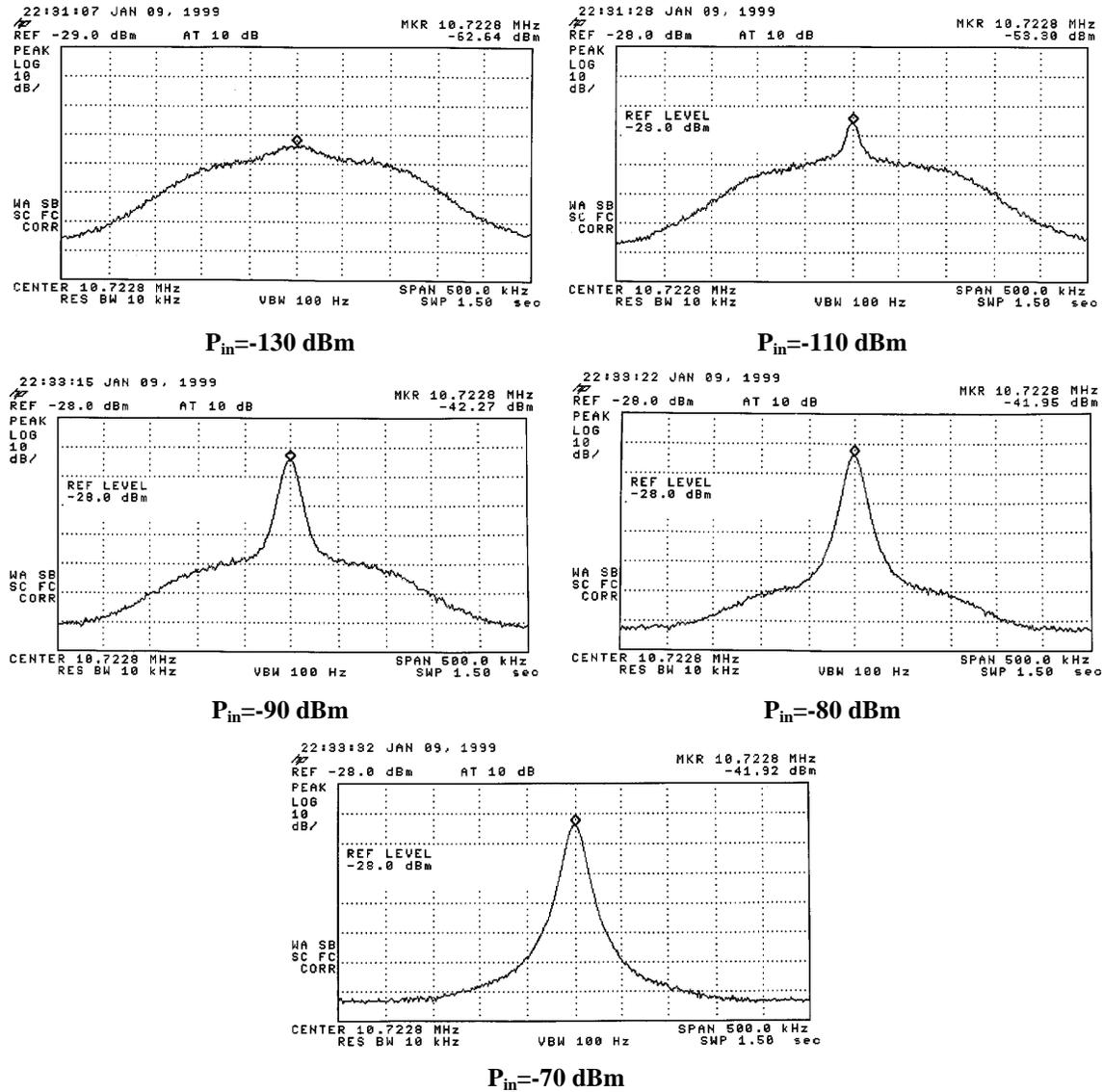
Figure 3.3 IF amplifier limiting effect on noise floor, measured at the IF output for various input carrier levels, vertical scale 10 dB / div with a maximum of -28 dBm, horizontal scale 50 kHz / div.
