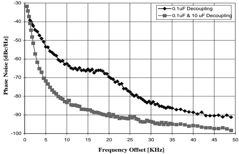
**Figure 7.14. Effect of power supply filtering on output SSB phase noise.**
