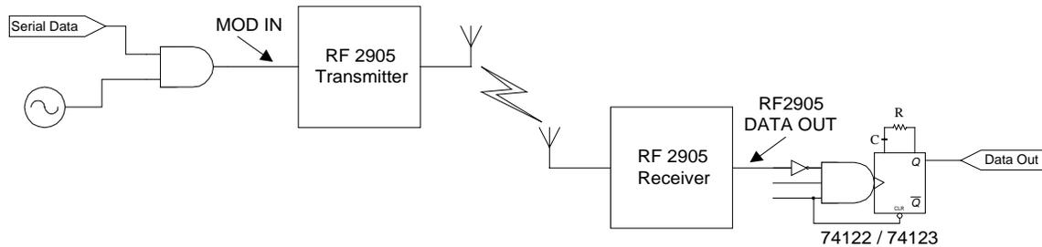
**Figure 4.7. Illustration of digital data modulation.**
