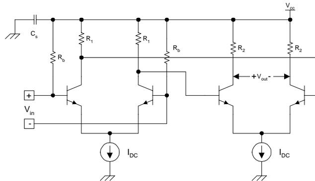
Figure 3.2. Representation of one possible IF amplifier circuit typology.
