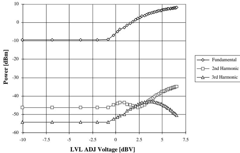
**Figure 4.2. Harmonic content of the output signal vs. LVL ADJ voltage**
