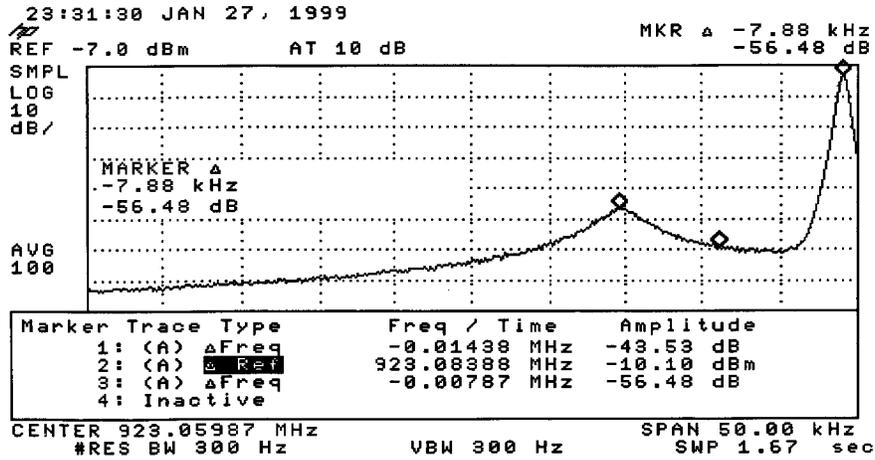
Figure 6.9. Illustration of phase noise peaking due to high loop filter resistor value.
