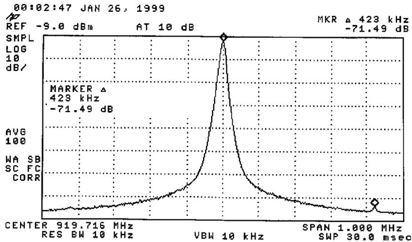
Figure 7.7. Output spectrum of implementation circuit with PLL bandwidth of 460 Hz.
