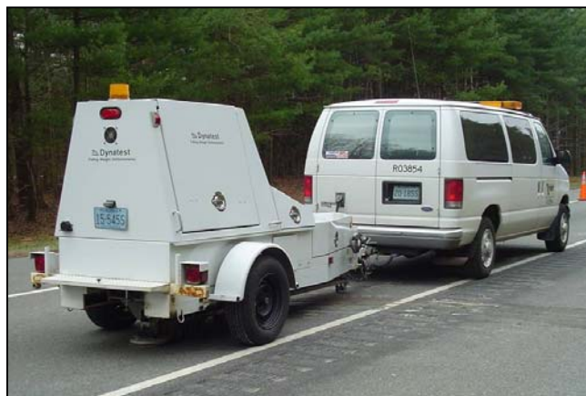
Figure 13. FWD Used by VDOT
