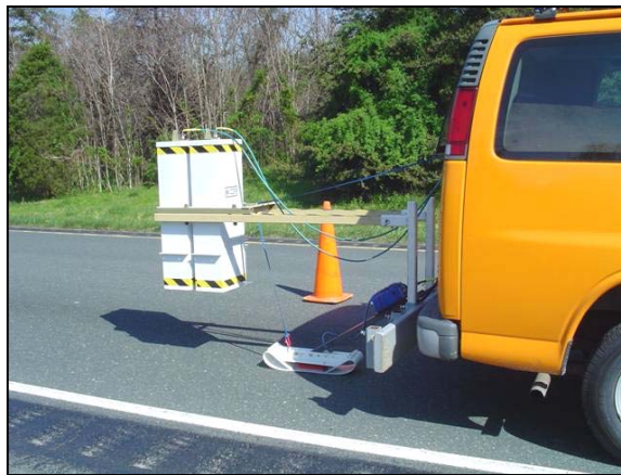
Figure 11. Antenna Used for GPR Collection
