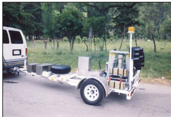
Figure 6. FWD – Dynatest Model 8002
