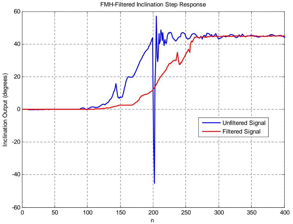
Figure 4.24: Filtered inclination step response with FMH(73) sampled at 500 Hz.
