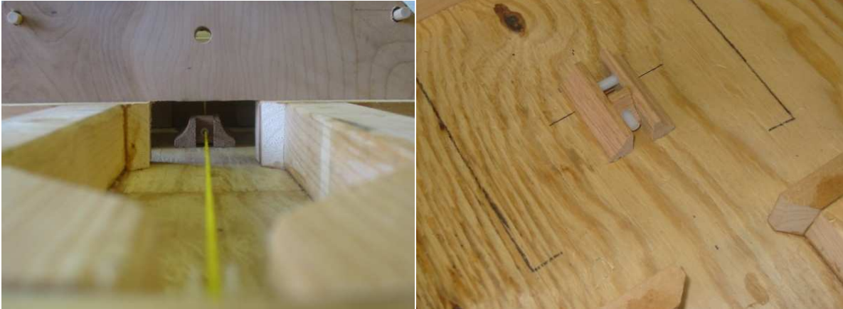
Figure 3.17: Pulley/wire guide combination (left) and wire guide without tilt platform (right).
