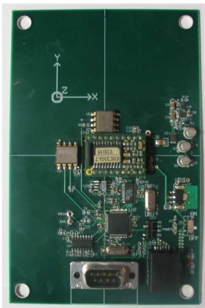
Figure 3.11: Magnetometer/inclinometer circuit board.
