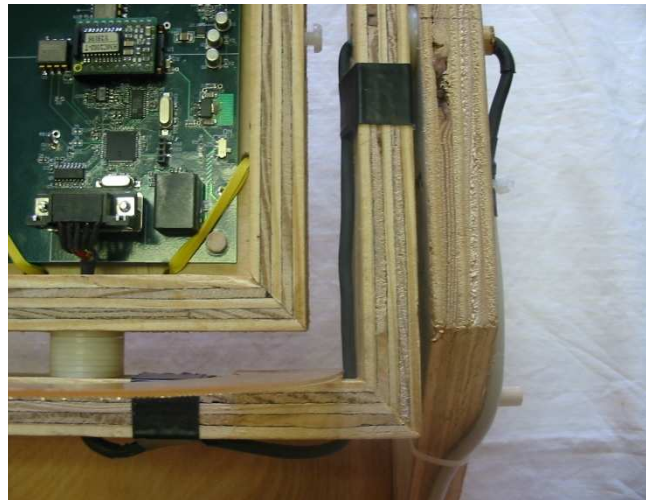
Figure 3.14: System cable routed through pitch and roll axle.
