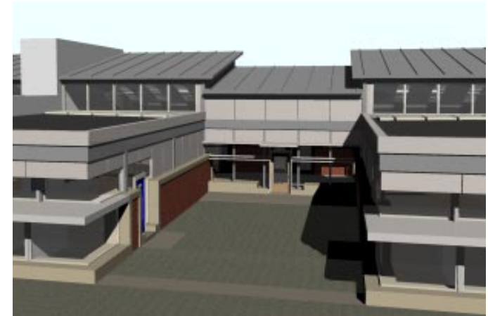
EXTERIOR VIEW OF COURTYARD SHOWING VARYING FENESTRATION. CLERESTORIES AT GRADE PODS. WINDOW WALLS BETWEEN PODS.
