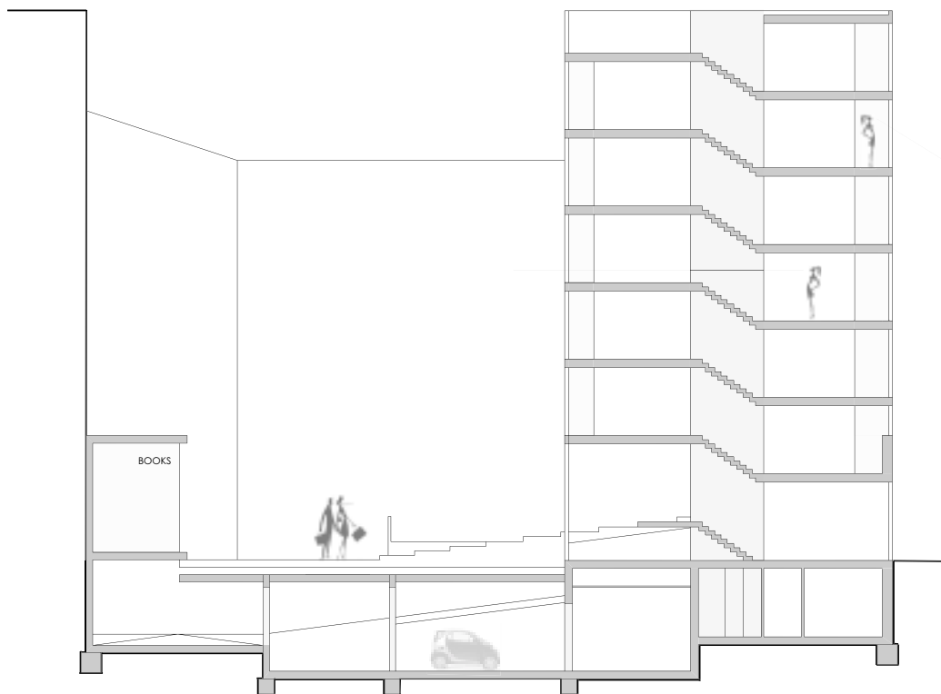
Section A: Volume II -apartment split level and courtyard with underground parking
