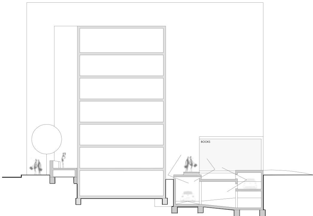
section F: Setback, existing building and courtyard with underground parking
