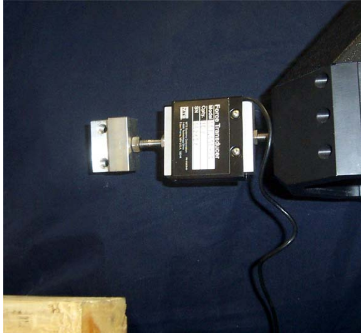
Figure 3.2: Clamp Used to Connect Load Cell to Tape End
