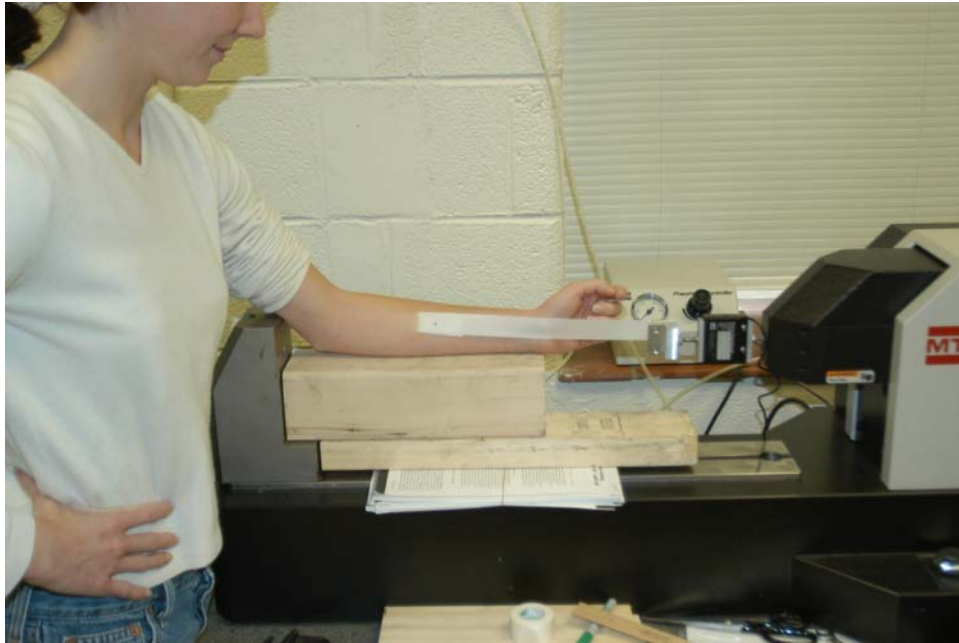
Figure 3.3: Experimental Setup Including Subject with MTS Tytron 250 Testing Machine
