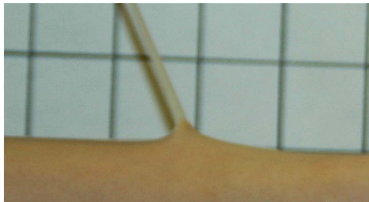
Figure 1.3: Photograph of Peeling at About 120 degrees
