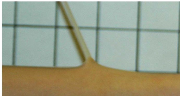
Figure 6.14: Peeling at Approximately 120 degrees
