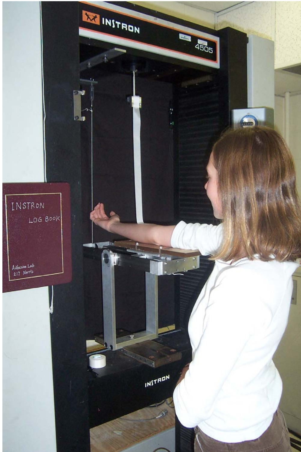
Figure 2.4: Experimental Setup for 90-degree Tests Including Subject with Instron 4505 Testing Machine
