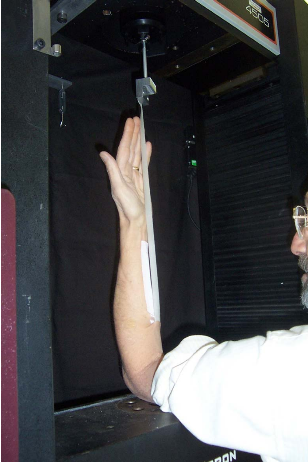
Figure 2.5: Experimental Setup for 180-degree Tests Including Subject with Instron 4505 Testing Machine
