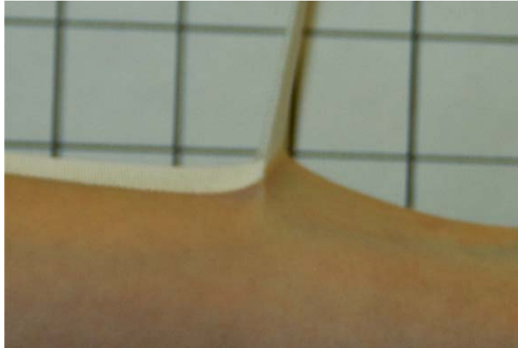
Figure 1.2: Photograph of Peeling at About 90 degrees
