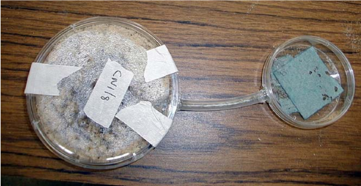
Figure 3-1. The No-choice subterranean termite arena. Termites were placed in the larger housing chamber where they could forage through a Tygon tube into a smaller diet chamber. The diet chamber contained dyed and/or hexaflumuron-treated paper towels.
