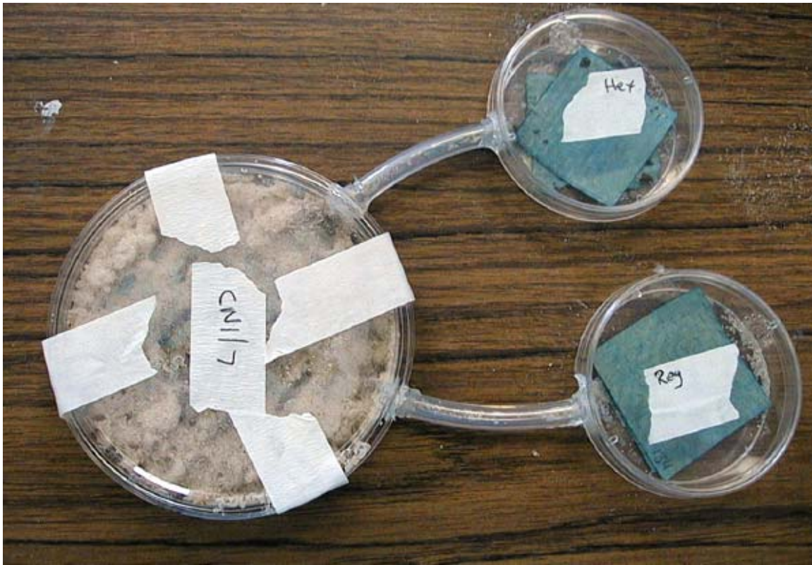
Figure 3-2. The Choice subterranean termite arena. Termites were placed in the larger housing chamber where they could forage through two different Tygon tubes into either of the smaller diet chambers. One diet chamber contained dyed paper towels as the control, and the second diet chamber contained dyed hexaflumuron-treated paper towels.
