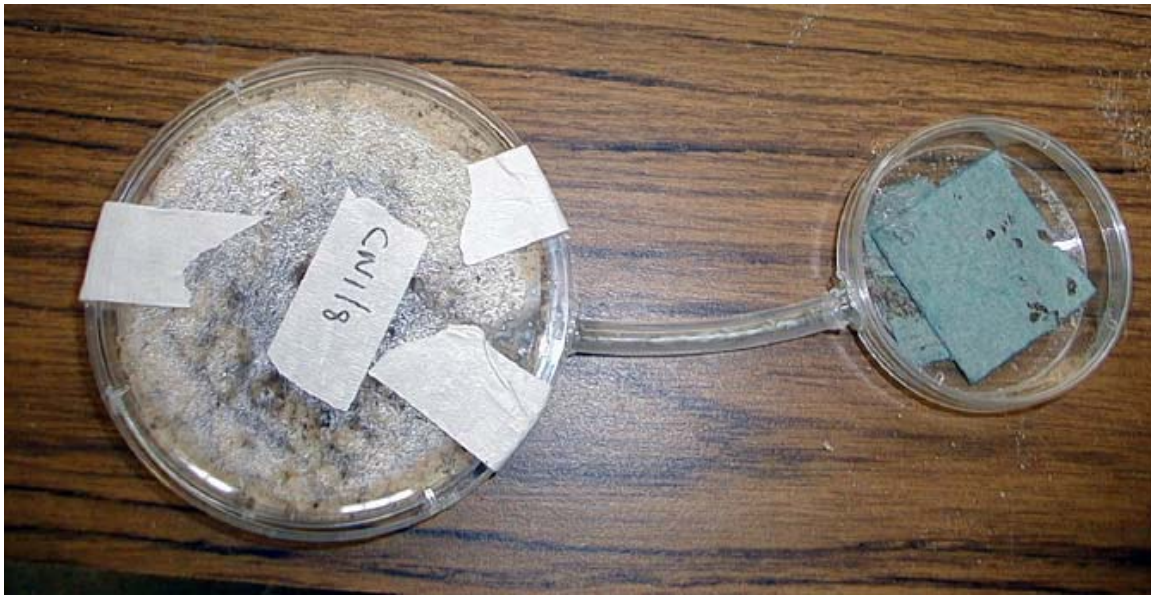
Figure 4-1. The No-choice subterranean termite arena. Termites were placed in the larger housing chamber where they could forage through a Tygon tube into a diet chamber. The diet chamber contained dyed and/or hexaflumuron treated paper towels.
