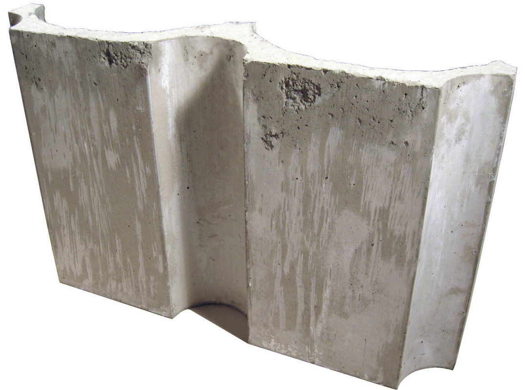
Full scale form work used to cast prototype concrete panel.
