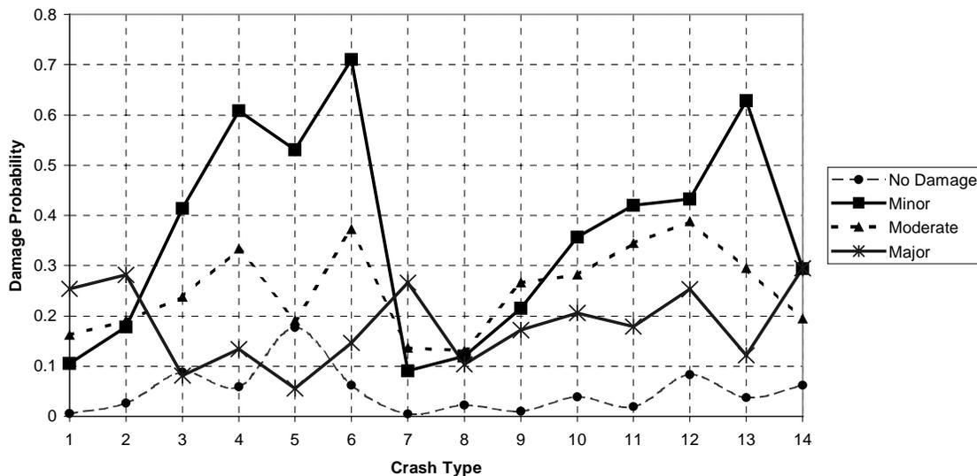
**Figure 5-1 Damage probability per crash type**
