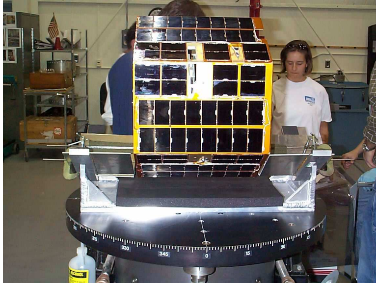
Figure 5.36: Mass Properties Testing Configuration
