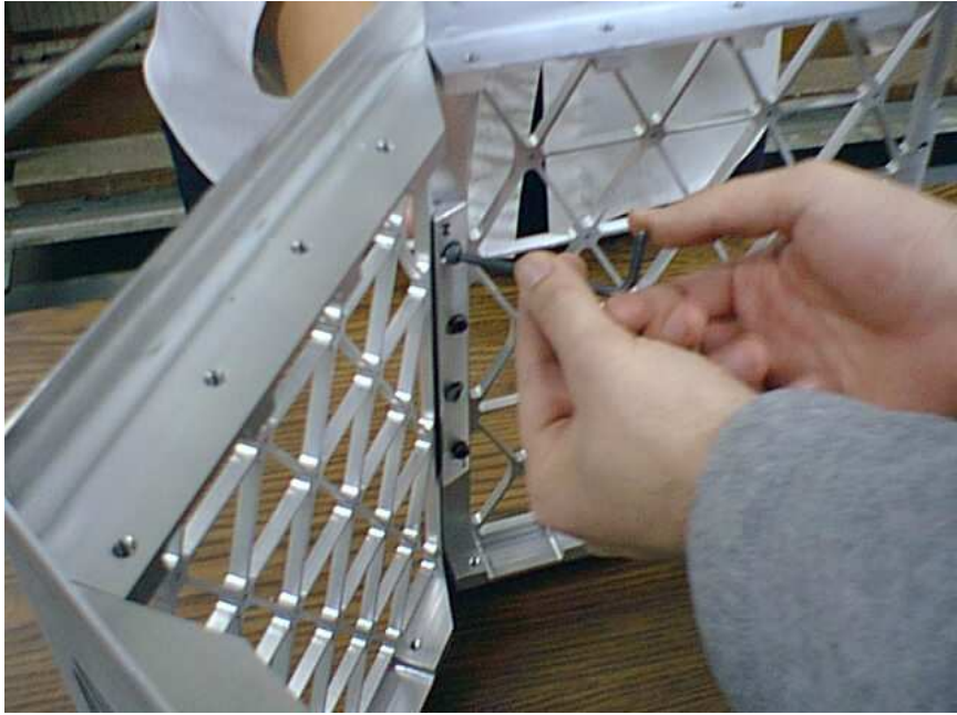
Figure 3.8: Side Panel Assembly (Bracket Design 1)
