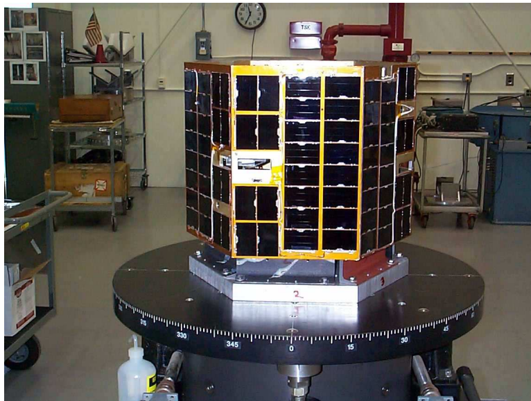
Figure 5.37: Mass Properties Testing Configuration
