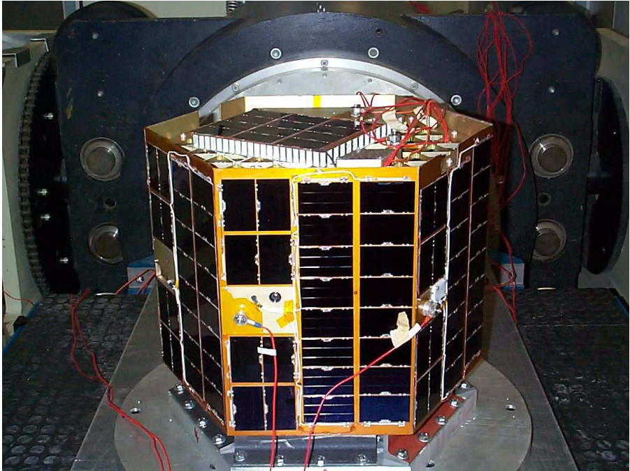
Figure 5.30: Flight Dynamic Testing Accelerometer Configuration
