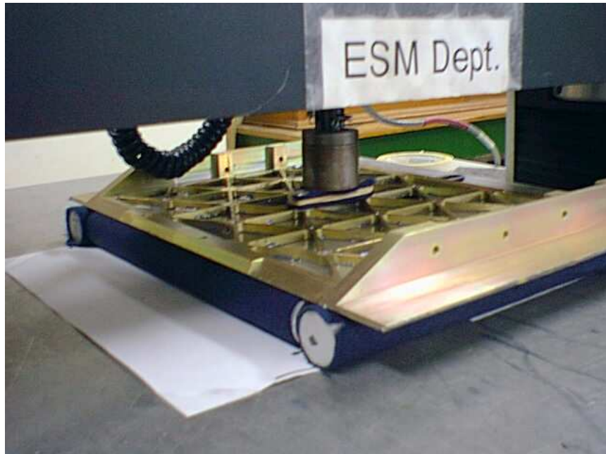
Figure 5.21: Composite Side Panel Static Test Configuration
