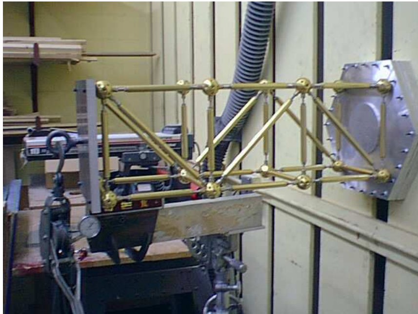
Figure 5.39: Truss Fixture Testing Configuration
