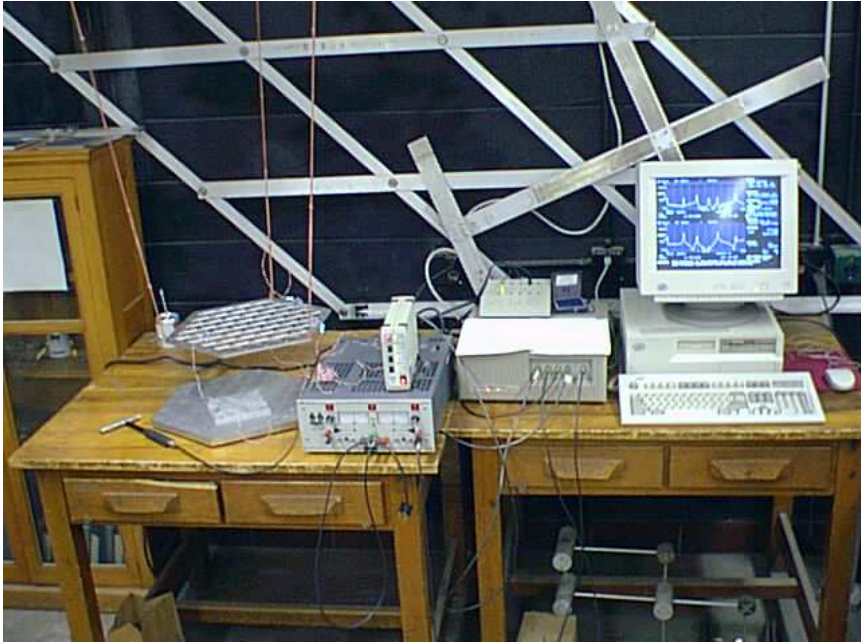
Figure 5.8: End Panel Modal Test Configuration
