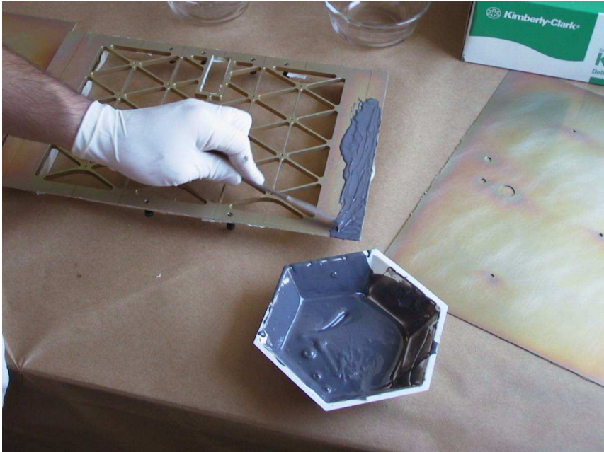
Figure 4.3: Application of the Epoxy to Isogrid Panel
