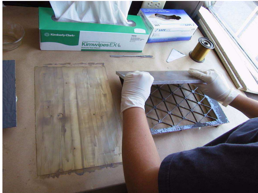
Figure 4.4: Spatula Method Used to Ensure Even Epoxy Distribution
