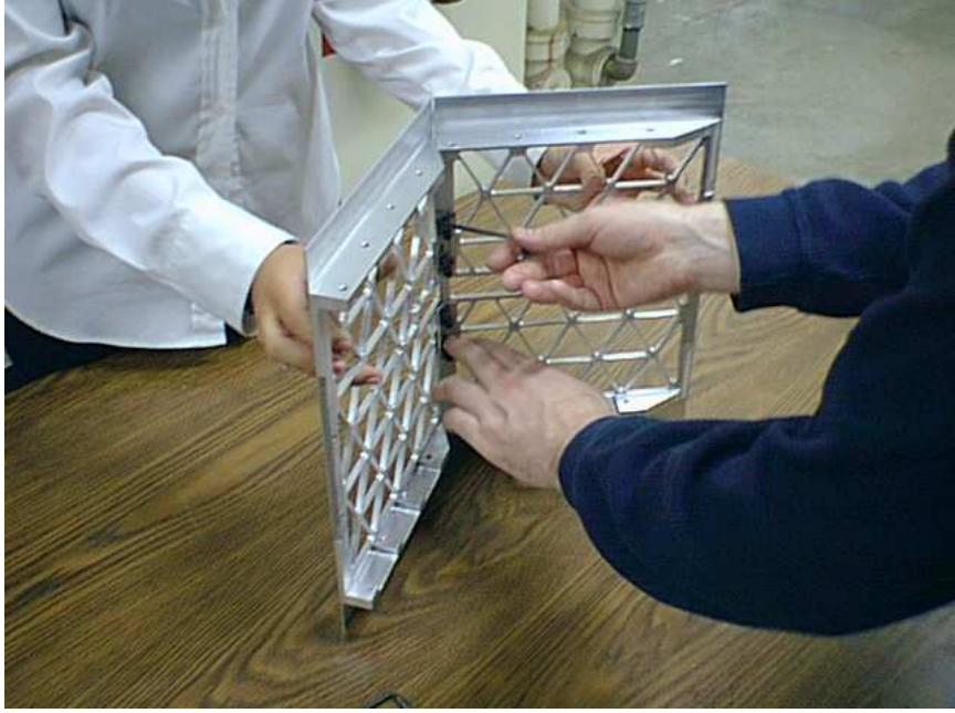
Figure 3.9: Side Panel Assembly (Bracket Design 2)
