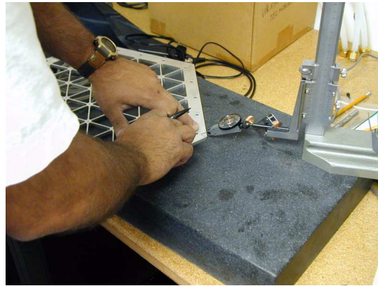
Figure 4.1: Method Used to Verify Lightband Flatness Requirements
