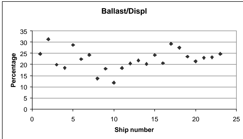
Figure 6.1: Ballast / displacement from several ship data
