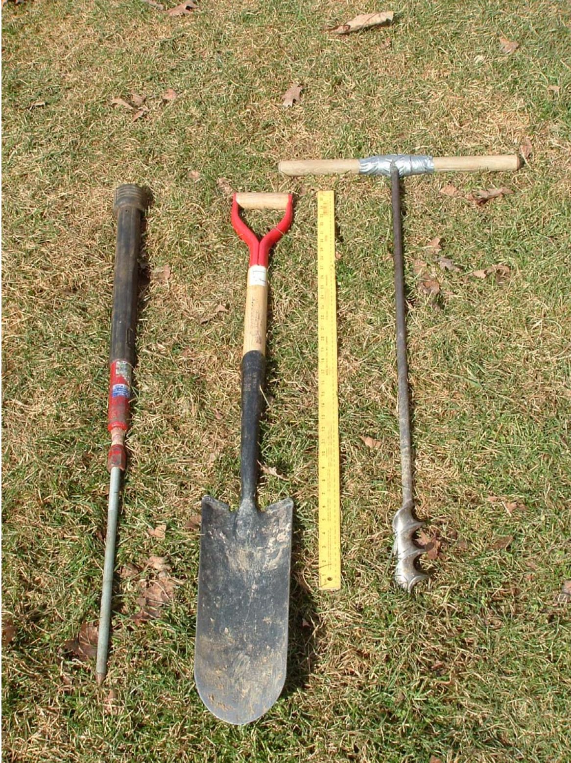
Figure III-1. Tools used to estimate bulk density measured by the excavation method on mine soils in the Appalachian region. From left to right: A slide hammer with a tapered tip (constructed by sharpening a carriage bolt), a sharpshooter, a meter stick for scale, and a screw auger.
