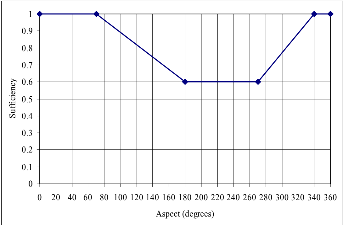
Figure V-9. Sufficiency curve for aspect used on mine soils in the Appalachian region, based on research by Hicks and Frank, 1984 and Burger et al., 2002.
