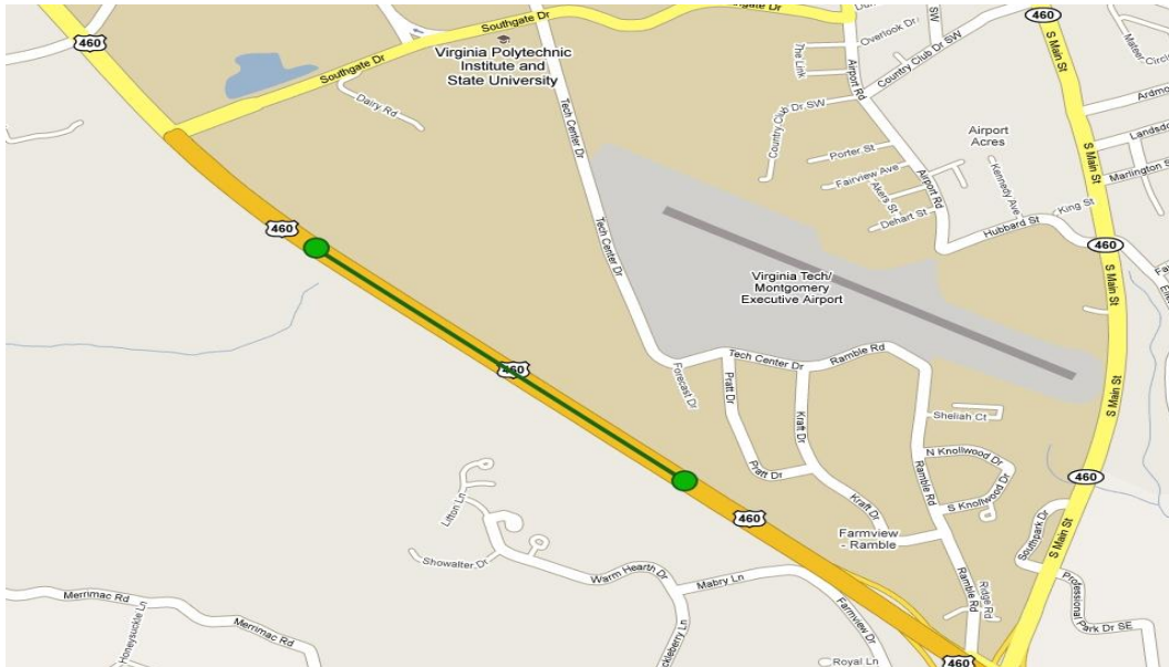
Figure 6: Example of a two lane road straight road segment with GPS points
