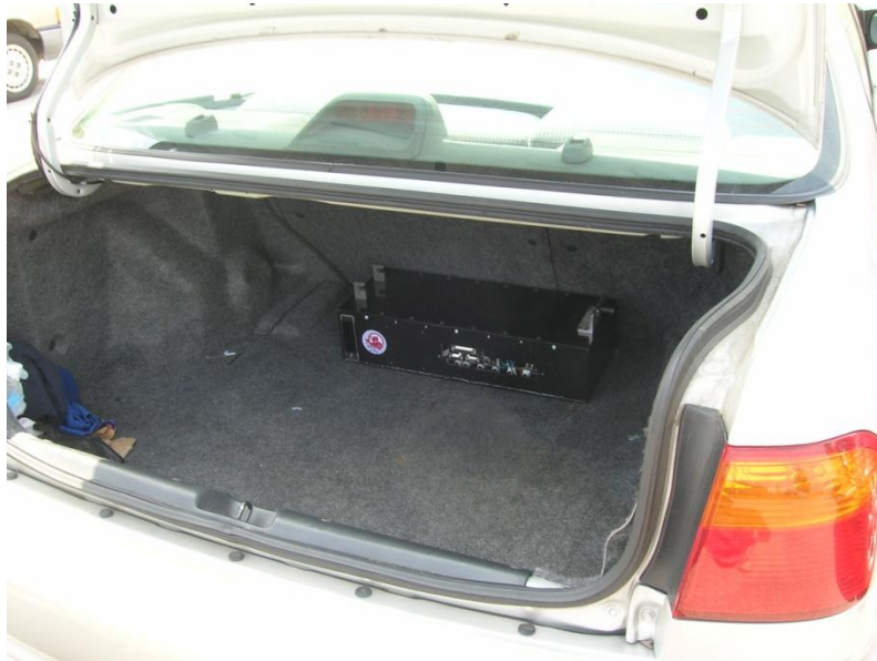
Figure 1: Data Acquisition System mounted under the package shelf in the trunk of a vehicle
