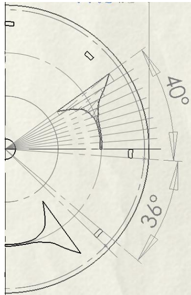
Figure 4.8 Close-up of orifice area profile, including construction line sketch, fourth iteration disc design
