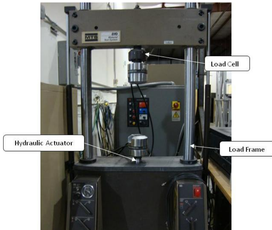
Figure 5.1 MTS load frame used in full scale damper tests
