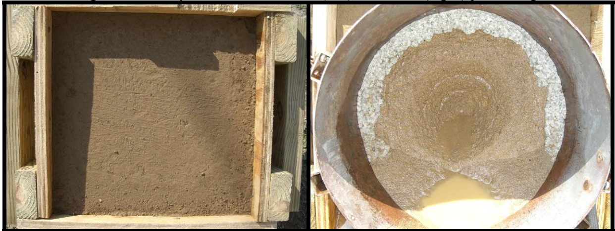
Figure A.4. Clay loam Run 4 before (left) and after (right) jet testing.
