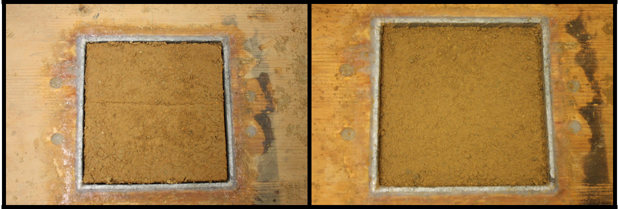
Figure A.33. Clay Run 5 before (left) and after (right) flume testing.
