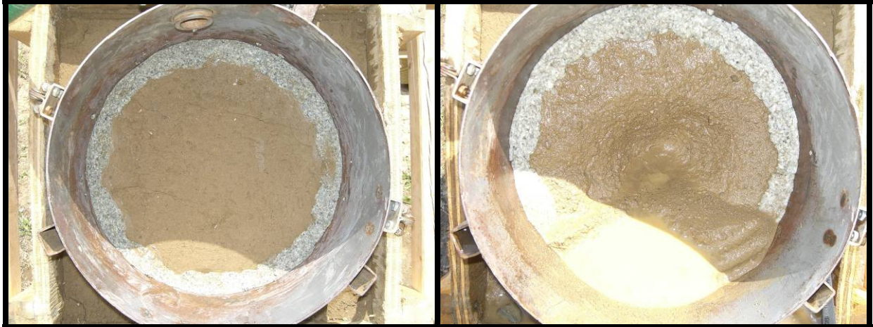
Figure A.9. Clay loam Run 9 before (left) and after (right) jet testing.
