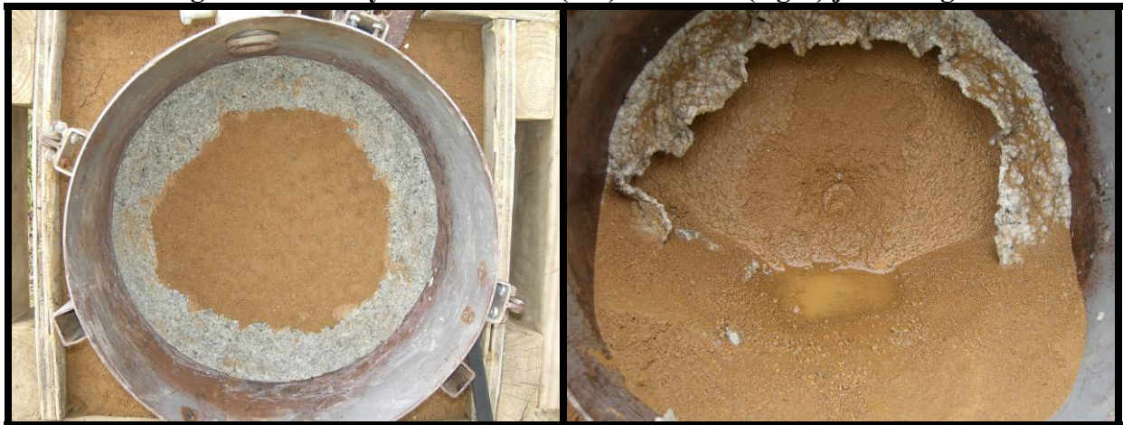
Figure A.19. Clay Run 8 before (left) and after (right) jet testing.
