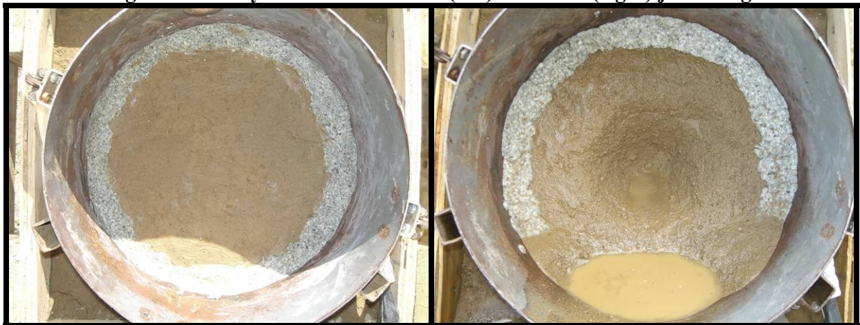
Figure A.8. Clay loam Run 8 before (left) and after (right) jet testing.
