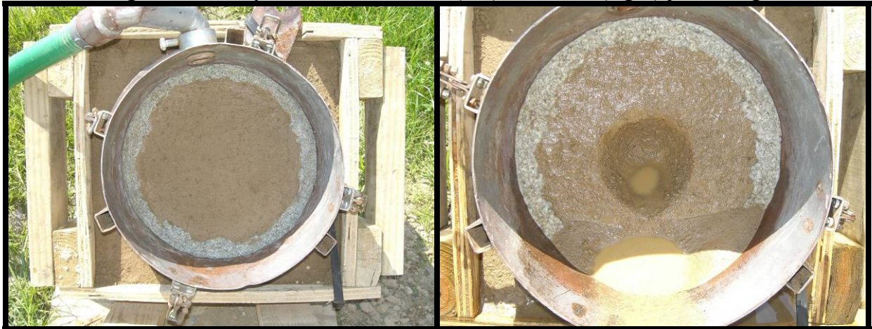
Figure A.10. Clay loam Run 10 before (left) and after (right) jet testing.
