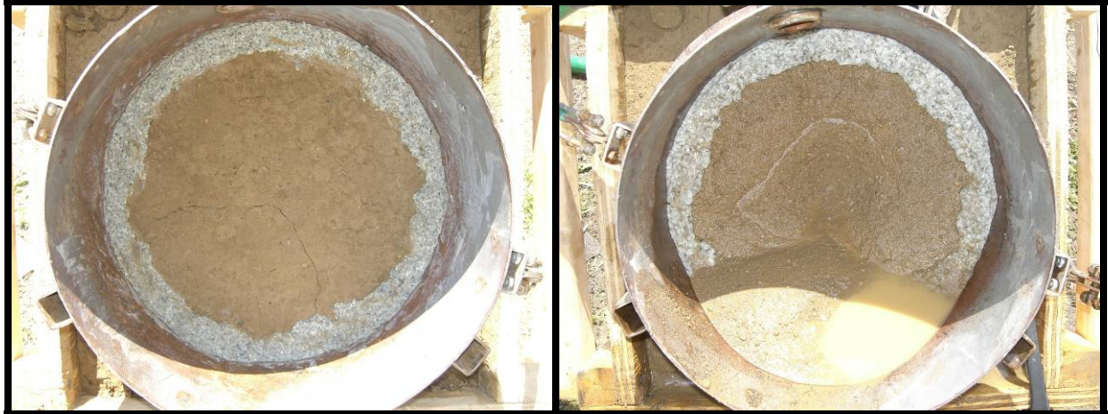
Figure A.3. Clay loam Run 3 before (left) and after (right) jet testing.
