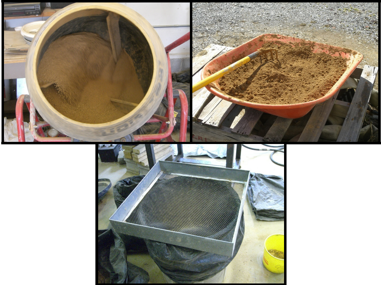
Figure 3.1. Clay preparation consisted of mixing (top left), wetting (top right), and sieving (bottom).
