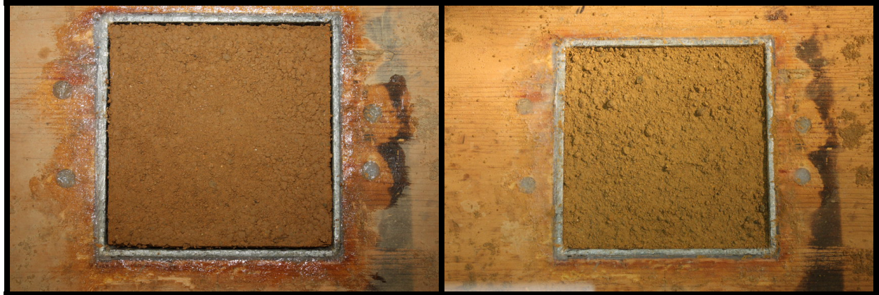
Figure A.30. Clay Run 2 before (left) and after (right) flume testing.
