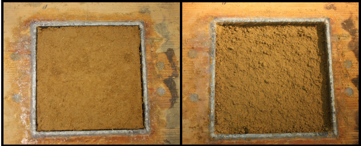
Figure 4.15. Before (left) and after (right) flume testing for clay Run 3.
