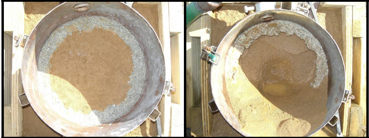
Figure A.15. Clay Run 4 before (left) and after (right) jet testing.
