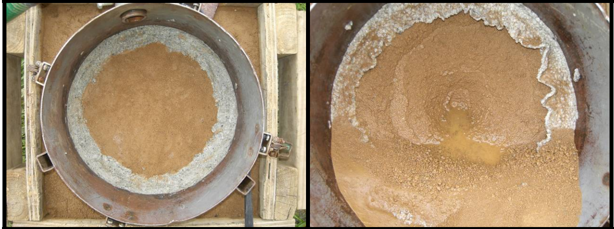
Figure A.21. Clay Run 10 before (left) and after (right) jet testing.
