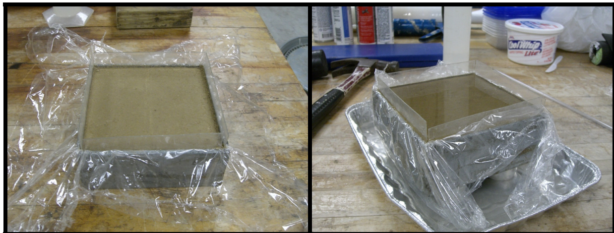
Figure 3.8. Remolded clay loam before (left) and during (right) wetting.
