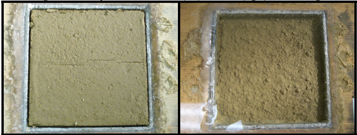
Figure A.28. Clay loam Run 7 before (left) and after (right) flume testing.
