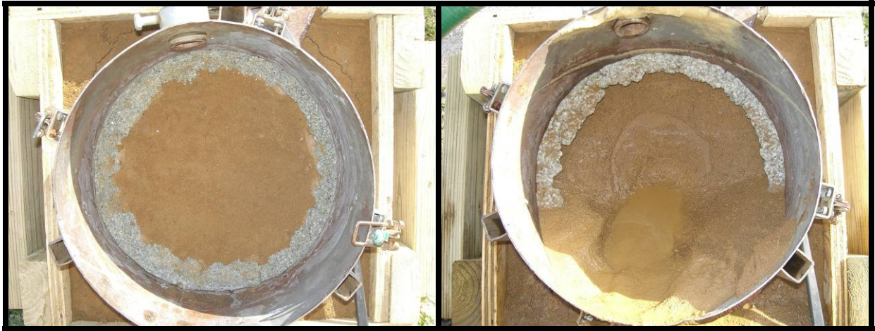
Figure A.12. Clay Run 1 before (left) and after (right) jet testing.
