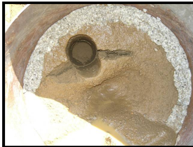
Figure 3.4. Bulk density sample inside base ring after clay jet test.
