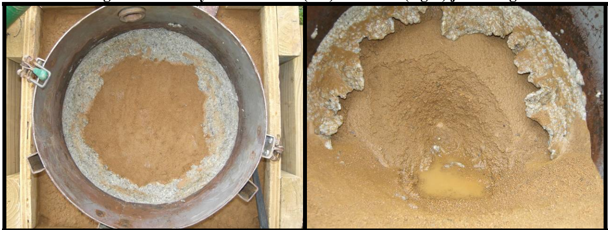
Figure A.20. Clay Run 9 before (left) and after (right) jet testing.
