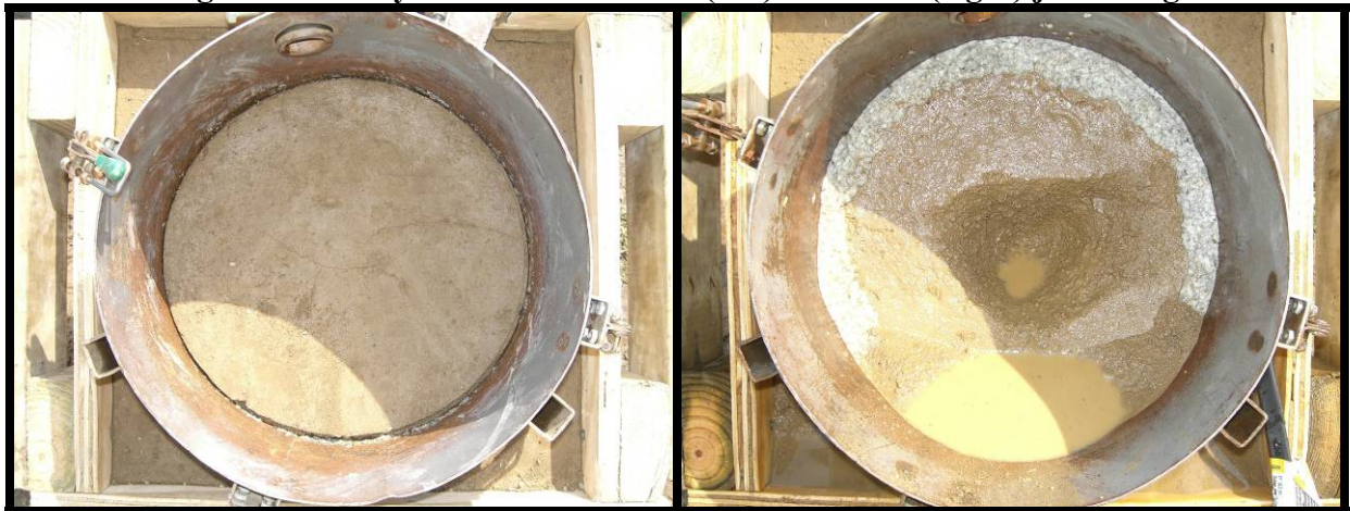
Figure A.7. Clay loam Run 7 before (left) and after (right) jet testing.
