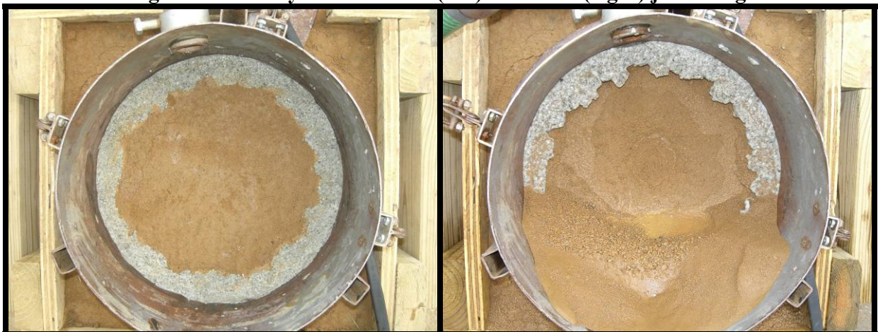
Figure A.14. Clay Run 3 before (left) and after (right) jet testing.
