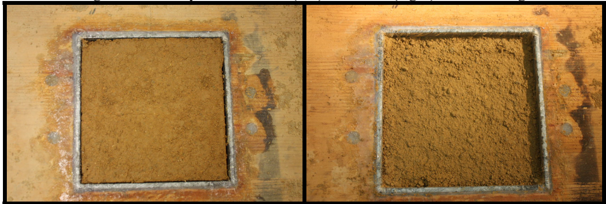
Figure A.31. Clay Run 3 before (left) and after (right) flume testing.
