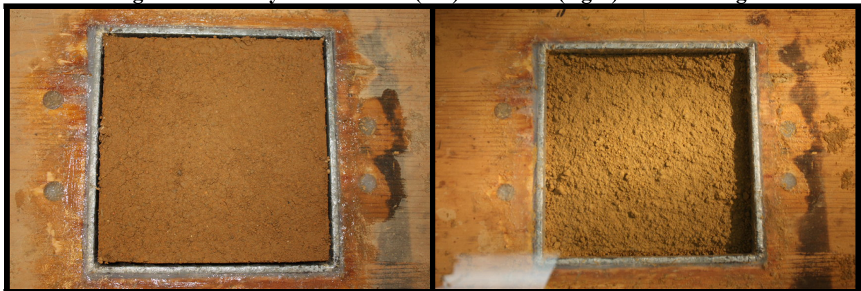
Figure A.32. Clay Run 4 before (left) and after (right) flume testing.
