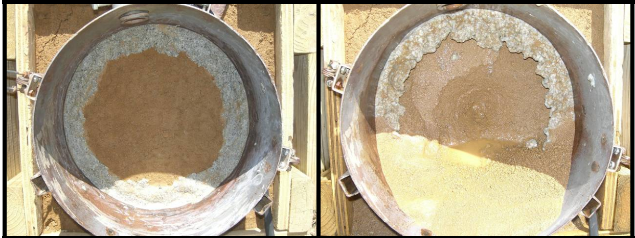
Figure A.18. Clay Run 7 before (left) and after (right) jet testing.
