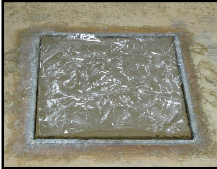
Figure 3.10. Clay loam box sealed in flume bed.
