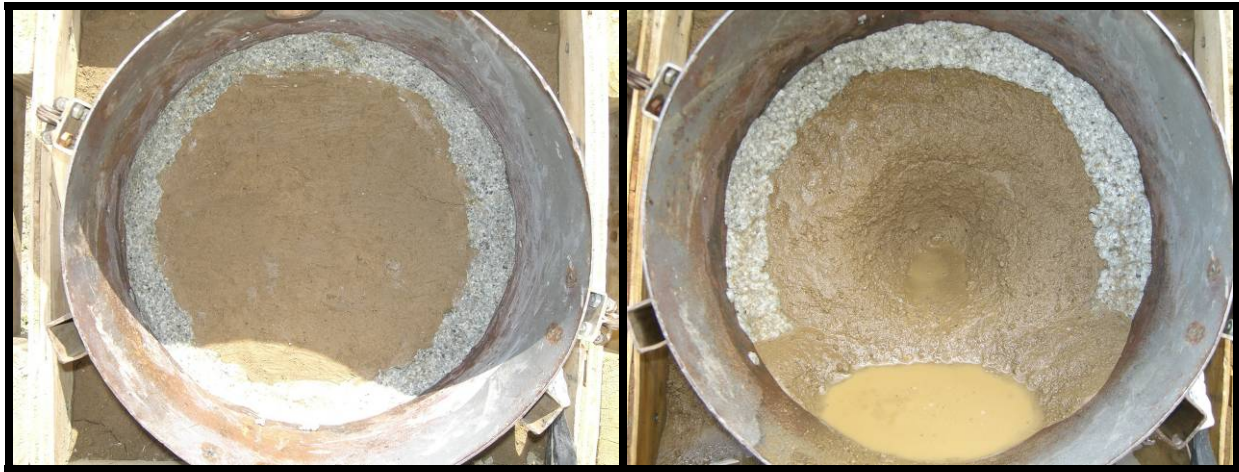
Figure 4.2. Clay loam Run 8 before (left) and after (right) testing.
