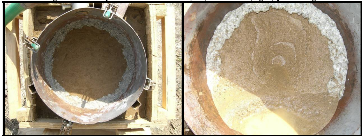
Figure A.2. Clay loam Run 2 before (left) and after (right) jet testing.
