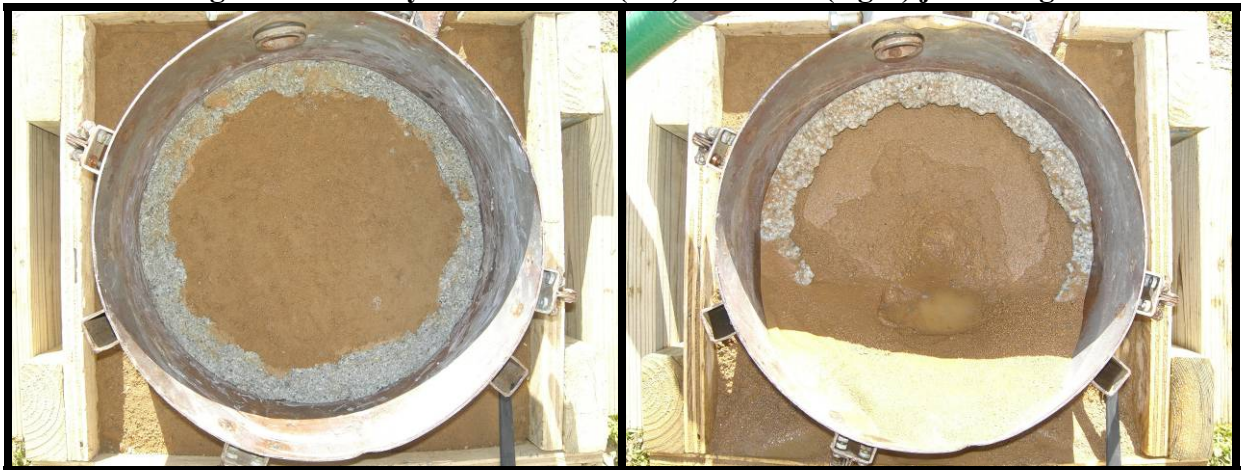
Figure A.13. Clay Run 2 before (left) and after (right) jet testing.
