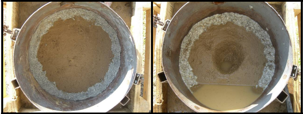
Figure A.1. Clay loam Run 1 before (left) and after (right) jet testing.
