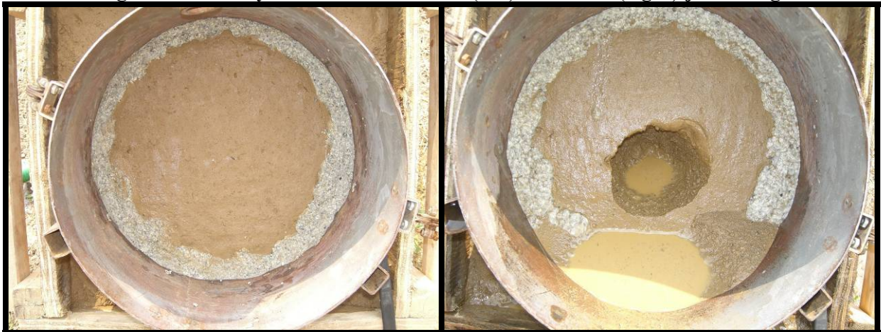
Figure A.11. Clay loam Run 11 before (left) and after (right) jet testing.
