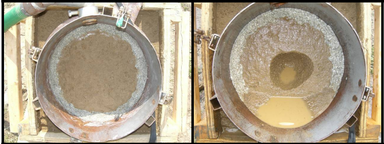
Figure A.6. Clay loam Run 6 before (left) and after (right) jet testing.
