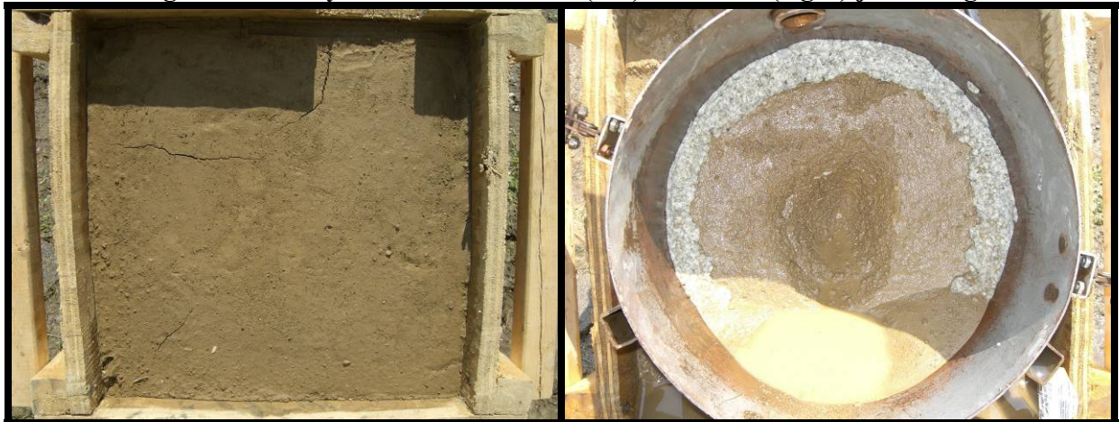
Figure A.5. Clay loam Run 5 before (left) and after (right) jet testing.
