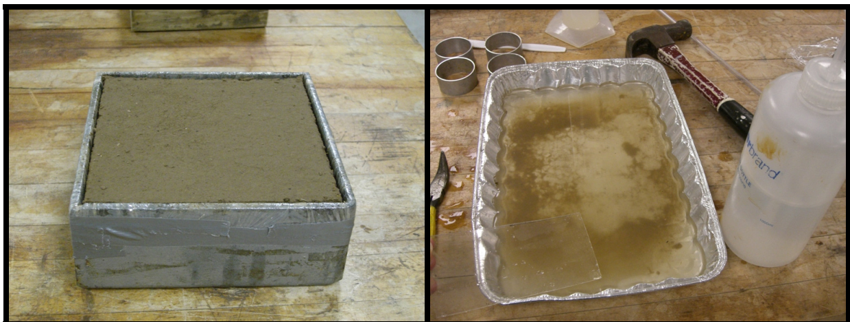
Figure 3.9. Clay loam box after removal of acrylic spacers (left) and after rinsing acrylic spacers (right).
