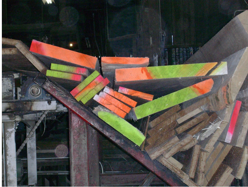
Figure 3.2. Lumber paint indicates different quadrants from which a board originated relative to the major and minor axes of each log
