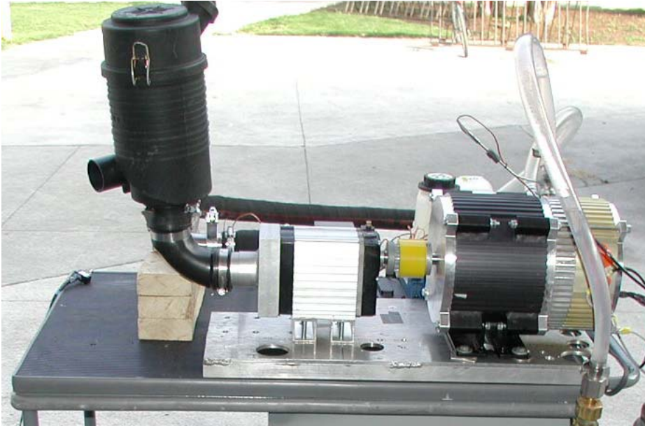
Figure 4: Motor-inverter unit coupled to the air compressor
