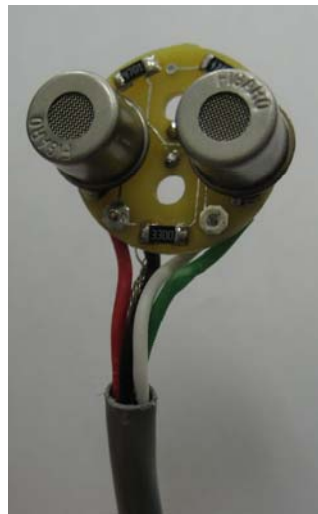
Figure 4-6. Ethanol Vapor Sensors on PCB
