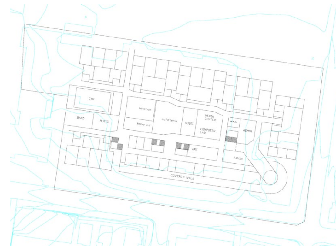
First attempt at space planning for the school. This had the grades along the perimeter, with all offices and specialty rooms near the center. This plan used controlled circulation throughout the building.
