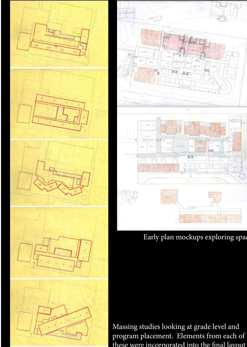
The next reworking rotated the 2nd and 3rd grades 15 and 30 degrees respectively. It also retooled the entry and main stair, as well as adding the new commons area and front curves (see following pages)
