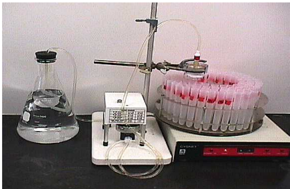
FIGURE 5.1 MISCIBLE DISPLACEMENT SYSTEM USED FOR DESORPTION STUDIES
