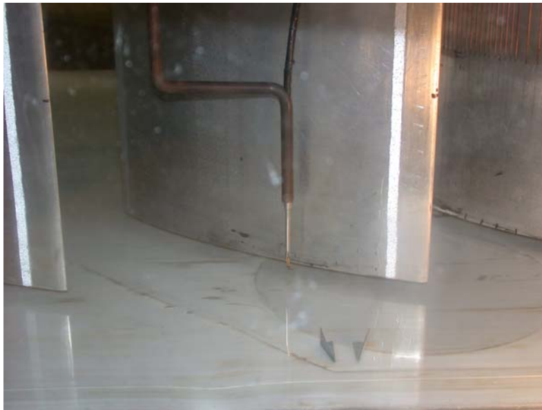
Figure 2.14 Boundary layer probe mounted in probe holder.
