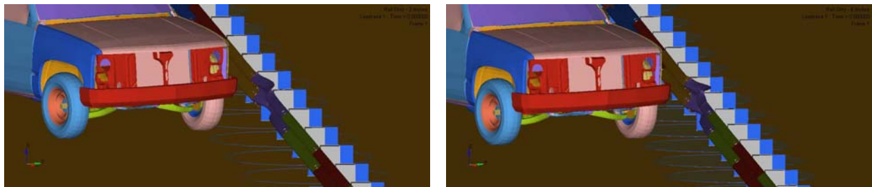
Figure 79: Pre-existing damage for rail deflection only simulations. 3 inches on left, 5.6 inches on right.
