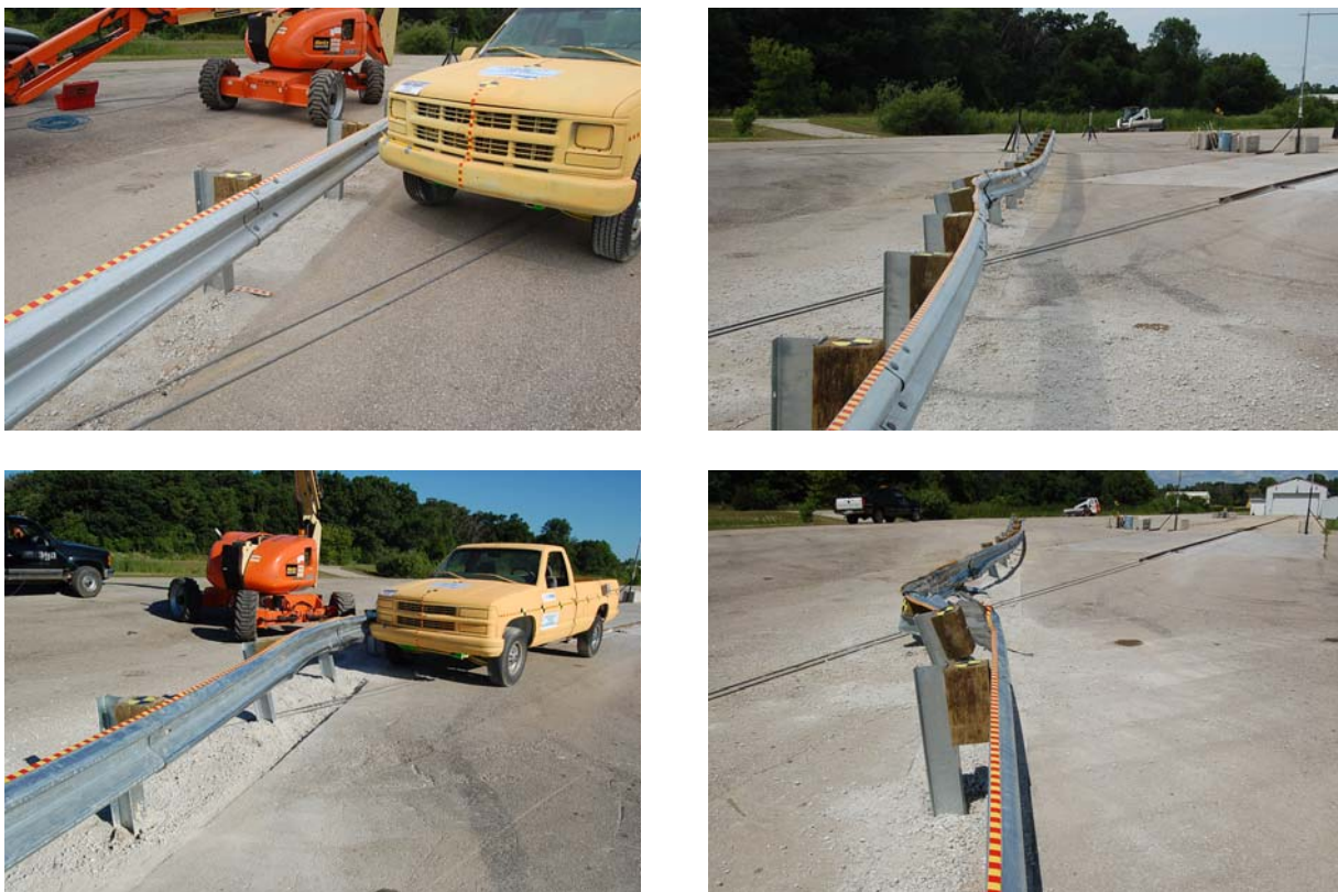
Figure 74: MGA Crash Test C08C3-027.1 after installation (top left) and after the first, low speed impact (top right) [16]. The following day, the guardrail was prepared for MGA Crash Test C08C3-027.2 (bottom left) which resulted in the vehicle vaulting and further damage to the guardrail (bottom right) [17].
