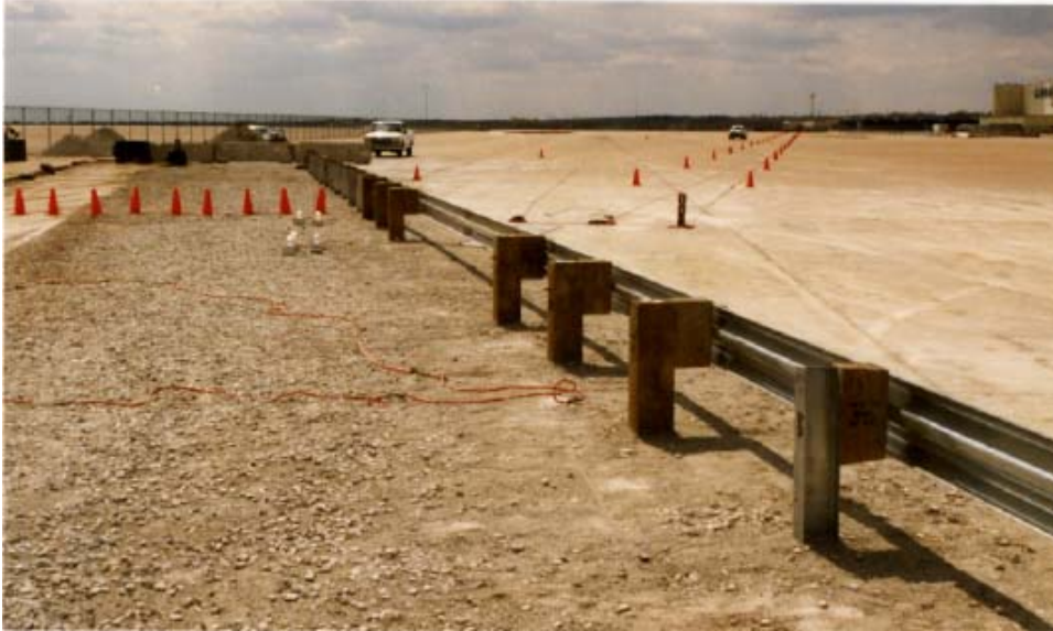
Figure 20: Strong-post w-beam guardrail with nested rail used for UNL crash test
