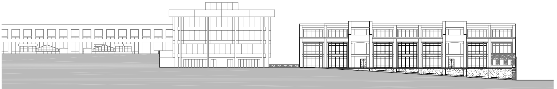
Building Elevation/ Section - Facing West: Cut along the center-line of the Cowgill Hall service road retaining wall, this graphic shows the articulation of the retaining wall, which marks the eastern edge of the newly formed plaza. (Illustration by author)
