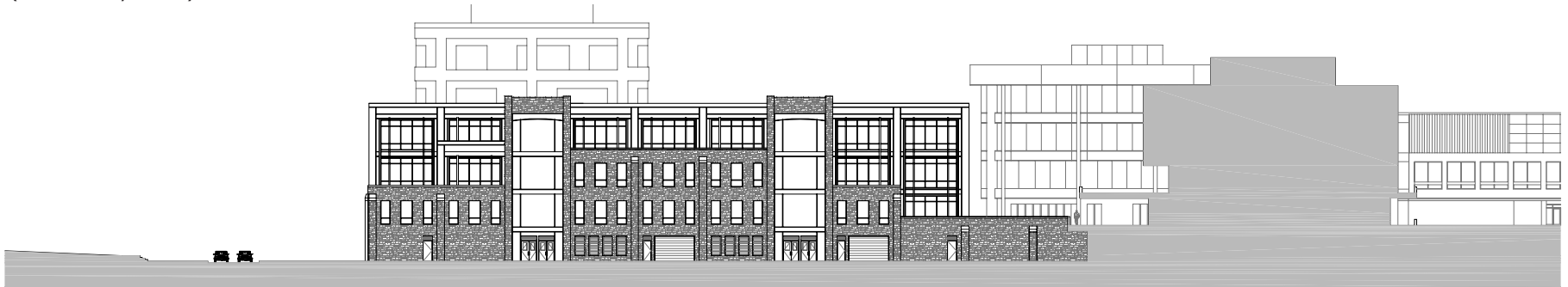
Building Elevation/ Section - Facing East: Cut along through Derring Hall, this graphic shows the west facing elevation of the Architecture Annex. Prominent in this view are the two Hokie-stone frame service cores, which provide vertical access through the building and mechanical riser space. This graphic also shows the Annex retaining wall connection to Derring Hall, thus completing the building edge along Perry Street. (Illustration by author)
