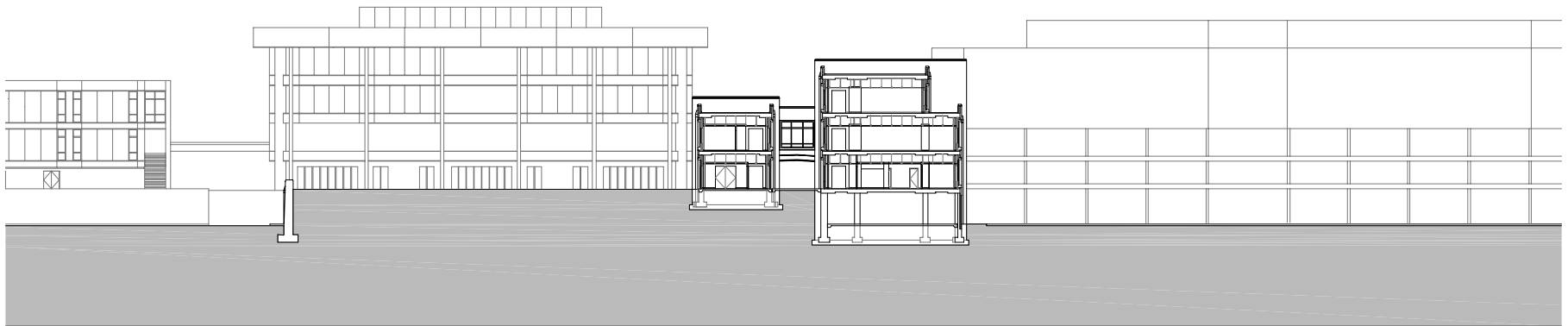
Site Section Elevation - Facing South : Showing the relative position of each floor of the Architecture Annex with respect to the grade changes, this graphic also indicates that the structure of the building is a concrete column and slab configuration. With a floor to floor height of 15', each floor slab is 16" thick and provides a 42" plenum space above the ceilings, which are set at 10'-0" (Illustration by author)
