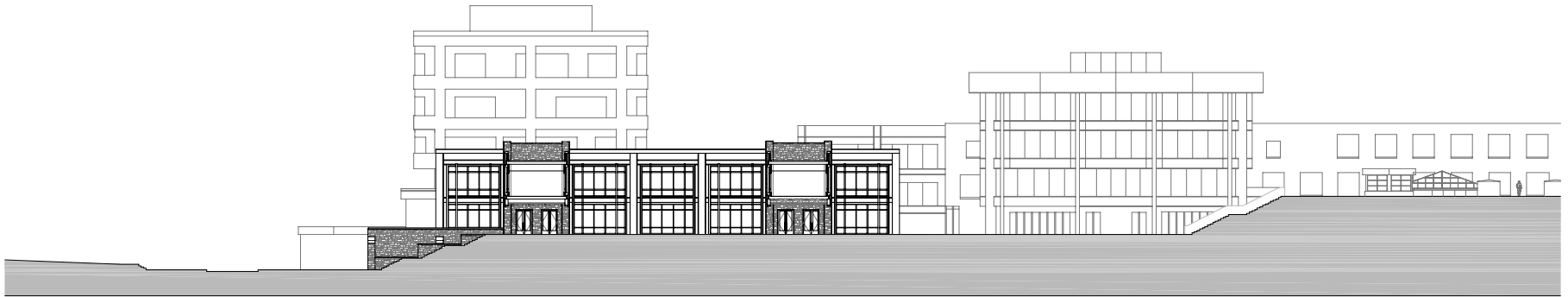
Building Elevation/ Section - Facing East: Cut along the centerline of the building and the minor axis path this graphic shows the system of stairs that negotiate the 30' elevation change from Perry Street to the level of Burchard Plaza. Also visible are the two bridge elements, which connect the two parts of the building, while spanning the axis path and serving as the entry portals into campus (Illustration by author)
