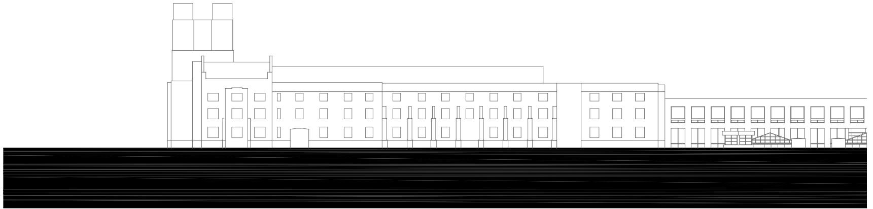
Site Elevation - Facing West: Cutting through Burchard Plaza, and the centerline of the axis path, this section clearly shows the elevation changes that are addressed on campus at this site. Looking towards the main building of the Architecture Annex this drawing also shows the location of the portal bridging and the articulation of the facade that overlooks the axis path. (Illustration by author)
