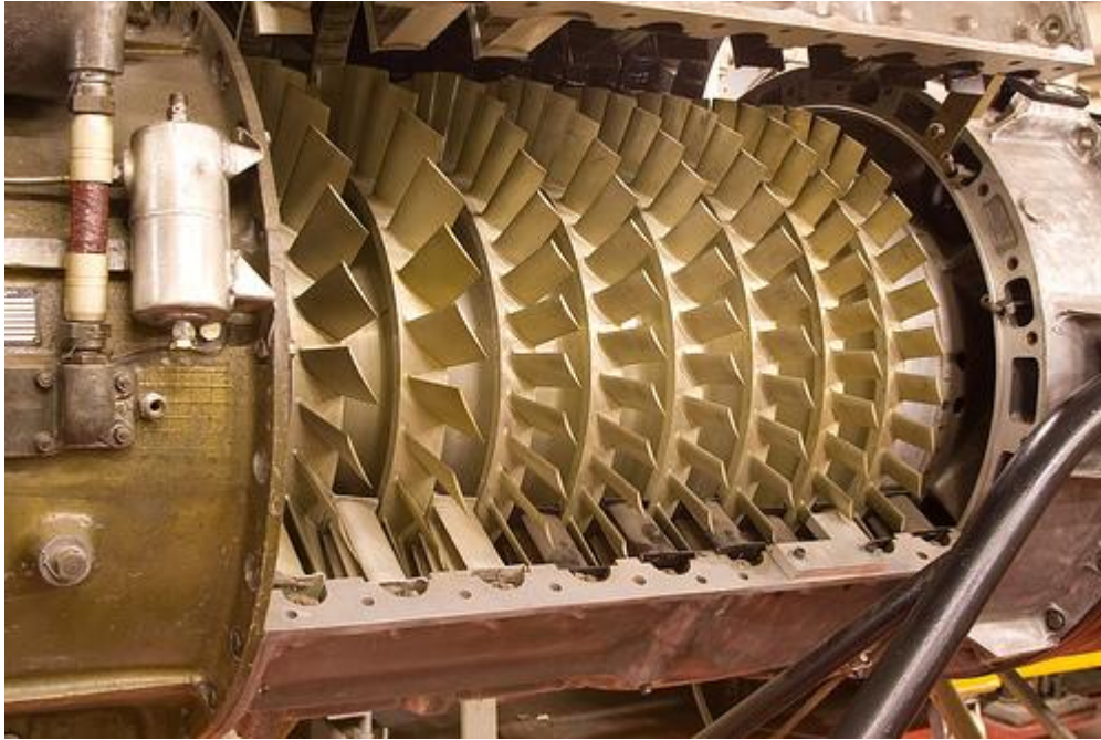
Figure 1.1.2: Multistage Axial Compressor
