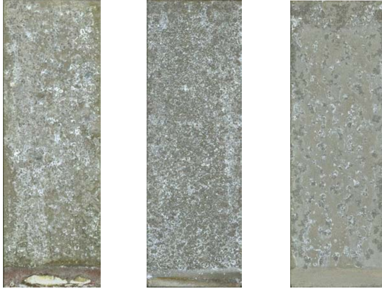
Figure 4.9: Sandblasted, unoxidized 2024-Al samples after salt spray testing. Left to right: Uncoated, (PAH / PAA), (PEI / Ultem)
