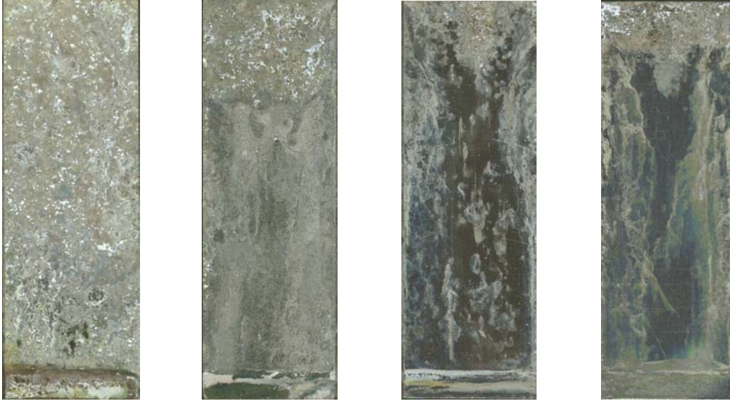
Figure 4.8: 2024-Al samples cleaned only with methanol after salt spray testing.
