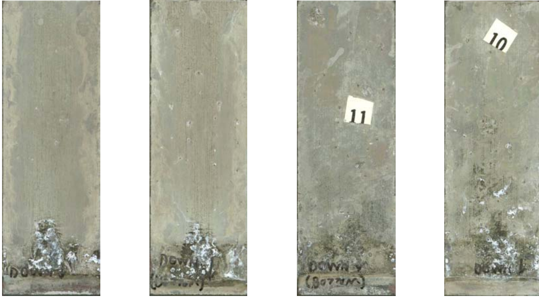
Figure 4.13: Front and back of acid etched, oxidized 2024-Al samples after salt spray testing. (PEI / Ultem / Lap) samples
