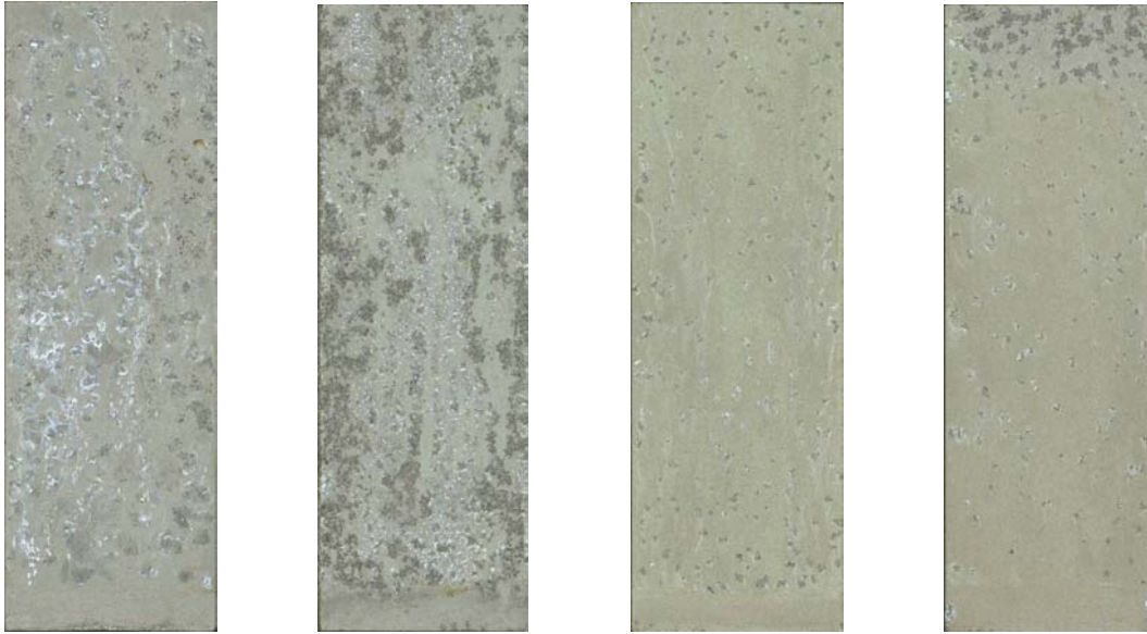
Figure 4.10: Sandblasted, oxidized 2024-Al samples after salt spray testing. Left to right: Uncoated, (PAH / PAA), (PEI / Ultem), (PEI / Ultem / Lap)
