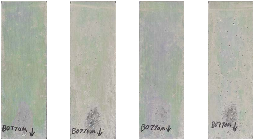
Figure 4.12: Front and back of acid etched, oxidized 2024-Al samples after salt spray testing. (PEI / Ultem) samples
