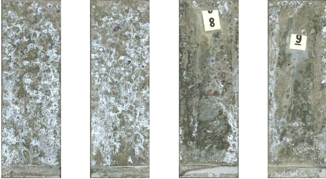
Figure 4.11: Front and back of acid etched, oxidized 2024-Al samples after salt spray testing. Uncoated samples
