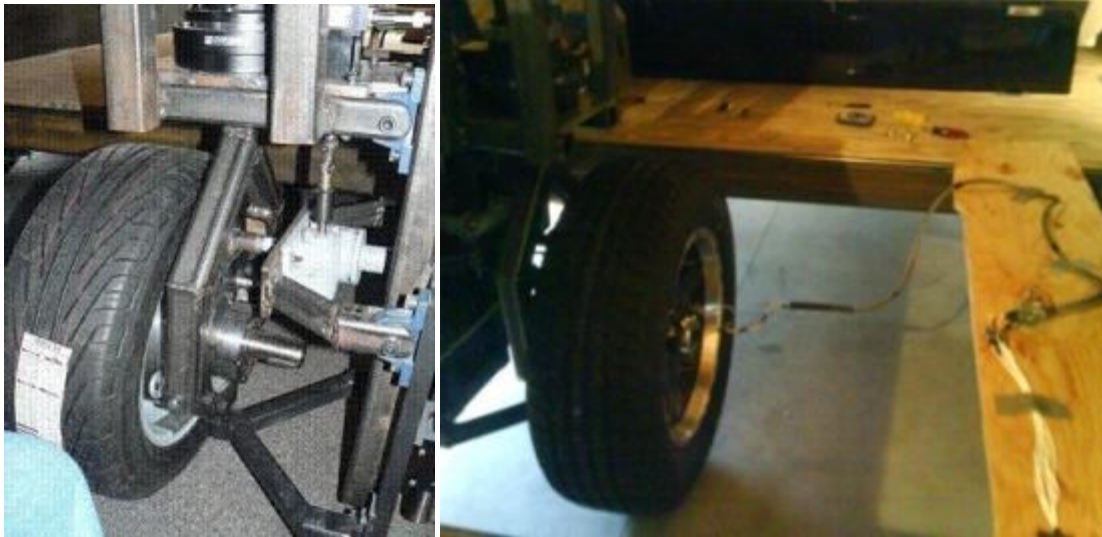
(a) (b) Figure 4.2. (a) Tire test rig and (b) its placement in the trailer
