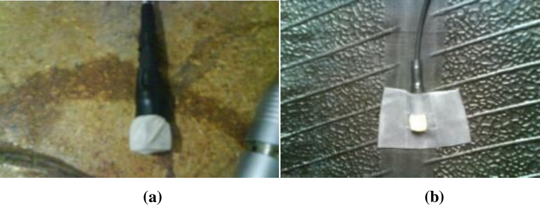
Figure 3.1. Accelerometer (a) enclosed in latex and (b) glued to the inner liner
